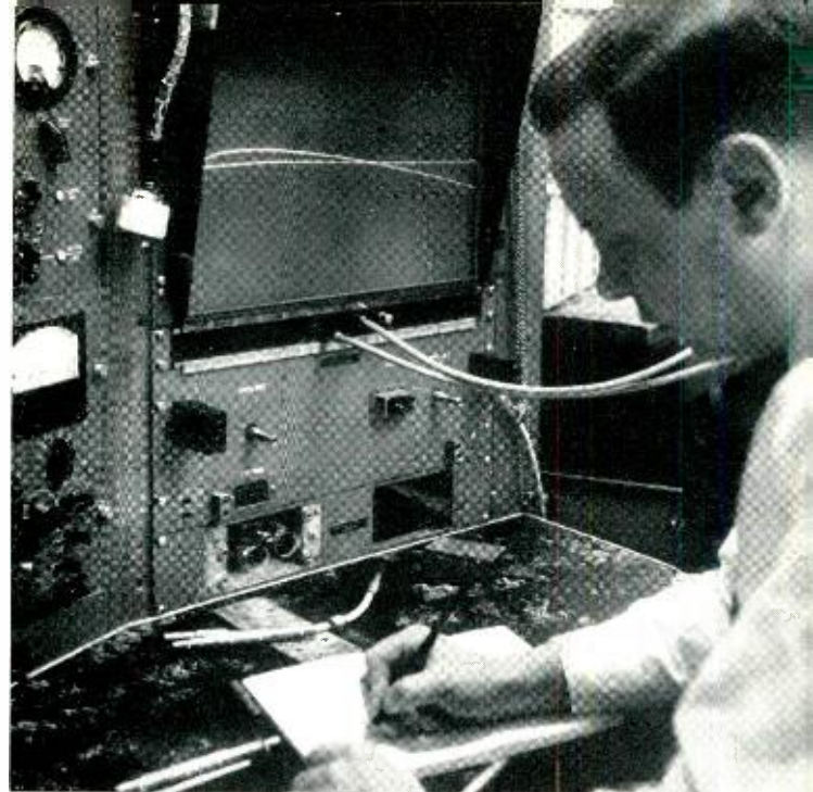
Fig. 4—J. J. Jansen measuring gain characteristics of an L3 amplifier in Bell Telephone Laboratories.
