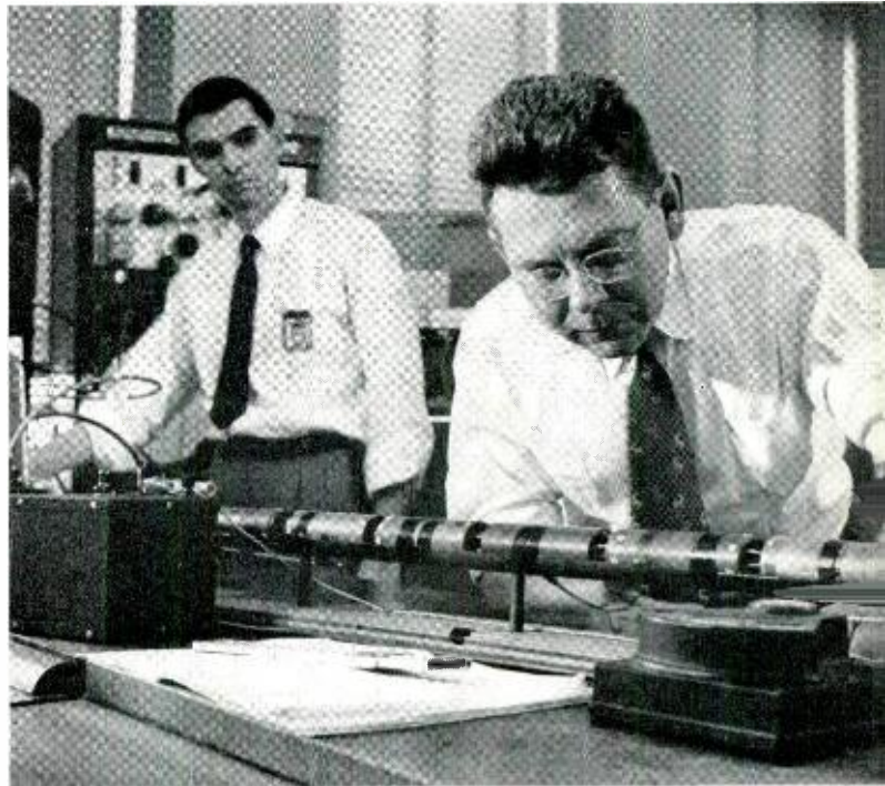
W. Klute, right, and Gilbert O'Connor perform equalization tests on a model of a submarine cable repeater. The units of the repeater are assembled as they would be in an actual repeater.
