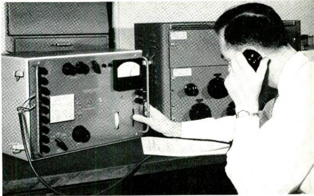
Fig. 3—R. A. Patterson makes a test of an interfering frequency. The receiver gives aural recognition of the interference.
