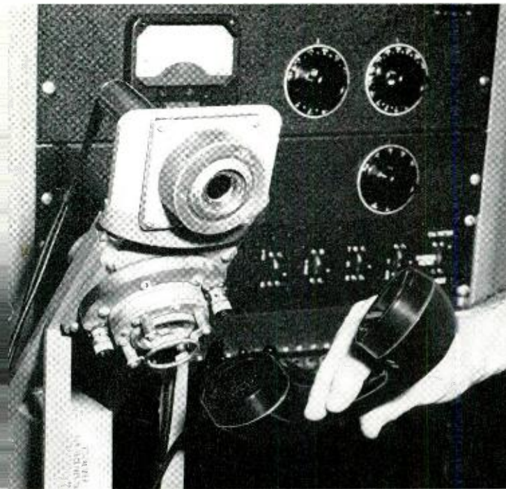
Fig. 4—Western Electric 640AA microphone (in upper fixture) and “artificial mouth” being used in device for testing telephone handsets.
