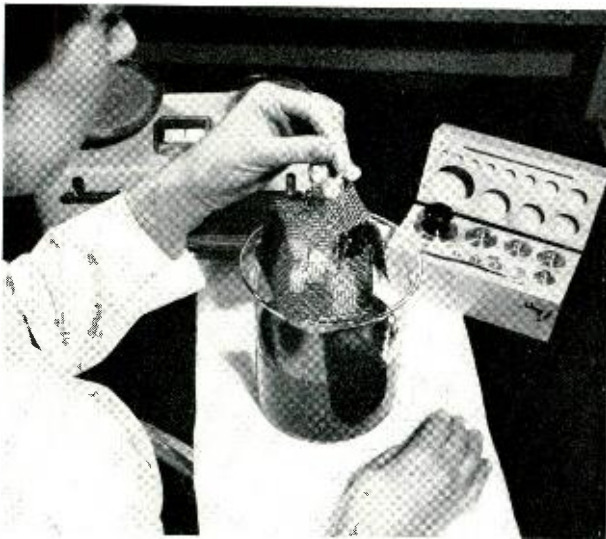
Fig. 4—Wood blocks being dipped in pentachlorophenol-petroleum solution to determine effect of mold on penetration of preservative.
