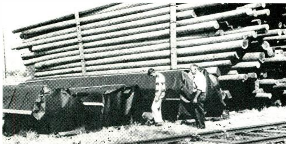
Fig. 2 — Douglas fir field experiment, Oregon, in 1952. L. R. Snoke, left, inspects tar paper covers on group of poles.
