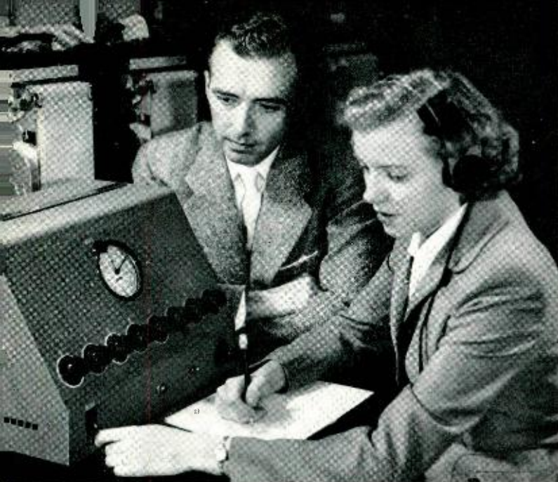
Fig. 1 — Mrs. Marilyn Cusick, of the New York Telephone Company, operates the Laboratories' dial tone speed measuring set while W. G. Barrett looks on.
