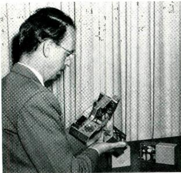
Fig. 2—The author plugs a channel filter into a carrier-frequency subassembly of a channel unit.
