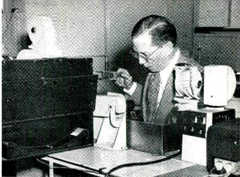
The author adjusts the external mirrors of the high-speed recorder to properly align the reflected beams on the film.
