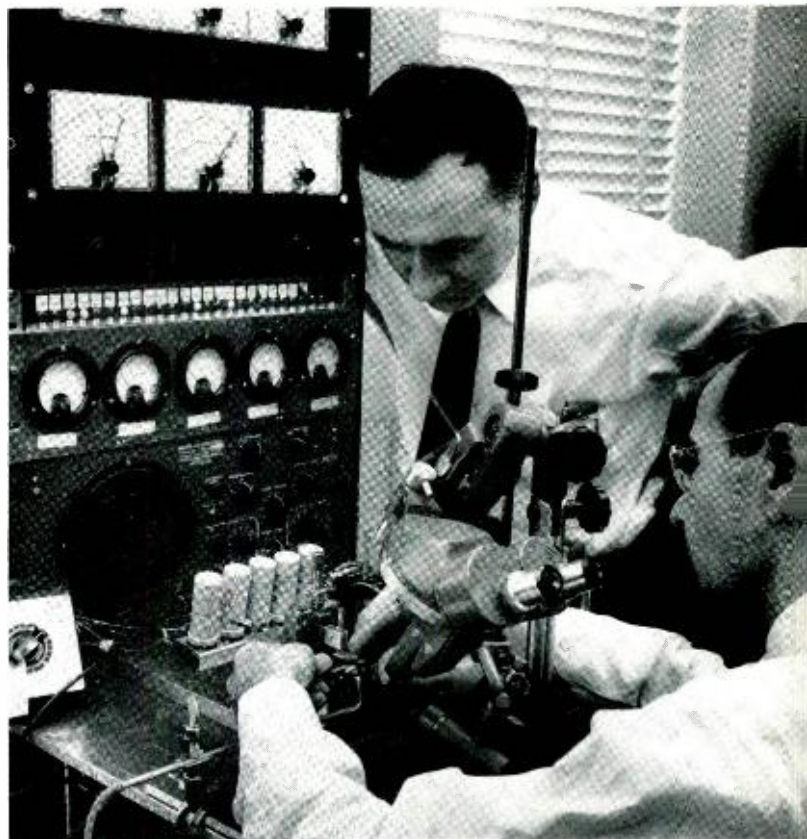
Fig. 5—The experimental automatic bonding machine: L. G. Schirapj (left) and E. Dickten are loading machine with a "header," in which is mounted the junction bar.
