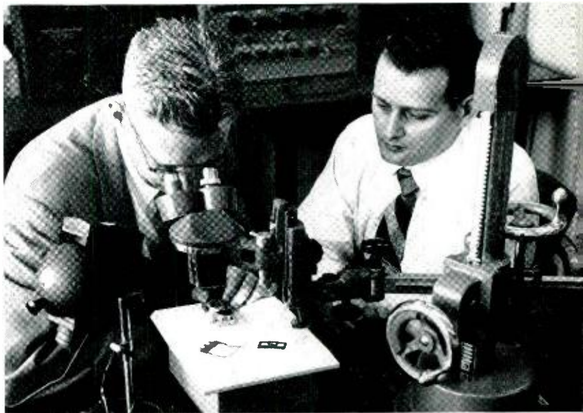
Fig. 2 — The author examines the surface of a wire-spring relay armature for wear, assisted by M. Feder.
