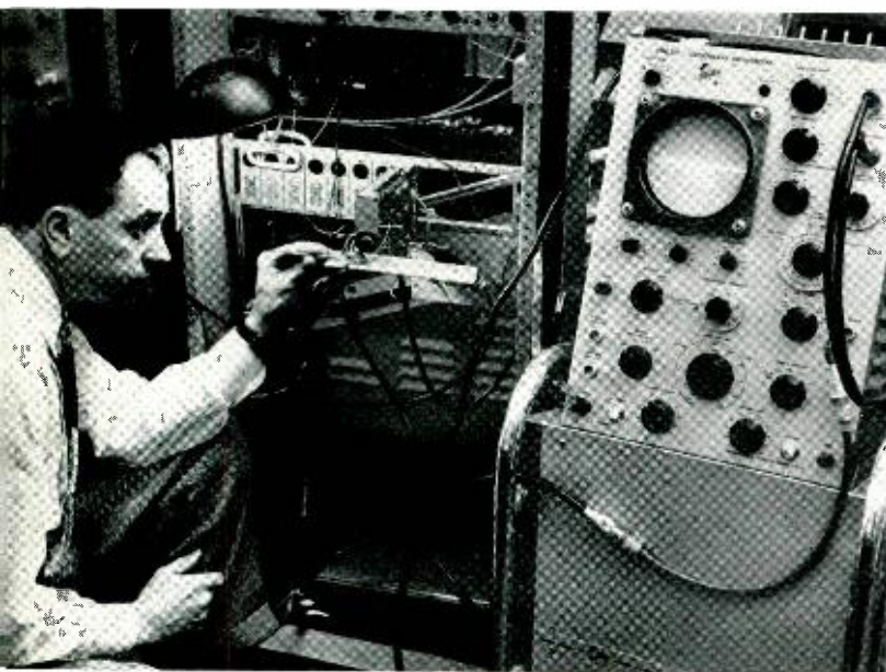
Fig. 1—R. L. Carbrey adjusting transformer in junction tetrode pulse generator. The oscilloscope at the left displays 0.050 microsecond pulses.
