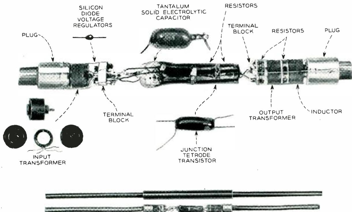
Fig. 1—An enlarged view of the amplifier unit with components is shown at the top. Actual size views of the amplifier, with and without cover, are shown below. The unit is shown inserted between lengths of experimental 0.1 inch coaxial cable.
