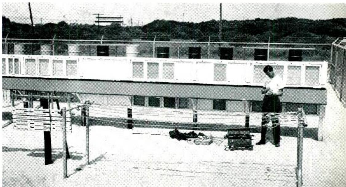
to determine the extent of deterioration, if any, including such factors as damage from corrosion and insect attack. Four of the eighteen exposure test locations were chosen chiefly for their soil conditions, these being acid, alkali, clay, and salt marsh. Three other areas are in large industrial cities so it is possible to observe how the plant reacts to industrial gases and fumes. Other plots were chosen for their insect-infested, humid, or corrosive conditions.
