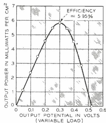
Fig. 6— Solar cell power output for various external loads, at an operating temperature under full sunlight of 25°C.
