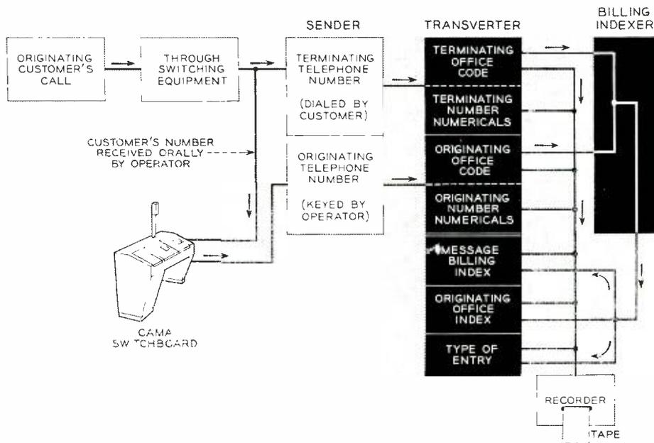
Fig. 1—Diagram showing flow of information through the transverter and billing indexer.
