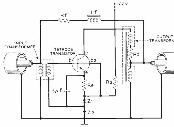
Fig. 5 — The amplifier electrical circuit.
