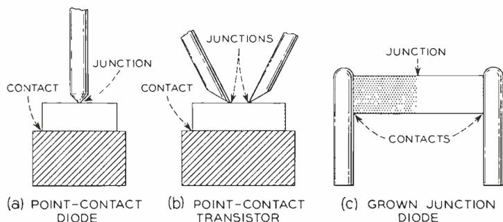
Fig. 3 — Three uses of fast recombination contacts.
