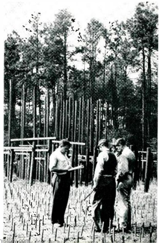
*Fig. 7 — A. Mendizza examining samples of strand, lashing wire, and cable sheathing for indications of corrosion at the exposure test plot at Kure Beach, North Carolina. Plot is close to the ocean so that materials are subjected to salt water spray.*
