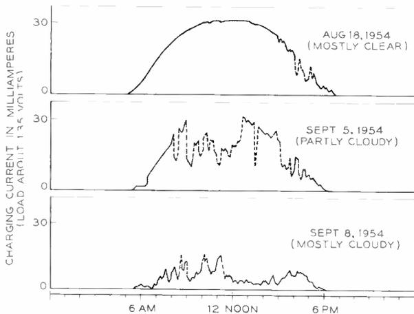
Fig. 7 — Storage battery charging current on clear, partly cloudy, and mostly cloudy days.
