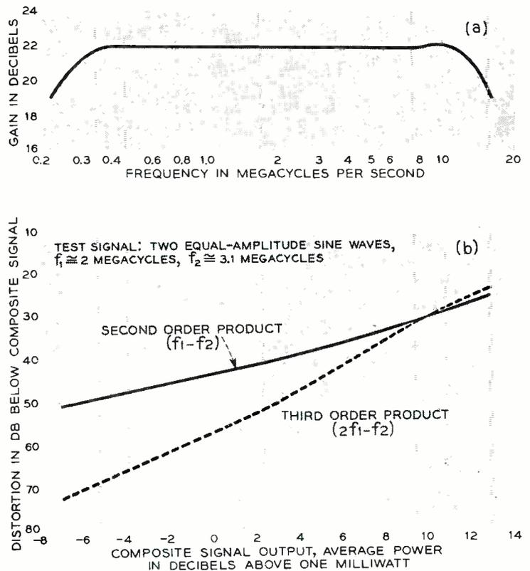
Fig. 2 — (a) Amplifier gain-versus-frequency, and (b) intermodulation distortion characteristics.
