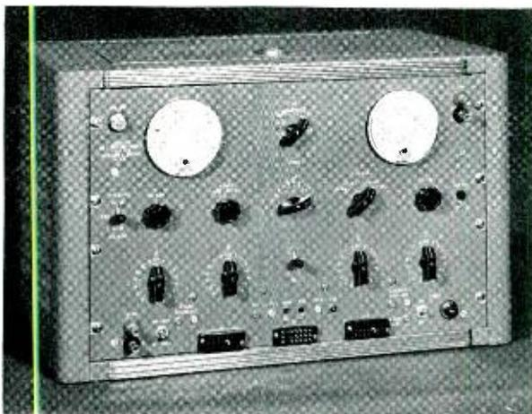
ample, it puts the correct termination on the vacuum-tube voltmeter and sets up the different signaling test conditions. Switches C and D, in like manner, can set up about 60 different test conditions for group, repeater, oscillator, and filter units.
