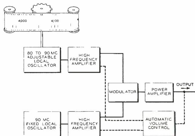
Fig. 2—Principal components of broadband test oscillator.
