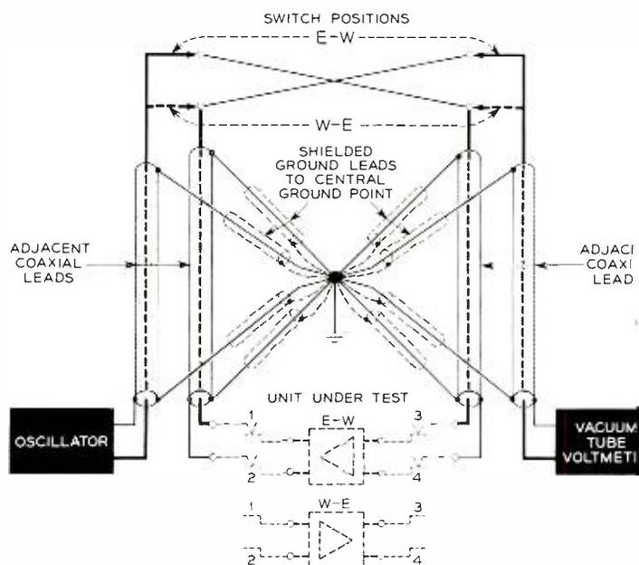
Fig. 4 — Final arrangement of coaxial cables and shielded ground leads in the test set.
