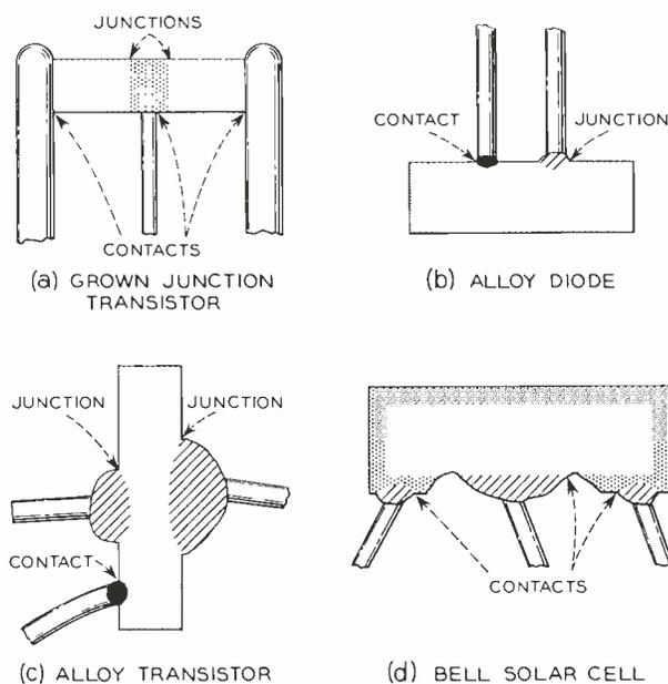
Fig. 4 — Four uses of non-injecting contacts.
