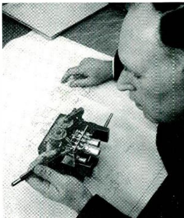
*Fig. 3 — K. F. Rodgers, who did the mechanical design of the local oscillators, checks the wiring on an experimental unit.*
