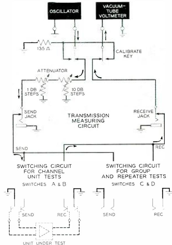
Fig. 2—The test set arranged for transmission tests.
