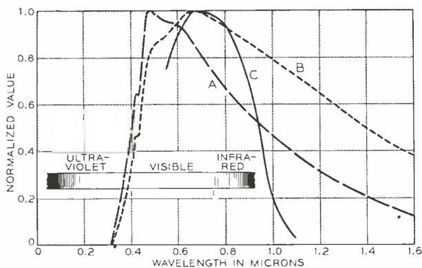
Fig. 4— (A) solar energy distribution, (B) photon distribution and (C) short-circuit response curve for a silicon solar cell.
