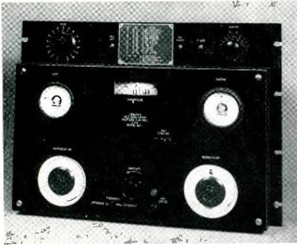
Fig. 1—Panel view of 56A Oscillator showing arrangement of meters and operating controls.
