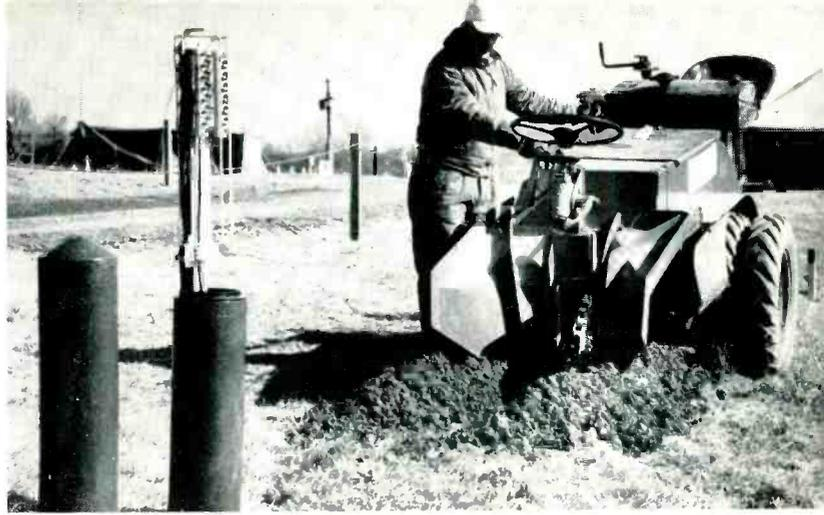
*Left — Conference members observed front-mounted hydraulic pole-hole digger in operation. Right — Cable terminals and cable terminal housings (left), and trenchers for burying distribution cable (right) were exhibited at Chester. Operator is T. W. Rolph of the Laboratories.*
