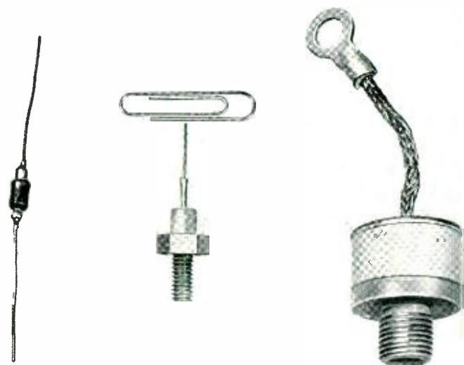
Fig. 3— Developmental silicon rectifiers. Left, 0 to 1 ampere; center, 1 to 10 amperes; and right 10-100 amperes.
