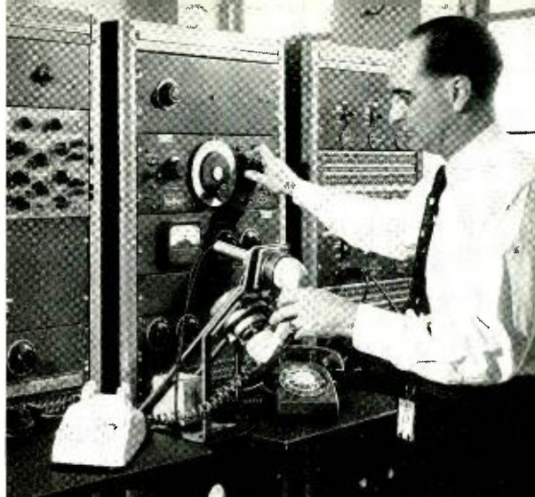
Fig. 1 — E. C. McDermott testing the transmission characteristics of the 500-type color set.
