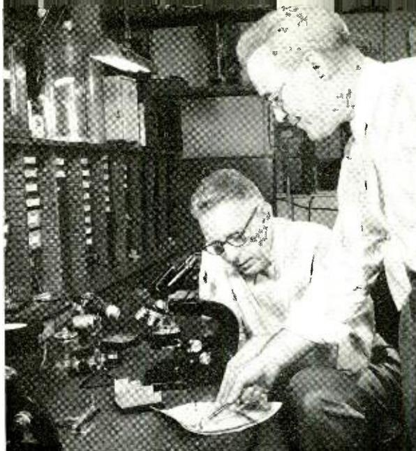
Contact contamination is a continual problem to the Bell System, and only thorough study of the various contaminants can lead to possible methods for eliminating their effects. Because of the small size of relay contacts and the difficulty of isolating microscopic contaminants without interrupting telephone service, a new technique was needed. This technique utilizes plastic replicas of the actual contact surfaces, effectively providing “fingerprints” of troublesome relays.
