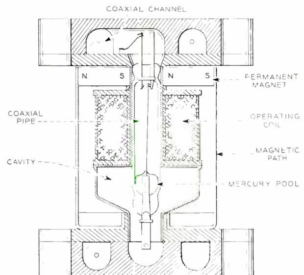
*Fig. 3 — Transverse section through one element of a 223-type coaxial switch.*
