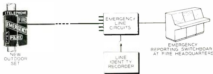
Fig. 1 — The direct-line telephone reporting system.
