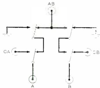
*Fig. 2 (above) — Simplified schematic of the signal circuit of the 223-type coaxial switch.*
