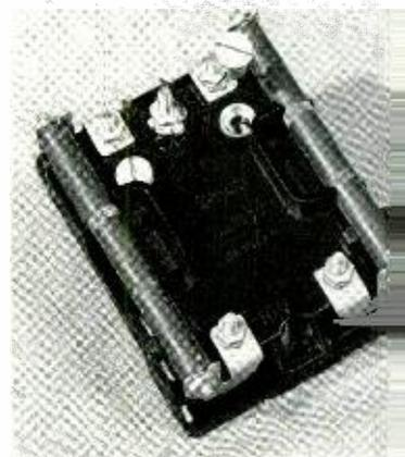
of the arrester. This fuse interrupts power contact current if that current is large enough, and persists long enough, to overheat the protector and possibly start a fire.
