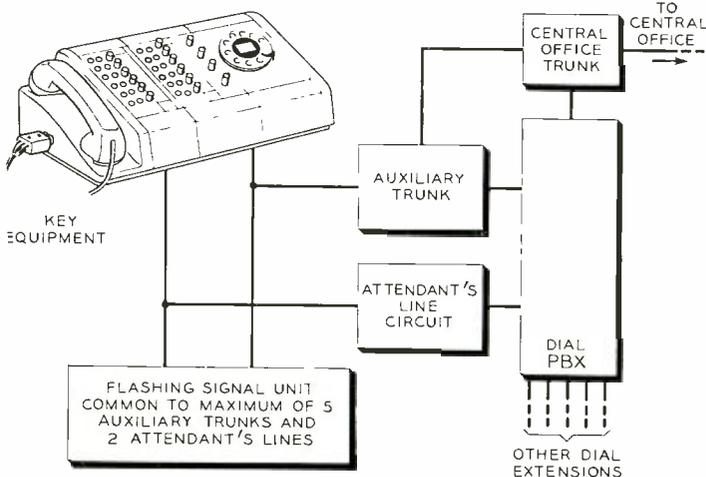
ig. 3 — How key equipment is used with a dial PBX.
