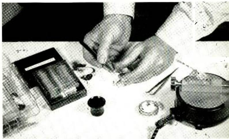
*Fig. 5 — The replica is returned to the slide immediately after it is made to reduce hazard of contamination.*
