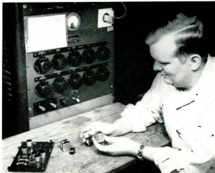
Fig. 2 — F. J. Sweeney compares the new transformer with its predecessor used in N1 carrier. Five of the new transformers can be seen on a PI-carrier printed-wire board.
