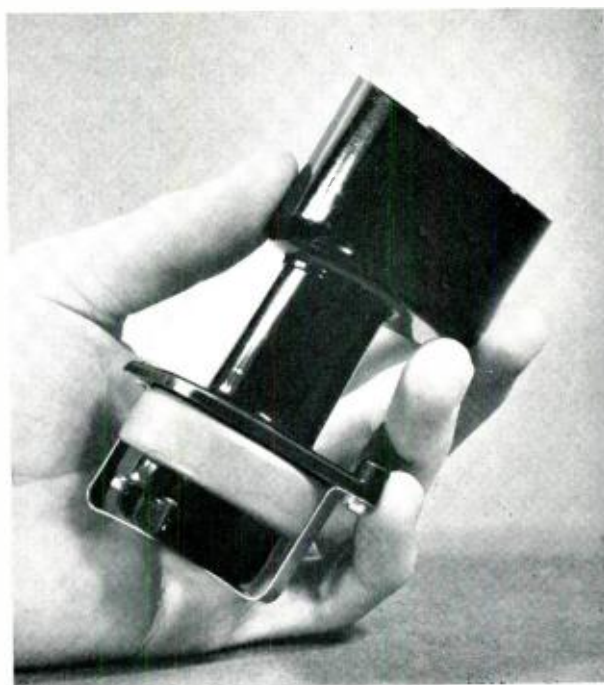
Fig. 2 — The sounder of the tone-ringer circuit — receiver is shown in palm of hand and double tube resonator appears above.
