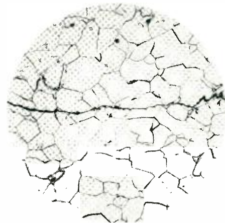
Fig. 2—Nonductile transcrystalline fracture is characteristic of metal failures due to fatigue.
