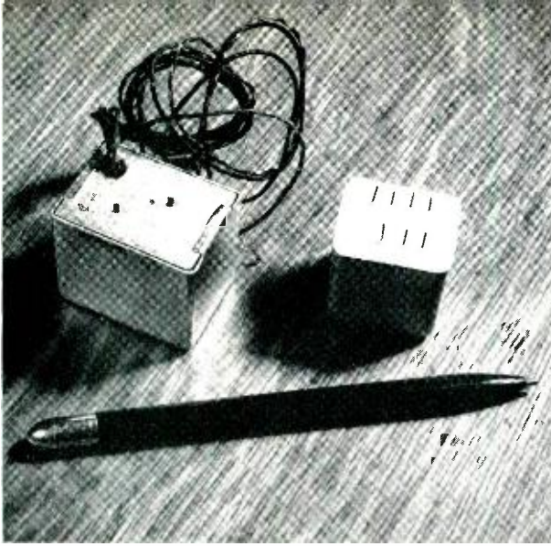
Fig. 3 — N carrier audio transformer, left, and new P carrier transformer, side-by-side, show comparison in size and construction details.
