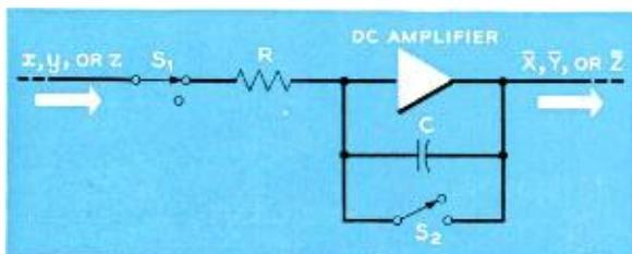
*The basic circuit for the bias outputs of the TDE. These outputs are obtained by using three dc amplifier-integrator circuits. The computed value is read out at the end of the evaluation interval.*
