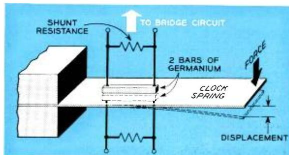
*Displacement gauge constructed with crystals of germanium. Such gauges are up to two orders of magnitude more sensitive than common types.*
