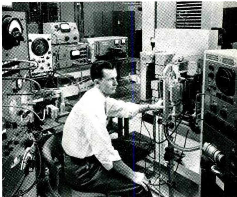
R. Kuntze running a test on equipment for the new TH microwave (6000 megacycles) system.
