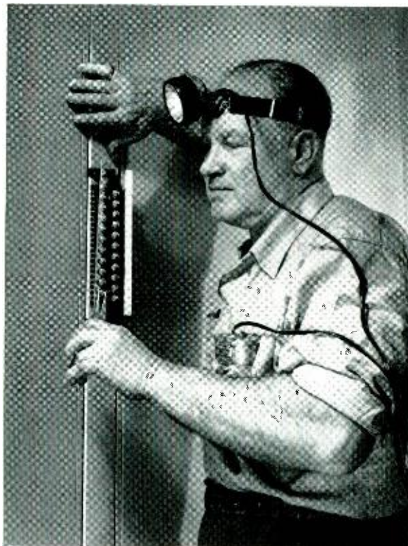
The Head Lamp is an important source of light when both hands must remain free. A diffusing lens creates a broad beam of light for close work.
