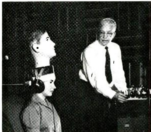
R. L. Hanson, right, sends electronically altered sounds to Mary Lou Hartig's "extra" head. She then indicates the apparent direction of sounds.
