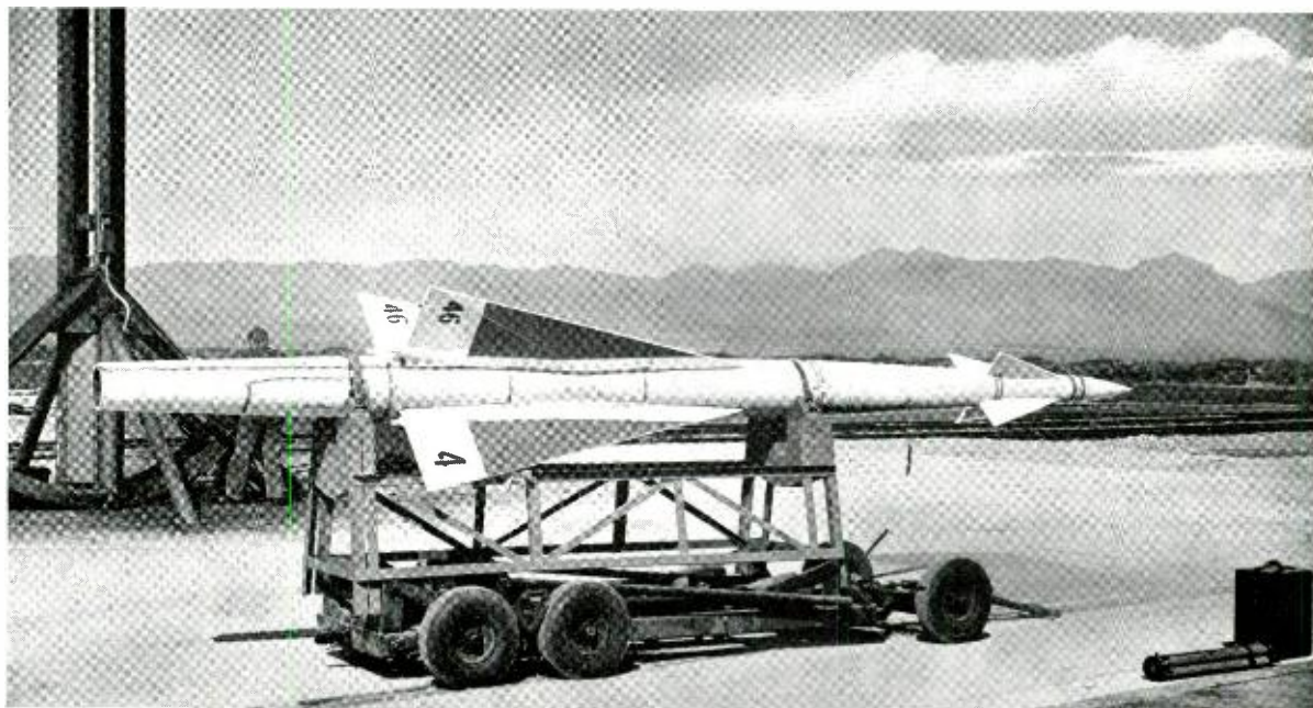
This is the 1946 model of the Nike missile, progenitor of the Nike family. With its solid-propellant booster and liquid-propellant sustainer,
