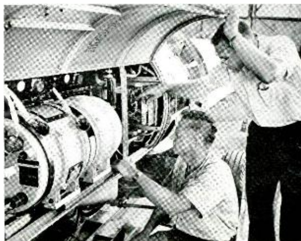
T. J. Greiser and D. R. Hagner examine second stage of the Air Force Thor-Able missile used to launch the NASA Tiros I weather satellite.
