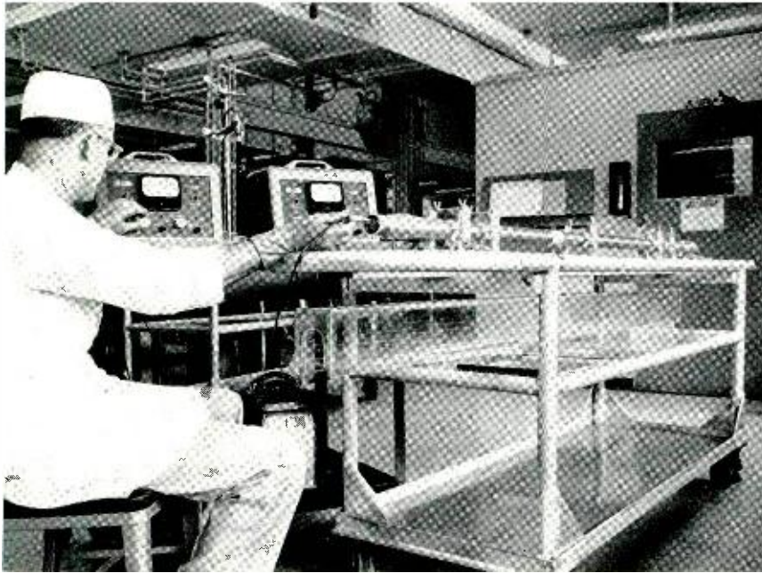
Technician examines glass seal with a Geiger counter to test its effectiveness.
