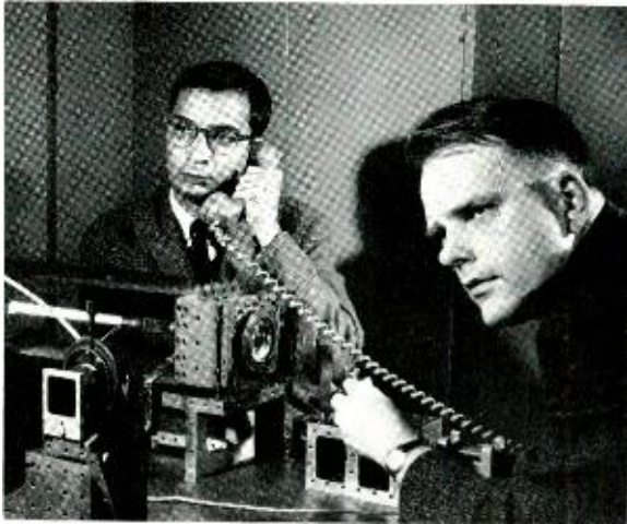
Infrared beam is voice modulated by Kerr Cell (left foreground). A. Javan prepares to talk over beam, while W. R. Bennett, Jr., adjusts optics.
