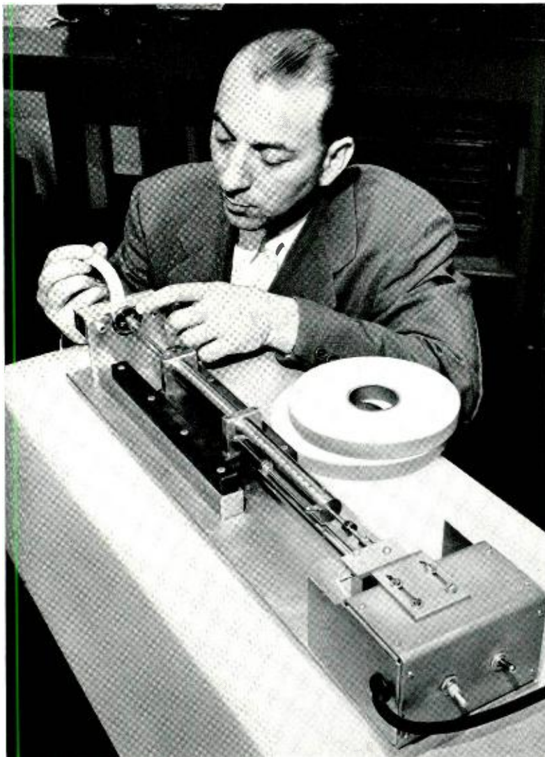
D. J. Nitti with instrument to measure paper tape punching pressure.
