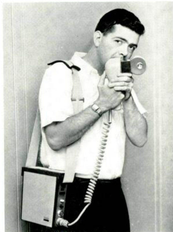
J. W. Ammons sights along portable maser housing. The power supply hangs from his shoulder.
