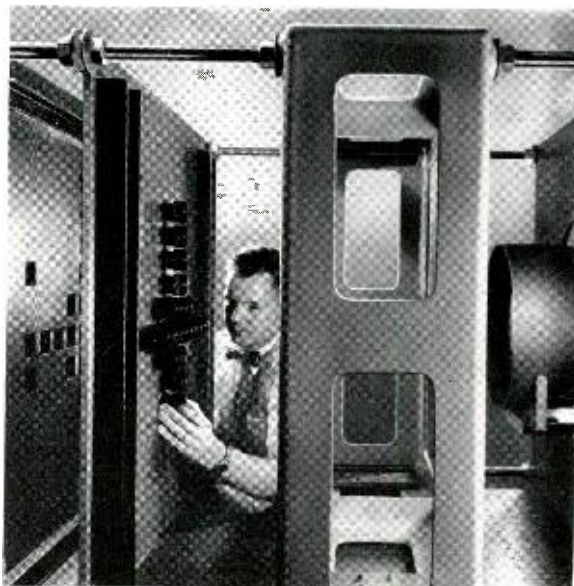
Lee H. Gallaher, Electronic Central Office Development Department, adjusts lenses on servo system of experimental flying spot store memory.
