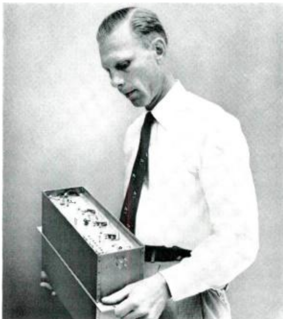
The author with low-pass filter package. This equipment passes the 312-to-2064 kc band and attenuates everything above it by at least 75 db.
