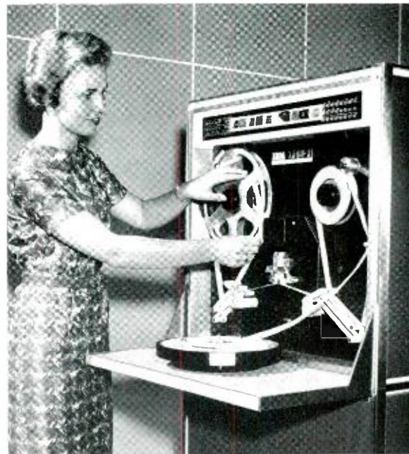
Mary O'Byrne, of Pennsylvania Bell, threads teletypewriter tape into reader, transmitting service order information to EDP equipment.
