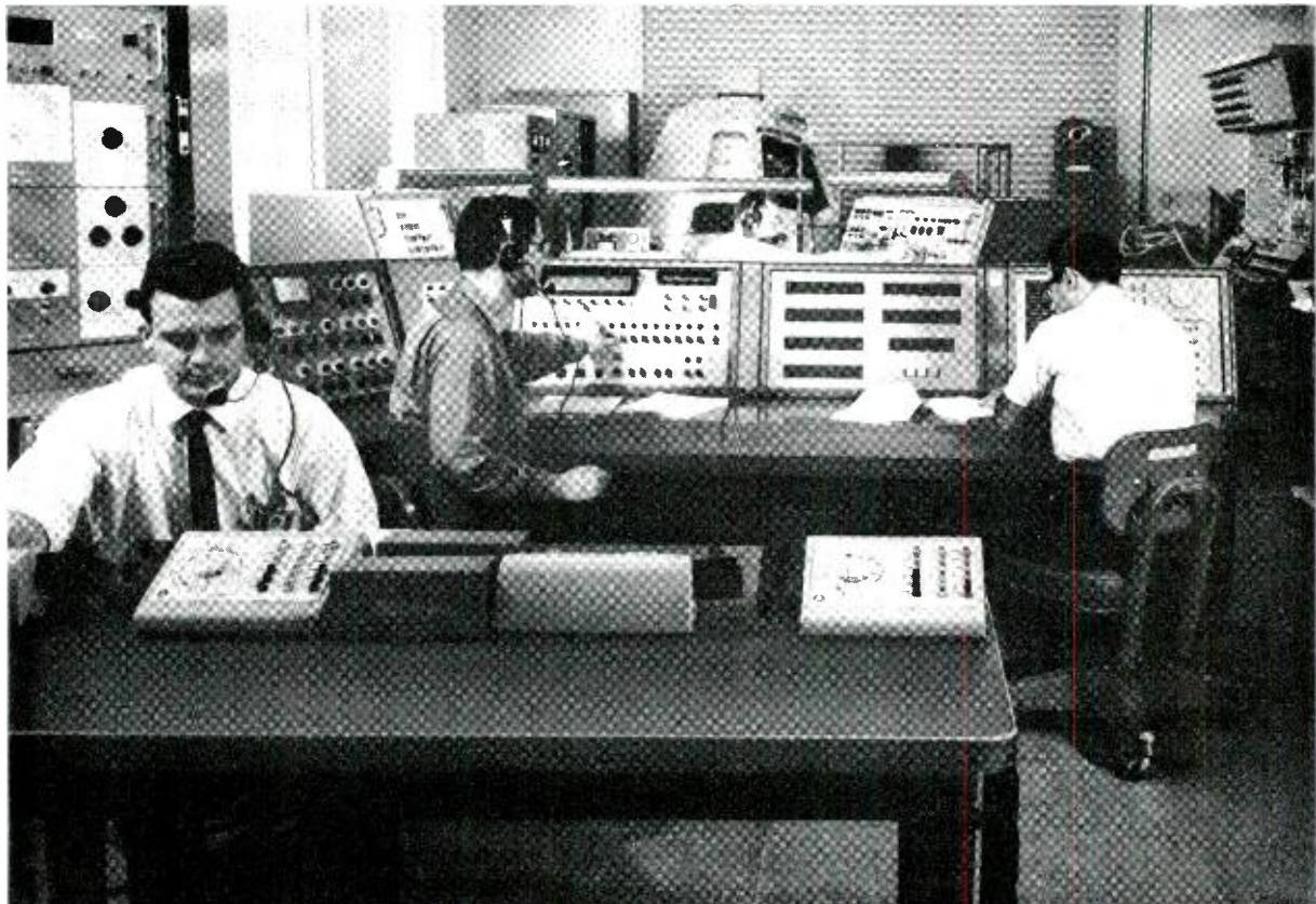
During simulation: two consoles (center) are the Telemetry and Command Subsystem and Chief
