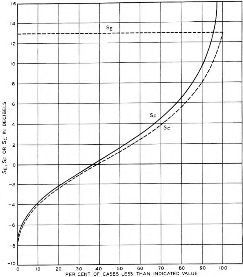
Fig. 7—Return loss distributions of cable pairs ( $S_F$ ), equipment ( $S_E$ ), and the combination ( $S_C$ ).
