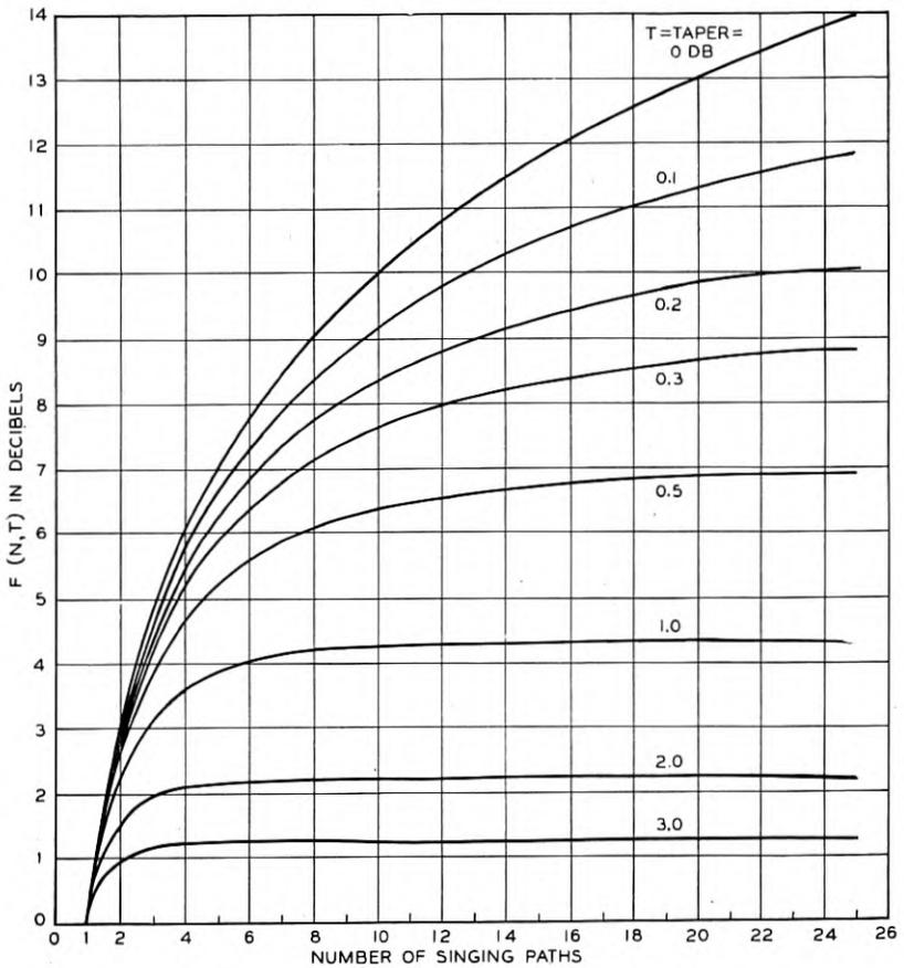
Fig. 3— $F(N, T)$  in perfectly regular circuit.
