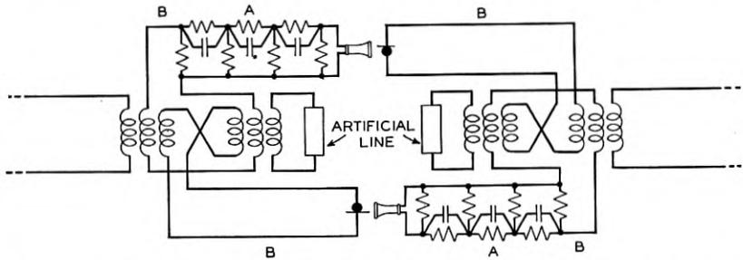
With this circuit the allowable unbalance is about double that with our present standard circuit. In addition to this, singing will not be introduced by any possible unbalance, however large, in either of the lines, provided the unbalance of the other line does not exceed a certain critical magnitude. Furthermore, the two lines connected together may differ radically in character since each is balanced separately against its own artificial line.
