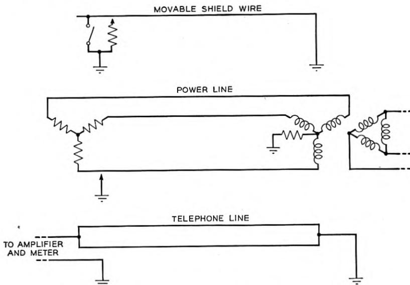
Fig. 5—Demonstration of shielding effect of grounded wire.
