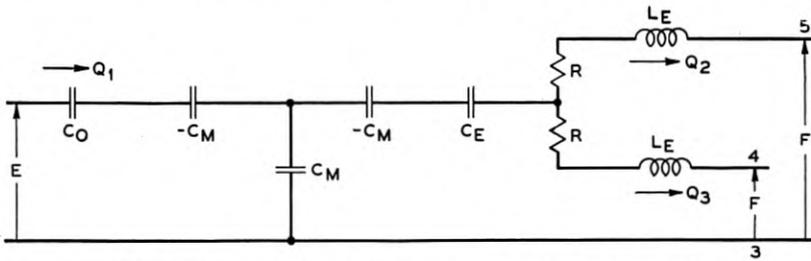
Fig. 2—Electromechanical representation of a symmetrical piezoelectric crystal.
