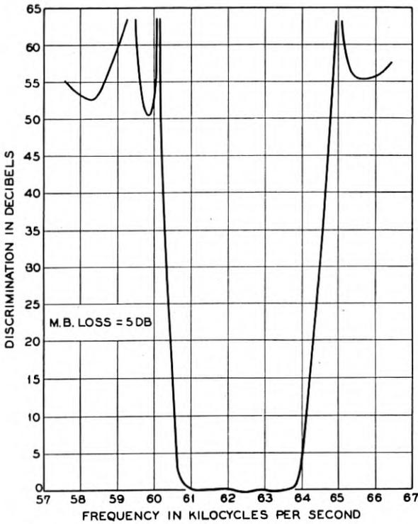
Fig. 7—Insertion loss characteristic of a single section band pass filter employing two crystals in each arm.
