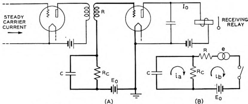
Fig. 25—Theory of level compensator. A. Simplified circuit.
