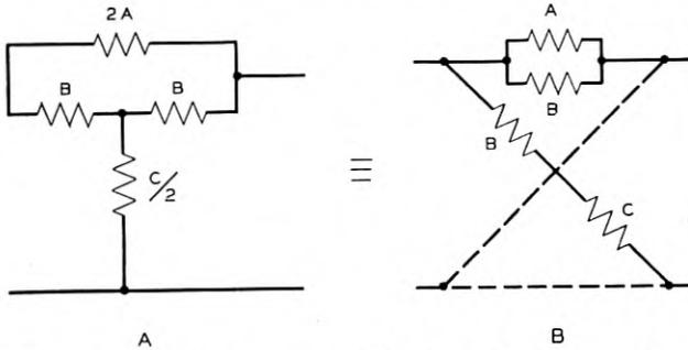
Fig. 10—Equivalence between bridge  $T$  and lattice networks.
