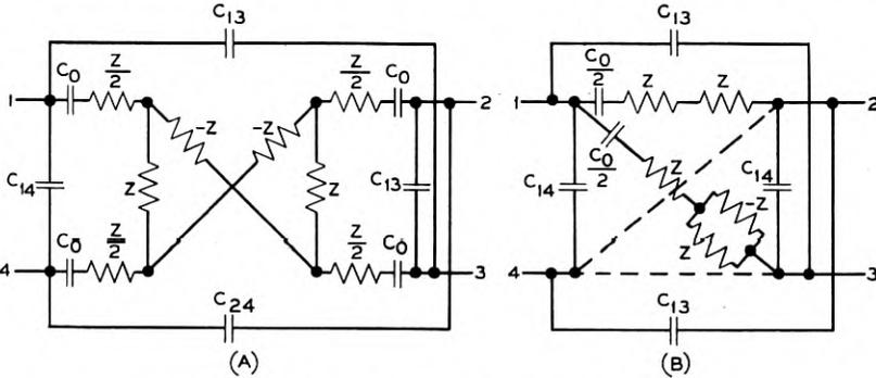
Fig. 17—Method for proving equivalence of Fig. 16A.
