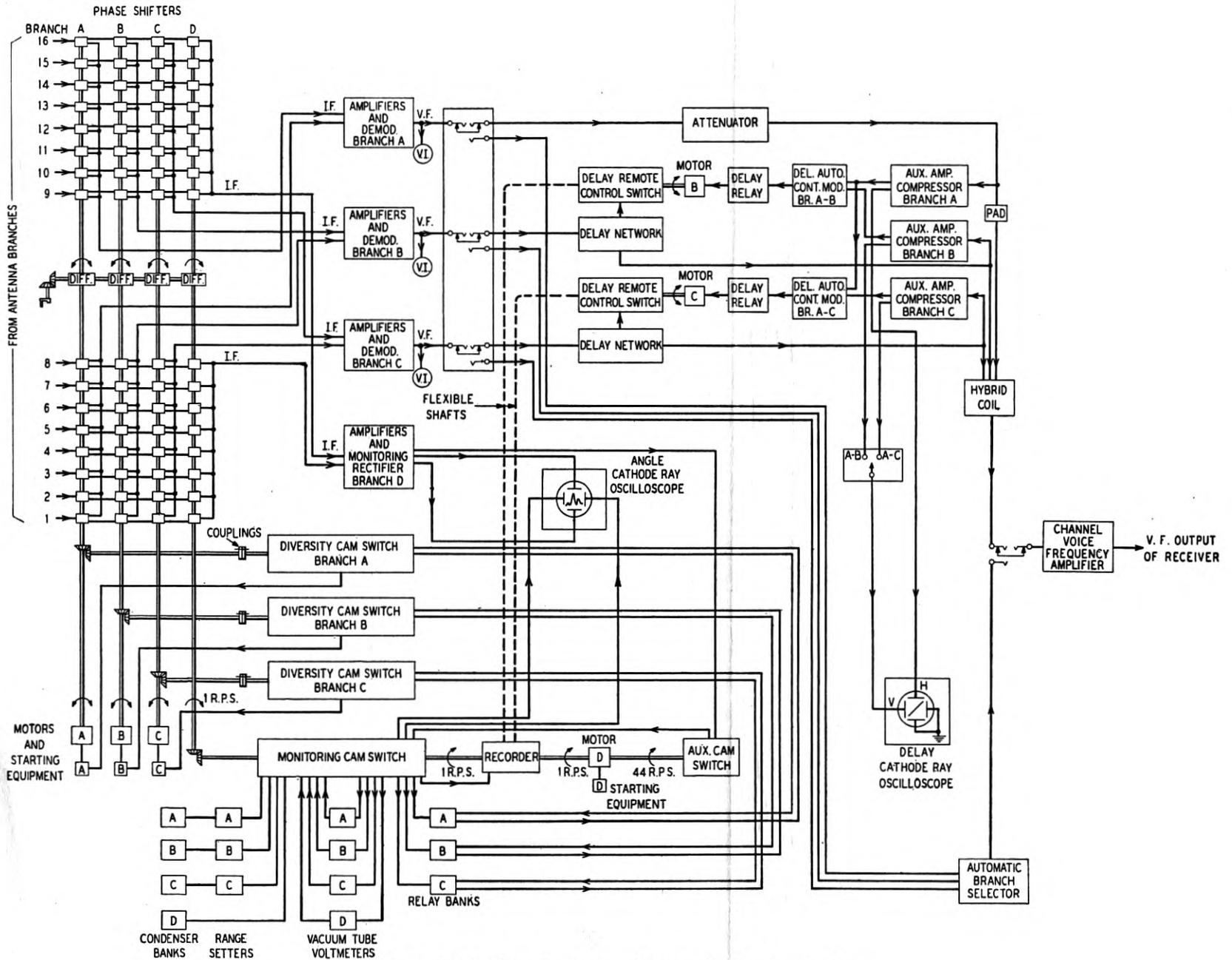
Fig. 8—Block schematic diagram of automatic adjusting circuits.
