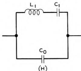
Fig. 14—Equivalent networks to represent transmission through divided plate crystal.
