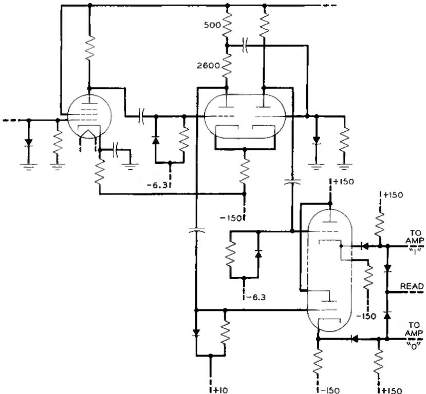
Fig. 17 — Readout circuit output signal generation.
