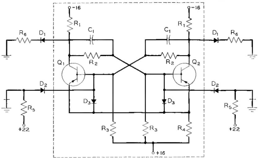
Fig. 15 — Flip-flop with simulated amplifier loads.
