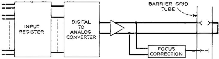
Fig. 3 — Deflection system functional diagram (one axis).
