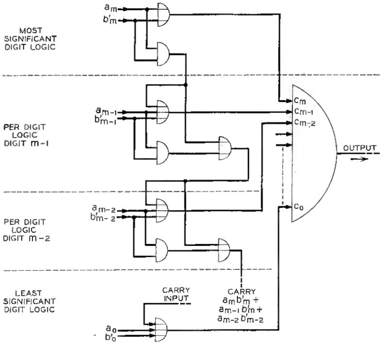
Fig. 5 — Sign-only comparator, binary-binary type.
