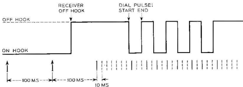
Fig. 9 — Two-rate scanning of calling lines.
