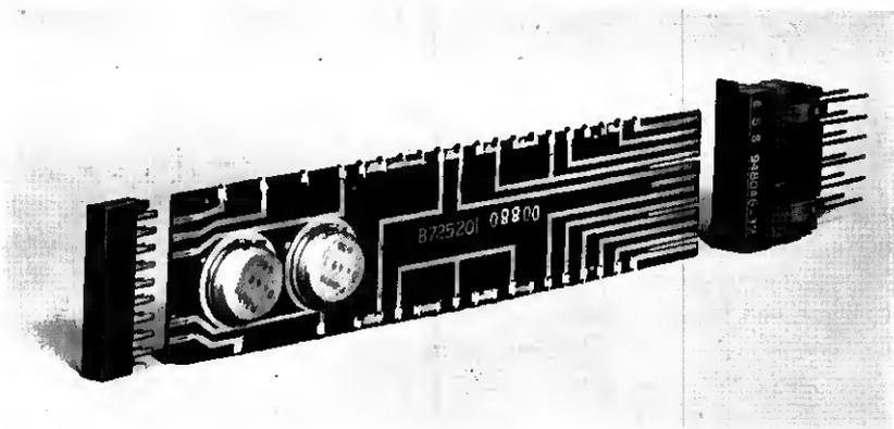
Fig. 22 — Printed board, shunting shoe and connector.
