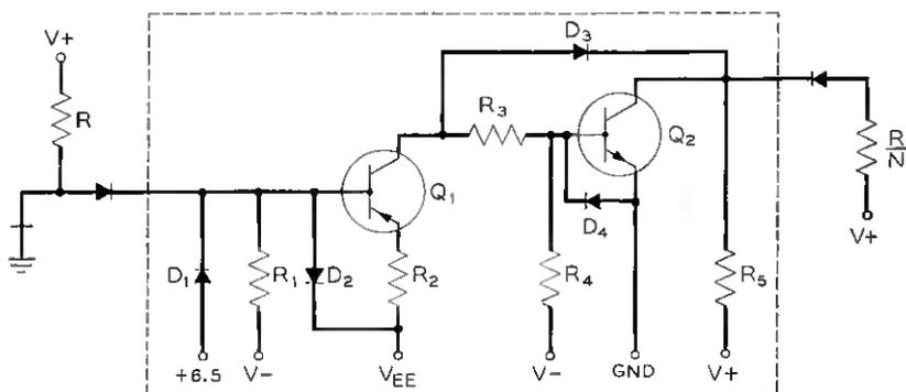
Fig. 13 — Nonsaturating amplifier.
