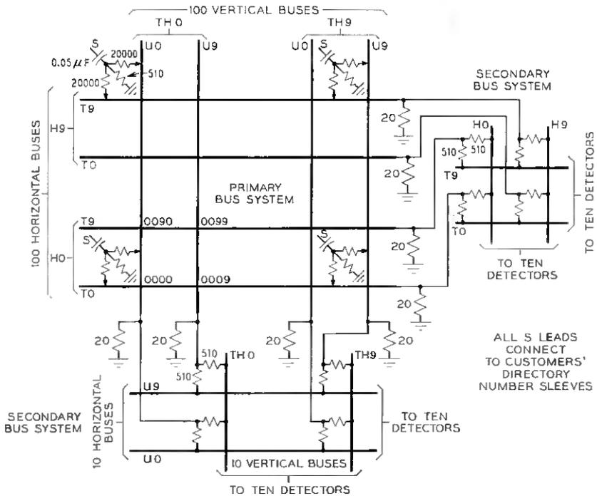
Fig. 2 — Number network and bus system.
