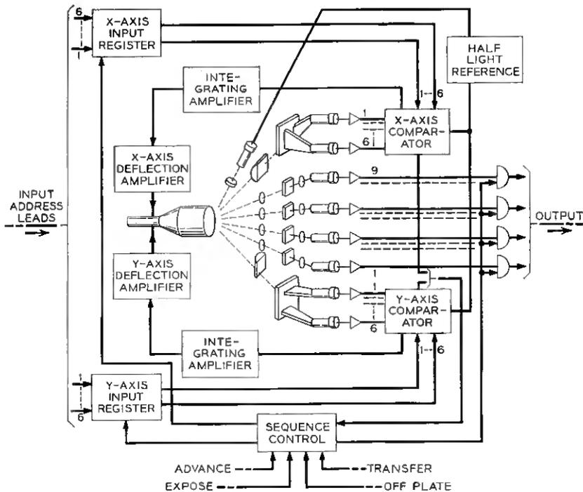
Fig. 7 — Block diagram of flying spot store.
