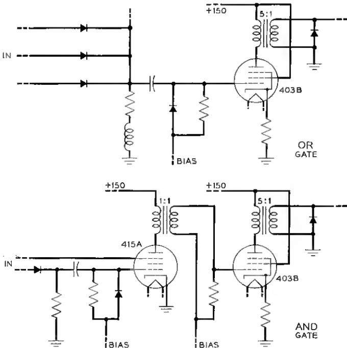
Fig. 10 — Logic circuit schematics.
