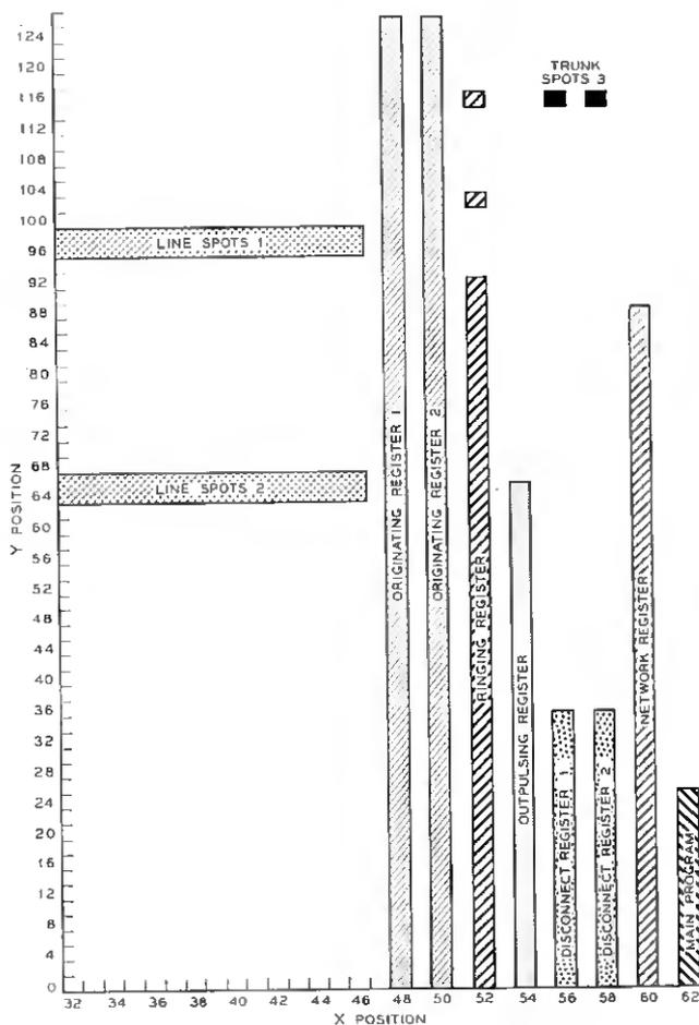
Fig. 12 — Barrier grid store spot layout.
