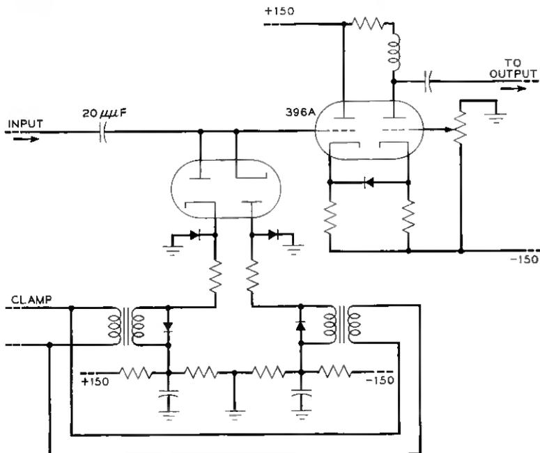
Fig. 16 — Readout circuit clamp and discriminator section.
