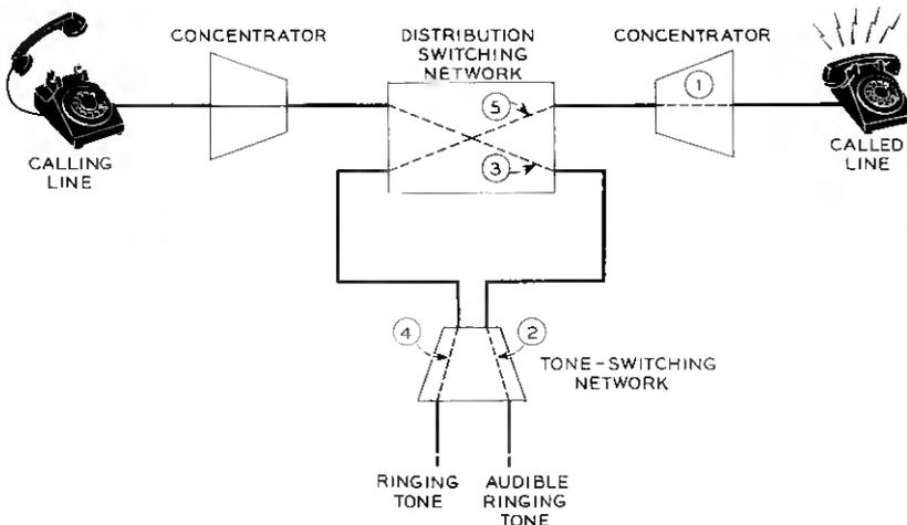
Fig. 17 — Ringing connections.
