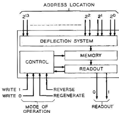
Fig. 1 — Barrier grid store system block diagram.
