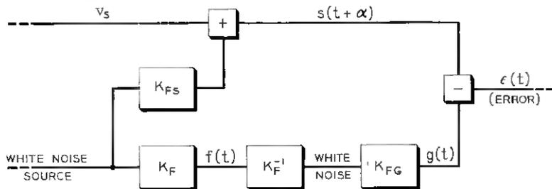
Fig. 15 — A physical model of a nonstationary system.
