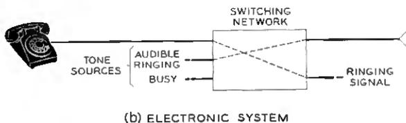
Fig. 6 — (a) Example of trunk circuit functions in electromechanical system; (b) example of use of switching network for signaling and supervisory functions.
