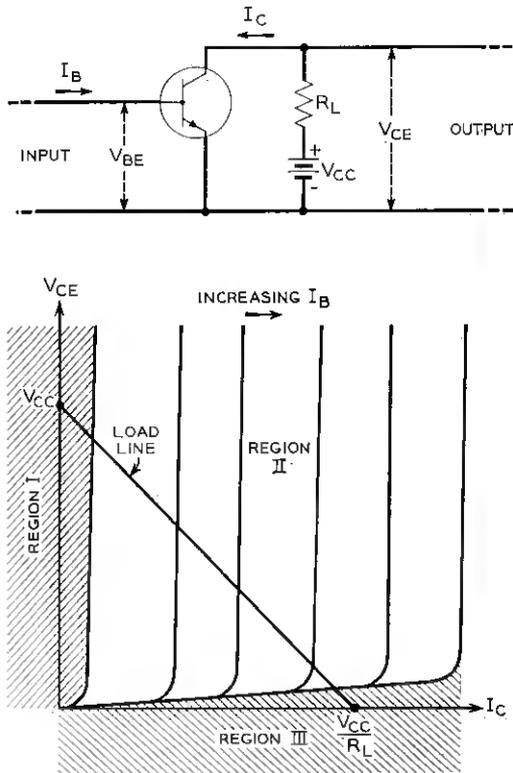
Fig. 7 — Transistor switch.
