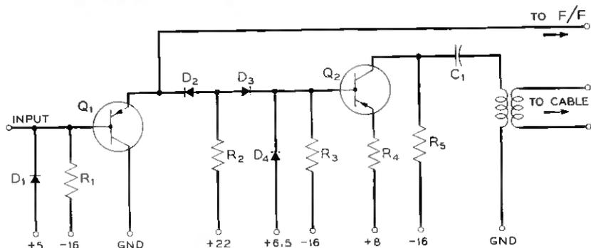
Fig. 19 — Cable pulser circuit.
