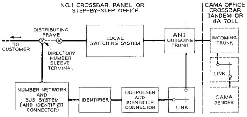
Fig. 1 — Block diagram of automatic number identification system.
