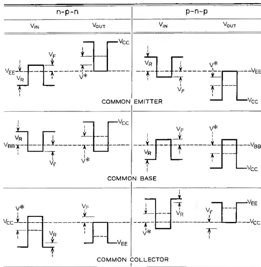
Fig. 8 — Input-output voltage relationships of various junction transistor configurations.
