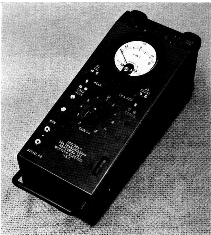
Fig. 40 — 54A transmission measuring set.
