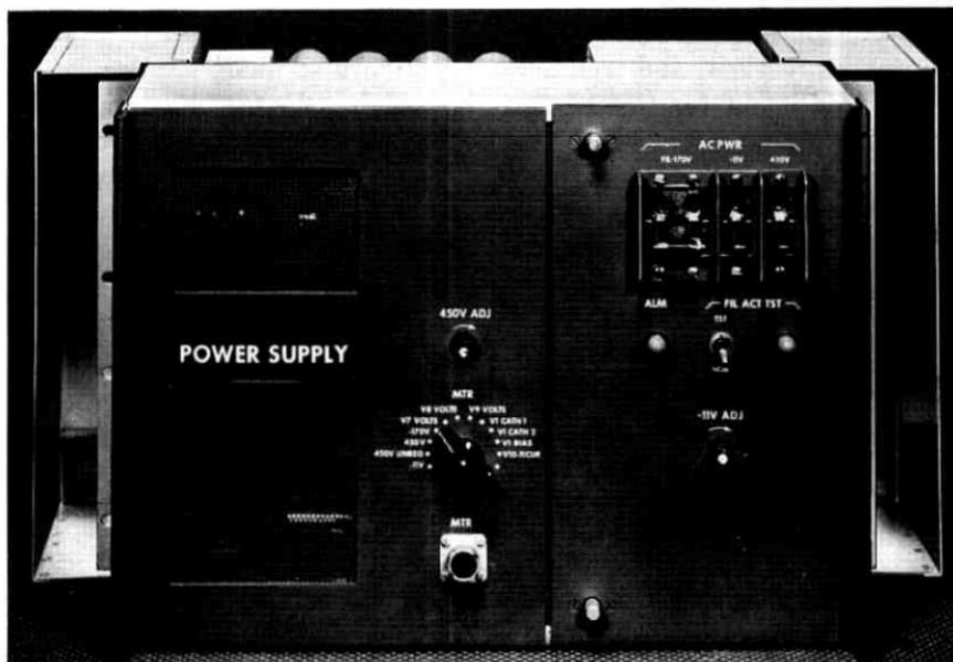
Fig. 11 — The klystron power supply.
