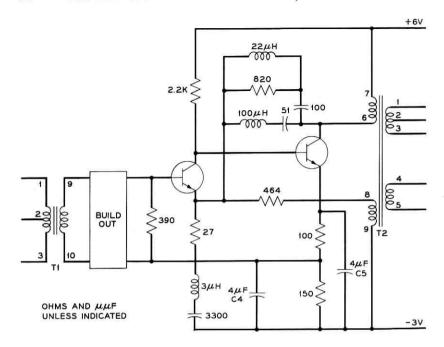
Fig. 14 - Repeater preamplifier circuit.
