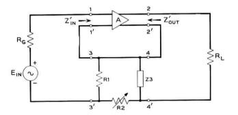
Fig. 2 - Equivalent circuit of a series feedback amplifier.
