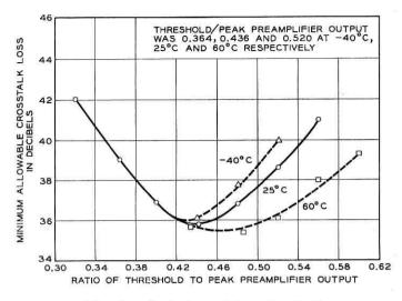
Fig. 61 — Typical crosstalk vs threshold.
