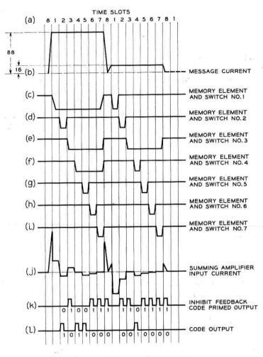
Fig. 20 — The encoding process.
