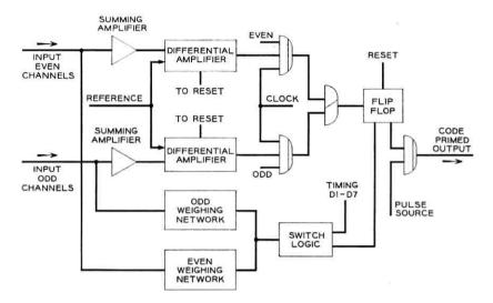
Fig. 21 - Dual encoder block diagram.
