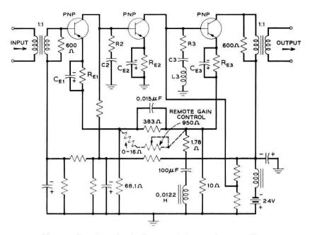
Fig. 5 - Complete circuit diagram of the transistor amplifier.
