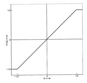
Fig. 15 — Limiting characteristic of system transmission in the absence of quantization.
