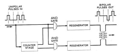
Fig. 11 — Bipolar converter.
