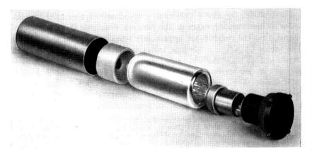
Fig. 16 — Temperature-controlled oven.
