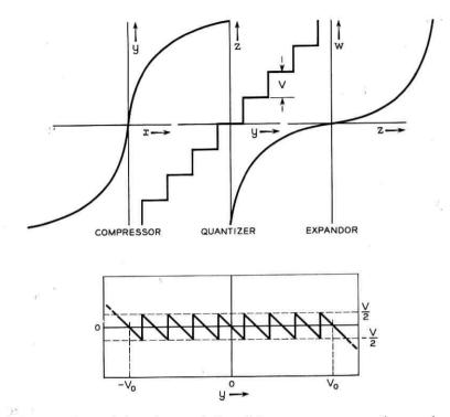
Fig. 7 — Transmission characteristics of the compressor, quantizer, and expandor. The quantizer transmission is decomposed into the sum of a linear term plus a periodic sawtooth function.
