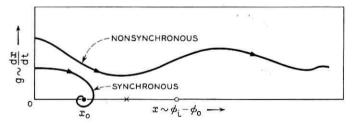
Fig. 2 — Phase plane representation of solution trajectories.
