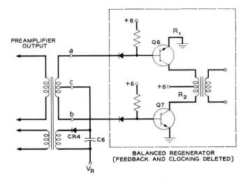
Fig. 22 - Conceptual threshold circuit.
