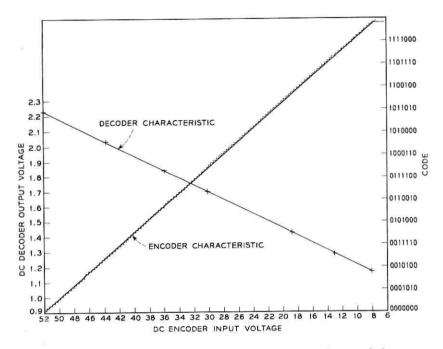
Fig. 28 — The encoding and decoding dc transfer characteristics.
