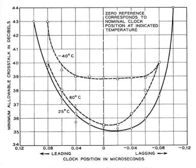
Fig. 60 — Typical crosstalk vs clock position.
