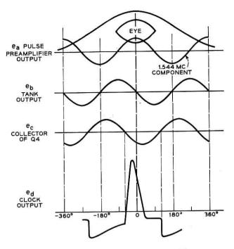
Fig. 33 — Clock phase at various points of Fig. 31.
