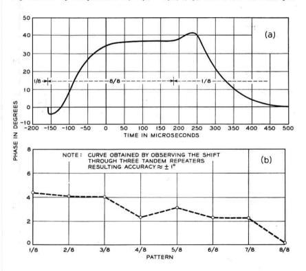
Fig. 58 — Measured clock pattern shift performance: (a) measured phase shift through eight repeaters due to abrupt change in pulse pattern; (b) measured phase shift per repeater due to change of pattern.
