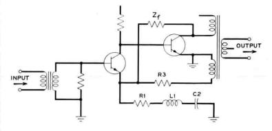
Fig. 10 - AC configuration of preamplifier.
