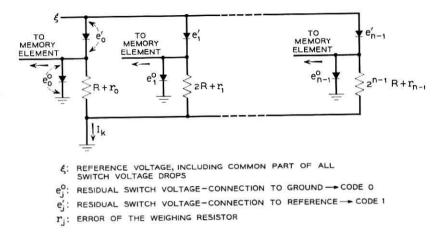
Fig. 22 - Network model for the study of the fine structure effects.
