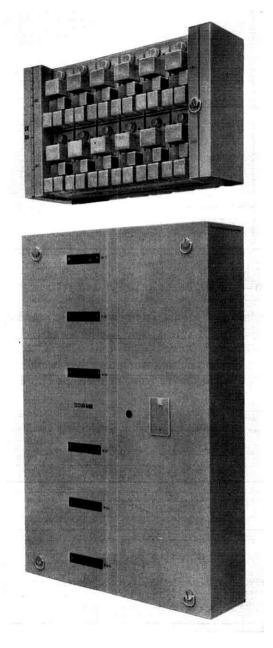
Fig. 9 - Comparison of A5 and A4 channel banks.
