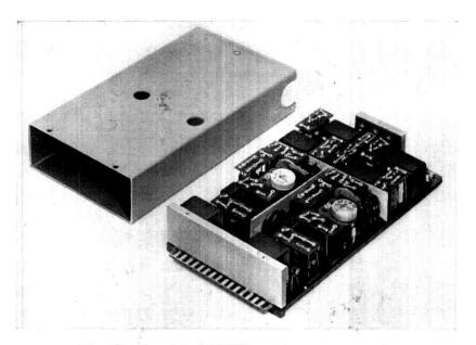
Fig. 48 - Experimental PCM repeater, cover removed.
