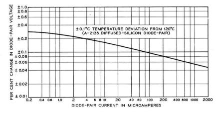
Fig. 14 — Compandor diode temperature characteristic.
