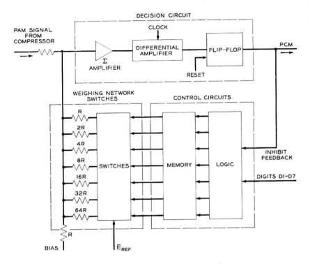
Fig. 19 — Sequential comparison encoder.
