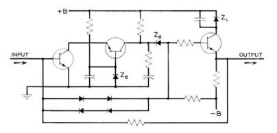
Fig. 24 - Summing amplifier schematic.
