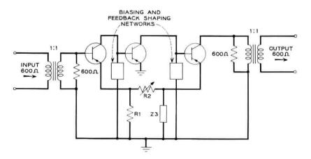
Fig. 3 - Simplified circuit of emitter feedback amplifier.
