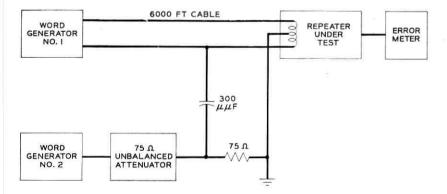
Fig. 54 — Experimental crosstalk simulator.
