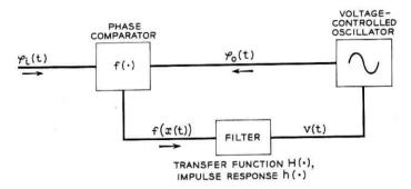
Fig. 1 - Phase-controlled loop.
