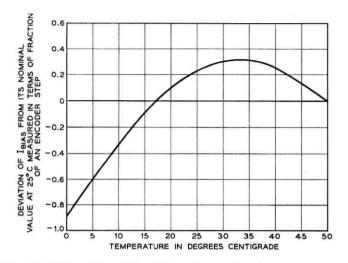
Fig. 29 — Stability of the origin of the code as a function of temperature. The nominal value of  $I_{\text{bins}}$  corresponds to a signal midway between the 64th and 65th encoder decision level.
