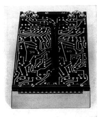
Fig. 50 - Printed wiring of repeater.
