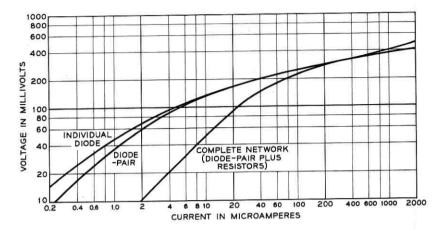
Fig. 11 — Compandor voltage vs current characteristics (diodes at 120°C, resistors at 25°C).
