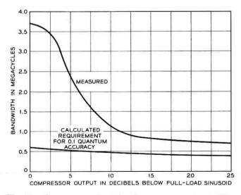
Fig. 18 - Compressor output signal vs compressor bandwidth.
