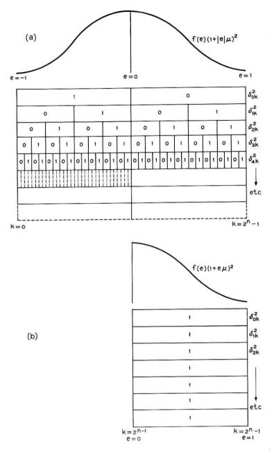
Fig. 31 — The complementary nature of the binary code gives  $\delta_{ik}$  a complementary nature: for example,  $\delta_{ok} = 0$  for all values of  $k \geq 64$ . Because of the complementary nature of  $\delta_{ik}$  and the symmetrical nature of f(e) and  $(1 + |e_k| \mu)^2$  about k = 64, the summation on k of (55) can be reduced to a summation over one-half of the range of interest which is independent of  $\delta_{ik}$ .
