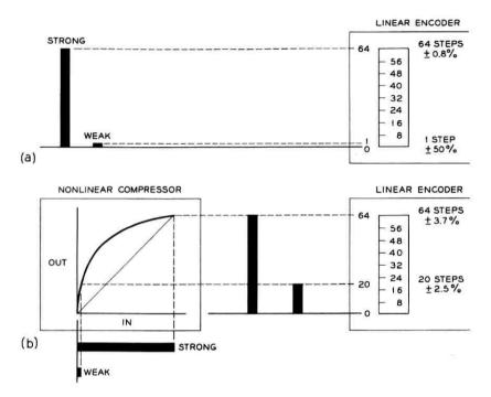
Fig. 1 — Reduction of quantizing distortion.
