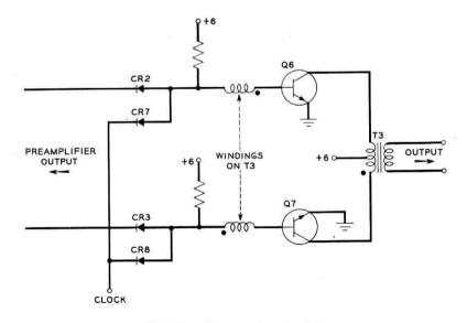
Fig. 34 — Regenerator circuit.
