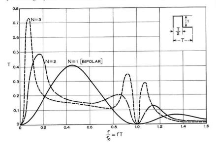
Fig. 12 - N pulse power spectra.
