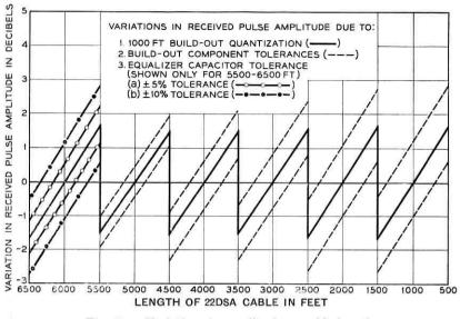
Fig. 21 — Variations in amplitude vs cable length.
