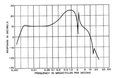
Fig. 15 — Measured preamplifier response.
