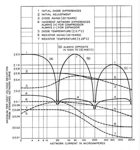
Fig. 12 - Compandor network tolerances that contribute to mistracking.
