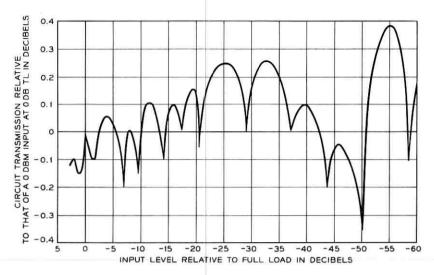
Fig. 14 — Net loss measurements — measured transmission relative to that for a 0-dbm input sinusoid.
