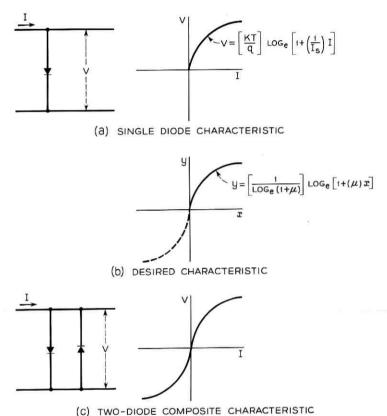
Fig. 8 — Smooth curve approximation to the logarithmic companding characteristic via the voltage-current characteristic of a semiconductor diode.
