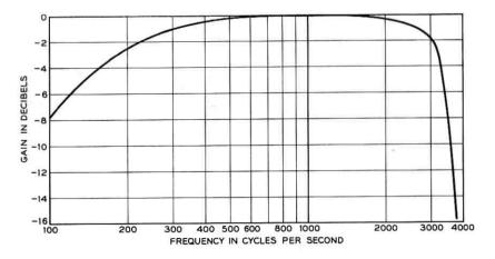
Fig. 6 — Typical bandpass characteristic of the channels.
