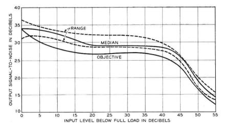
Fig. 4 — Plot of signal-to-noise measurements over 24 channels.
