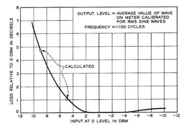
Fig. 17 — Measured signal compression vs input signal level.
