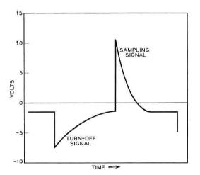
Fig. 32 - Idealized clock waveform.
