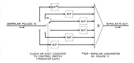
Fig. 13 — Bipolar N block diagram.
