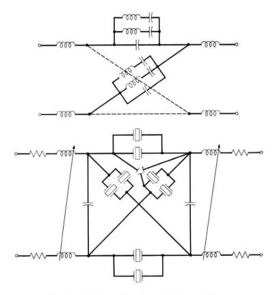
Fig. 14 — Configuration of a crystal channel filter.
