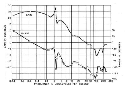
Fig. 16 — Measured open-loop transmission of repeater preamplifier.
