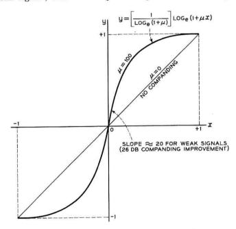
Fig. 2 — Desirable companding characteristic.
