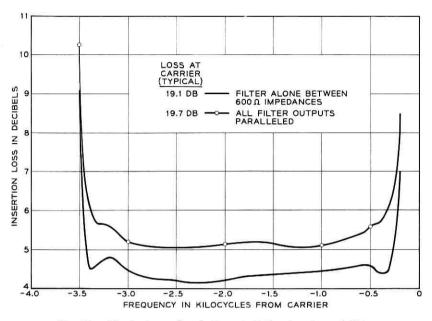
Fig. 17 — Typical pass-band characteristic of a channel filter.
