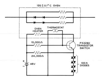
Fig. 17 — Increased thermostat life via transistor gain.
