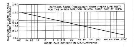
Fig. 13 — Compandor diode-pair aging characteristic.
