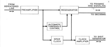
Fig. 52 - Block diagram of receiving repeater.
