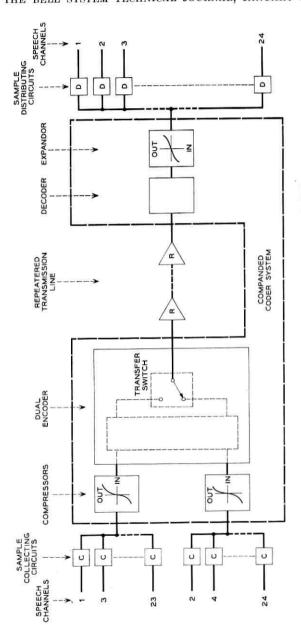
Fig. 5 — Companded coder system for the experimental PCM system.
