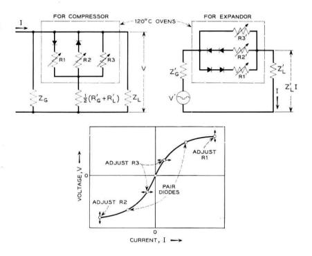
Fig. 9 - Practical companding network (seven-point fit).
