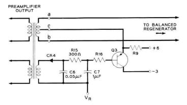
Fig. 23 — Actual threshold circuit.
