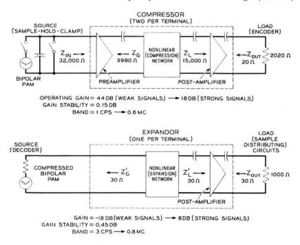
Fig. 7 — Block diagrams showing compressor and expandor.
