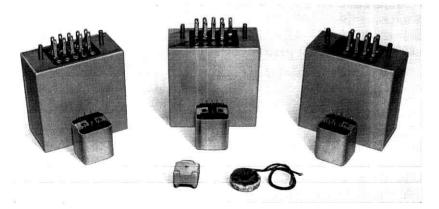
Fig. 18 - Comparison of transformers and inductors used in A5 and A4 banks.
