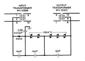
Fig. 41 — Repeater power circuit.
