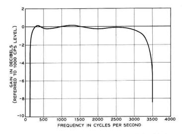
Fig. 19 — Typical channel gain-frequency characteristic of A5 bank.
