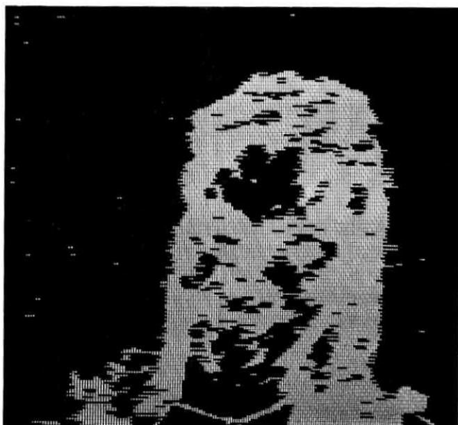
Fig. 7—A display of elements that would be transmitted using cluster coding for the changes in Fig. 4. Isolated changes are ignored and gaps of three or less are bridged.
