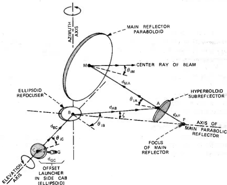
Fig. 9—Beam reflector feed for offset Cassegrainian antenna.
