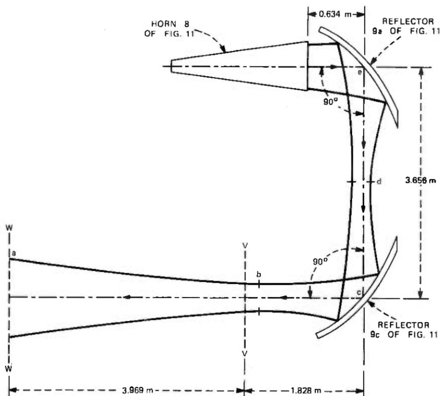
Fig. 12—Unfolded beam waveguide.
