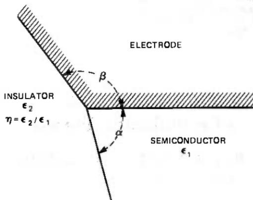
Fig. 1—Electrode, insulator, semiconductor configuration.
