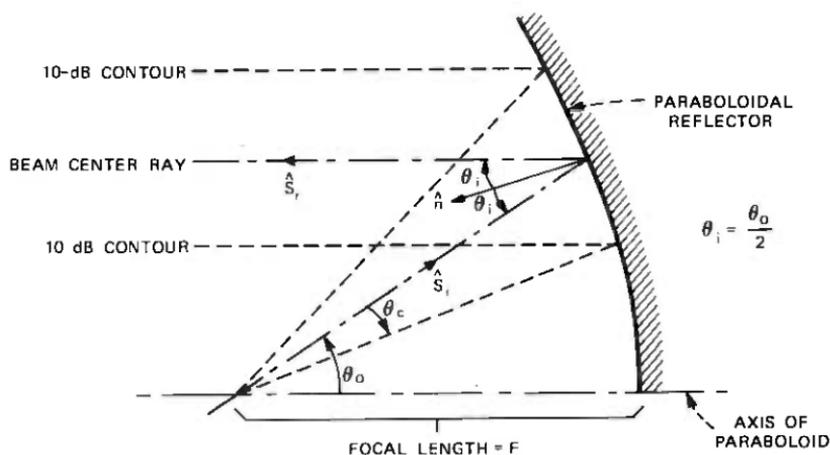
Fig. 2—Offset paraboloid launcher.
