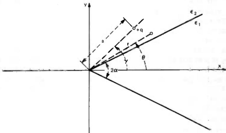
Fig. 2—The dielectric wedge and line charge.
