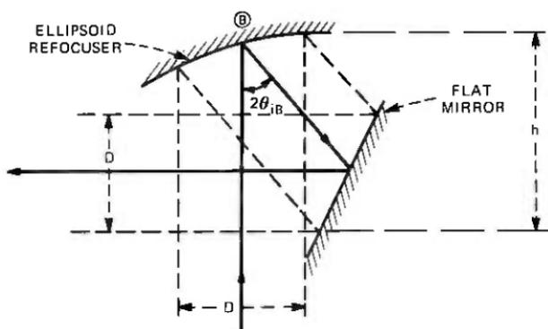
Fig. 10—Combination ellipsoid and flat to reduce  $\theta_{iB}$ .
