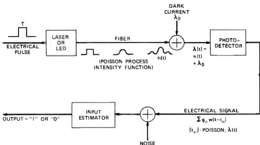
Fig. 1—Passage of a single pulse through the optical system.
