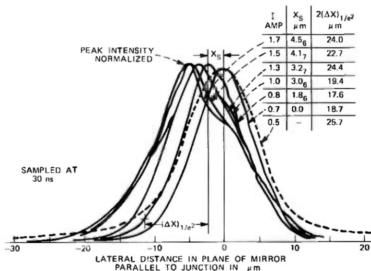
Fig. 9—Output-mirror intensity distribution parallel to junction plane. These mirror scans parallel to the junction plane show that the intensity peak shifts to the left by an amount  $x_s$  with increasing current; simultaneously, a shoulder appears on the right, indicative of multimode output. The values of  $2(\Delta x)_{1/e^2}$  are estimates of the main lobe width.
