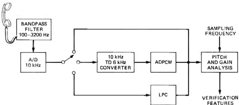
Fig. 2—Block diagram of the data collection system.
