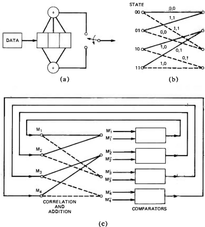
Fig. 8—Viterbi decoding for  $K = 3$ ,  $r = 1/2$  convolutional code. (a)  $K = 3$ ,  $r = 1/2$  encoder. (b) State transition diagram and generated channel symbols. (c) Decoder path metric update.
