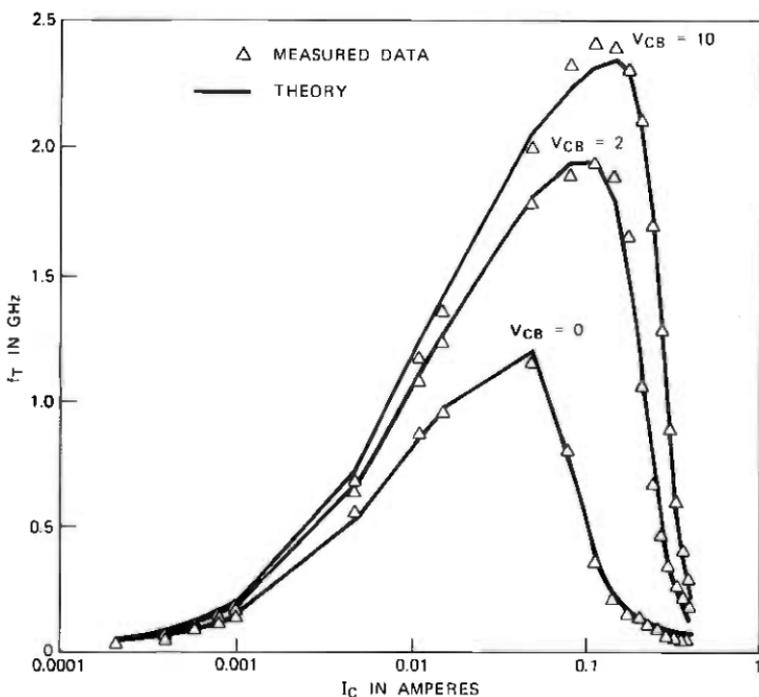
Fig. 25— $f_T$ -current characteristics.
