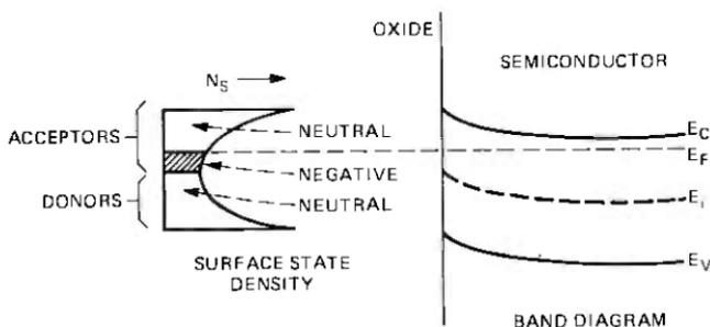
Fig. 8—Charge in surface states.
