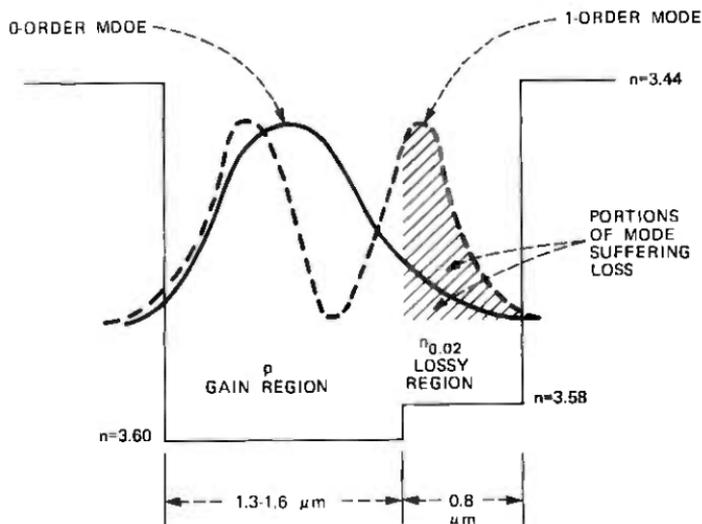
Fig. 4—Mode control perpendicular to junction plane by loss selectivity of optical modes. The  $n_{0.02}$ -layer is made optically lossy by heavy tellurium doping. A larger fraction of the undesired 1-order mode exists within this lossy region than is the case for the desired 0-order mode. By properly controlling the loss and the p- and  $n_{0.02}$ -layer thicknesses, the pulse-current threshold for 1-order lasing can be kept above the currents required for micrographics use.
