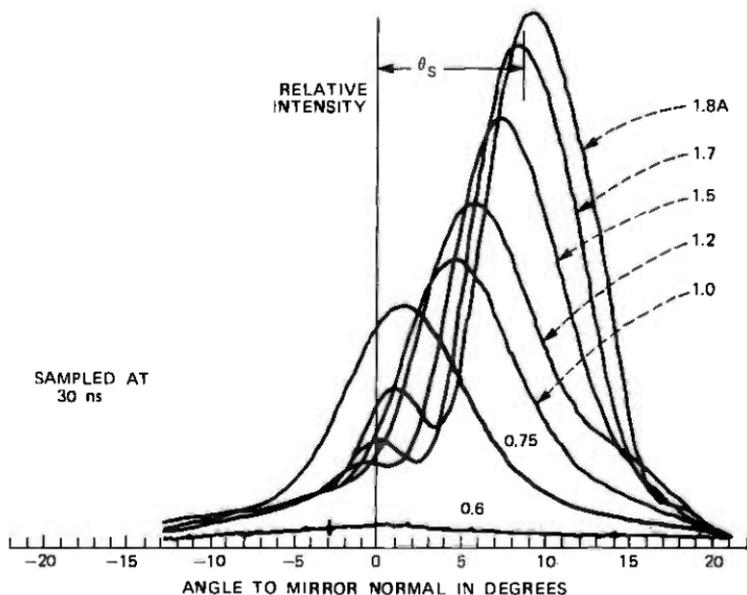
Fig. 6—Intensity angular distribution parallel to junction plane. The angular position of the peak of the far-field intensity distribution parallel to the junction plane defines the beam-steering angle,  $\theta_s$ . Side-lobe structure in the intensity profiles becomes increasingly pronounced as the current is raised. The data were measured 30 ns after the beginning of a 100-ns-duration pulse.
