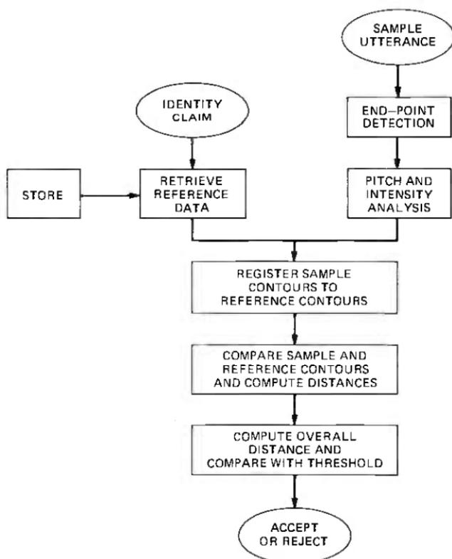
Fig. 1—Flow diagram of the verification system.
