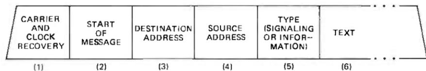
Fig. 5—TDMA burst structure.
