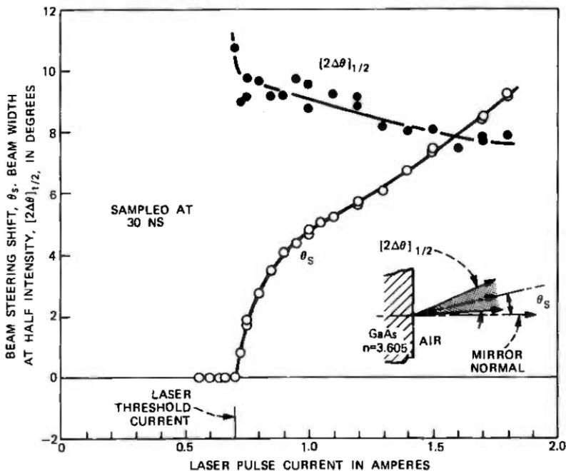
Fig. 7—Dependence on current of beam-steering angle and profile width parallel to junction plane. The far-field intensity full-width at half-maximum amplitude,  $[2\Delta\theta]_{1/2}$ , depends very little on current, whereas the beam-steering angle,  $\theta_s$ , increases rapidly with current and actually exceeds  $[2\Delta\theta]_{1/2}$  at high currents.
