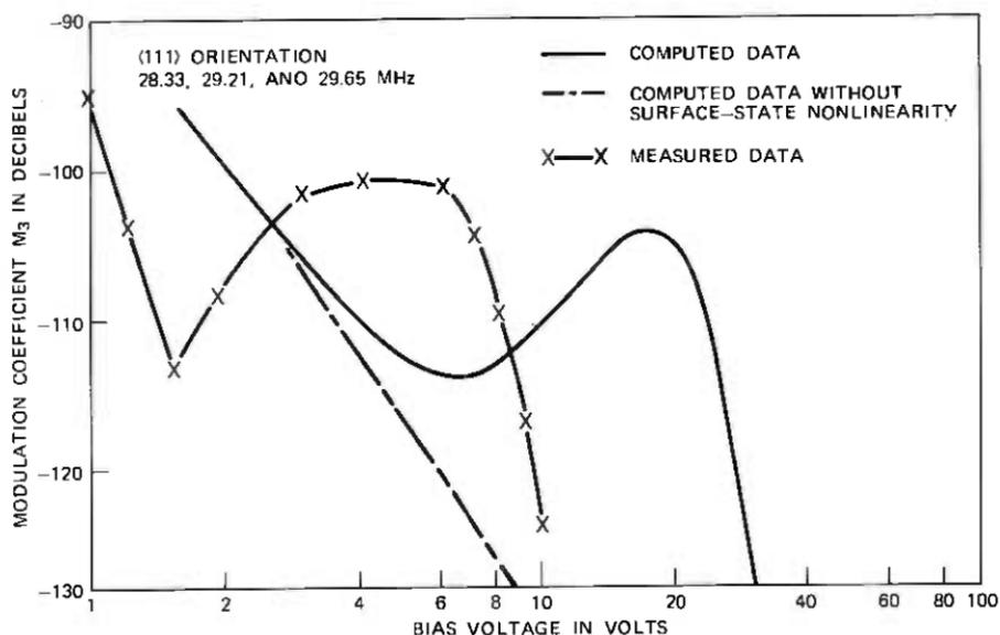
Fig. 15—Intermodulation characteristic.
