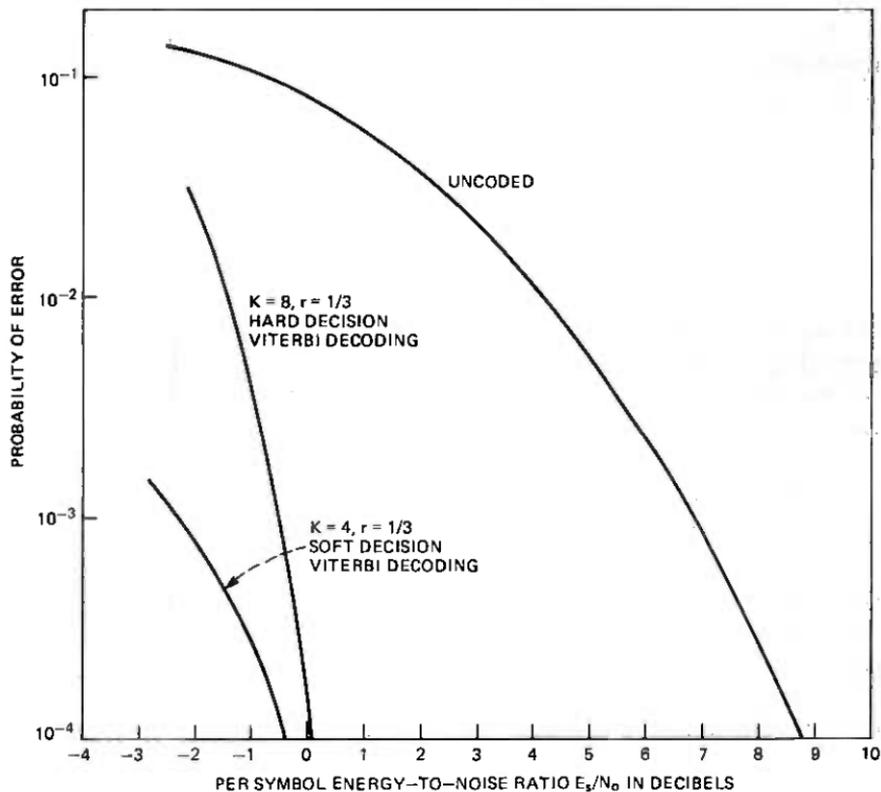
Fig. 3—BER performance for coded and uncoded transmission.
