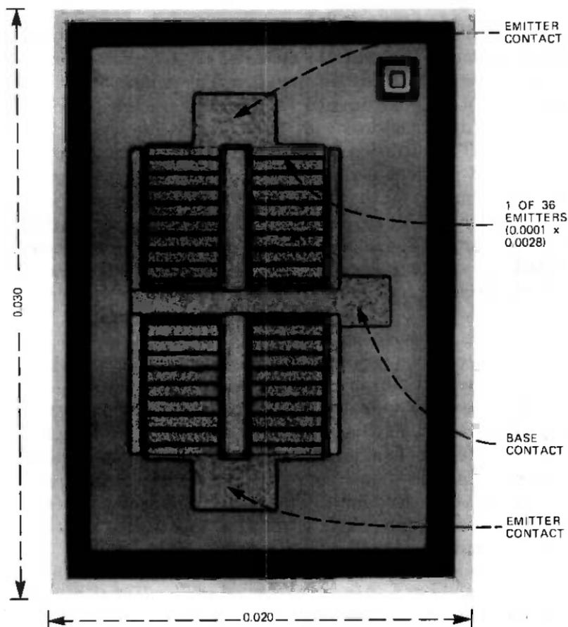
Fig. 3—Transistor chip.
