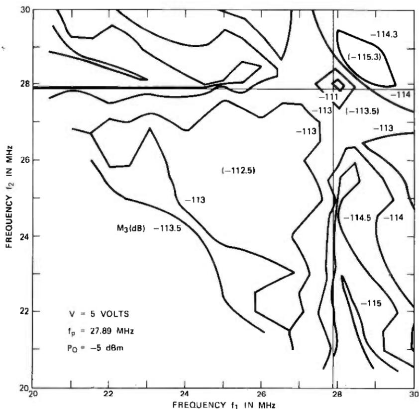
Fig. 21—Measured  $M_3$  frequency map for (100) collector-base junction.
