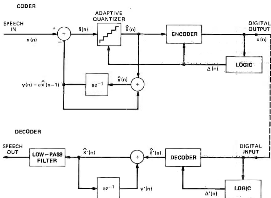
Fig. 3—Block diagram of the ADPCM coder.
