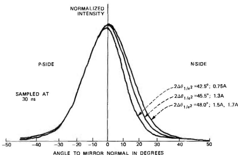
Fig. 8—Intensity angular distribution perpendicular to junction plane. The far-field intensity distribution normal to the junction plane shows evidence only of the 0-order mode. Its width increases slightly with increasing pulse current.
