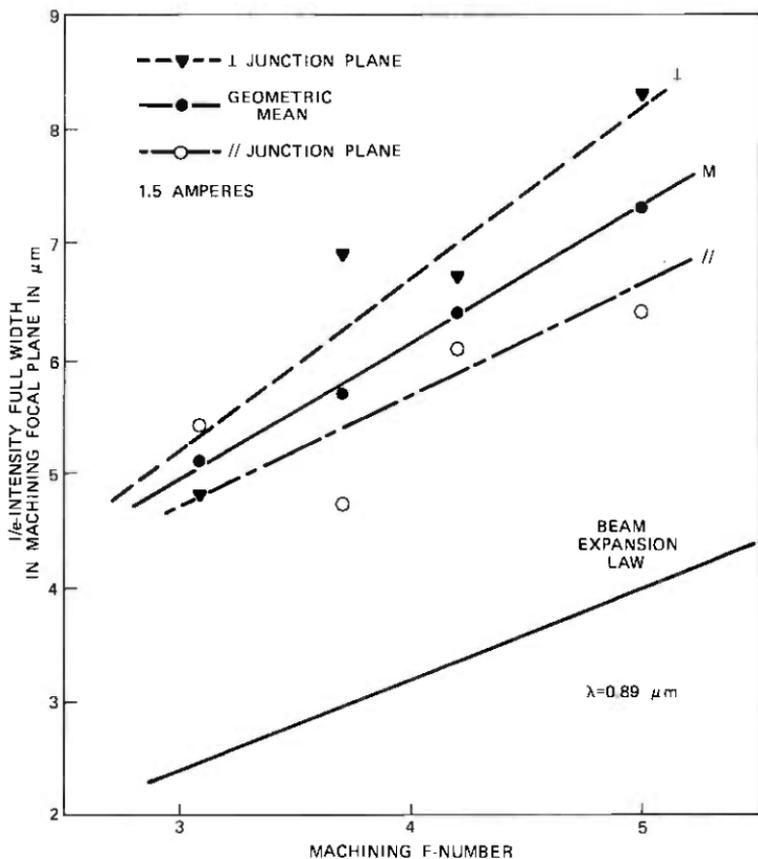
Fig. 33—Numerical-aperture requirements for focusing GaAs beam. The  $1/e$ -intensity full widths of the machining-beam waist measured parallel and perpendicular to the junction plane are plotted versus the machining beam F-number (i.e., the ratio machining-lens-focal-length/collimated-beam-nominal-diameter) for 1.5-A laser current. Predictions of the Gaussian-beam expansion law at  $0.89\text{-}\mu\text{m}$  wavelength are shown for comparison.
