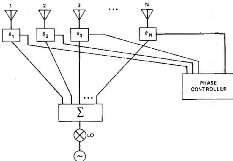
Fig. 1—A phased array with digital phase shifters.
