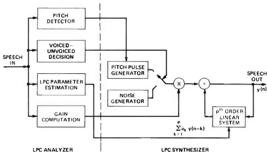
Fig. 4—Block diagram of the LPC vocoder
