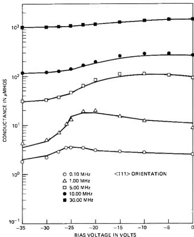
Fig. 10—Conductance of MOS capacitor.
