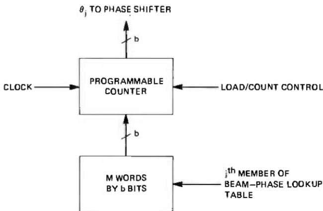
Fig. 11—How to provide phase dither.
