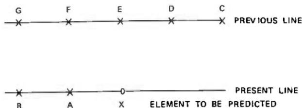
Fig. 1—The configuration of the seven elements constituting the state which is used to construct the predictor used for forward ordering.
