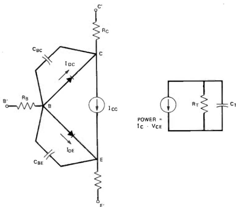
Fig. 24—Transistor model topology.
