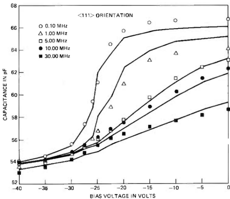
Fig. 11—Capacitance of mos capacitor.
