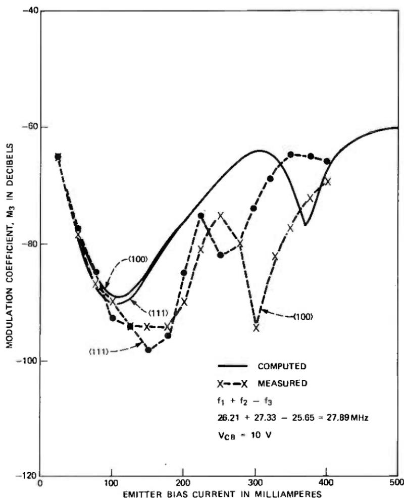
Fig. 28—Transistor intermodulation-current characteristics.
