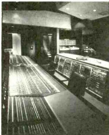
The new SSL I Studio Suite features a Solid State Logic SL-8000 console with Ultimotion.
