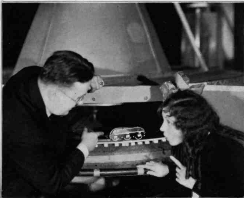
A close-up of the tiny funnel-enclosed car that produces the realistic railroad rhythm of wheels on rails
