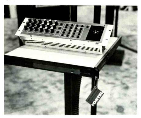
Fortel's new CC2 color corrector is selectable for NTSC, component, or PAL, and it features a Harry-style cursor-location trackball for ease of operation.
