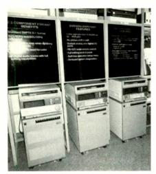
Type-C one-inch made a comeback in popularity and the halfinch wars continued as Sony offered an impressive array of digital video recorders, part of its 4:2:2 digital studio.
