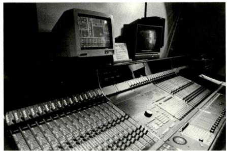
The updated Series X console from Harrison features new VGA Ten interactive graphics for on-screen display of mixing functions.
