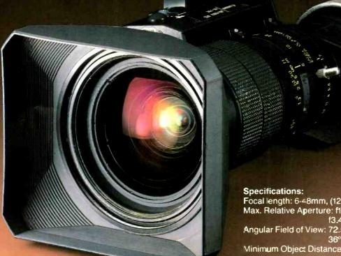
Focal length: 6-48mm, (12-96 w/extender) Max. Relative Aperture: f1.7 (6-33mm), f1.9 at 48mm f3.4 (12-66mm), f3.8 at 96mm
