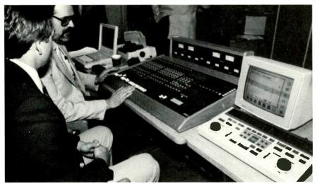
Orion president Richard Hajdu demonstrates the new AMU softwarebased audio mixing system, especially designed for TV audio applications.
