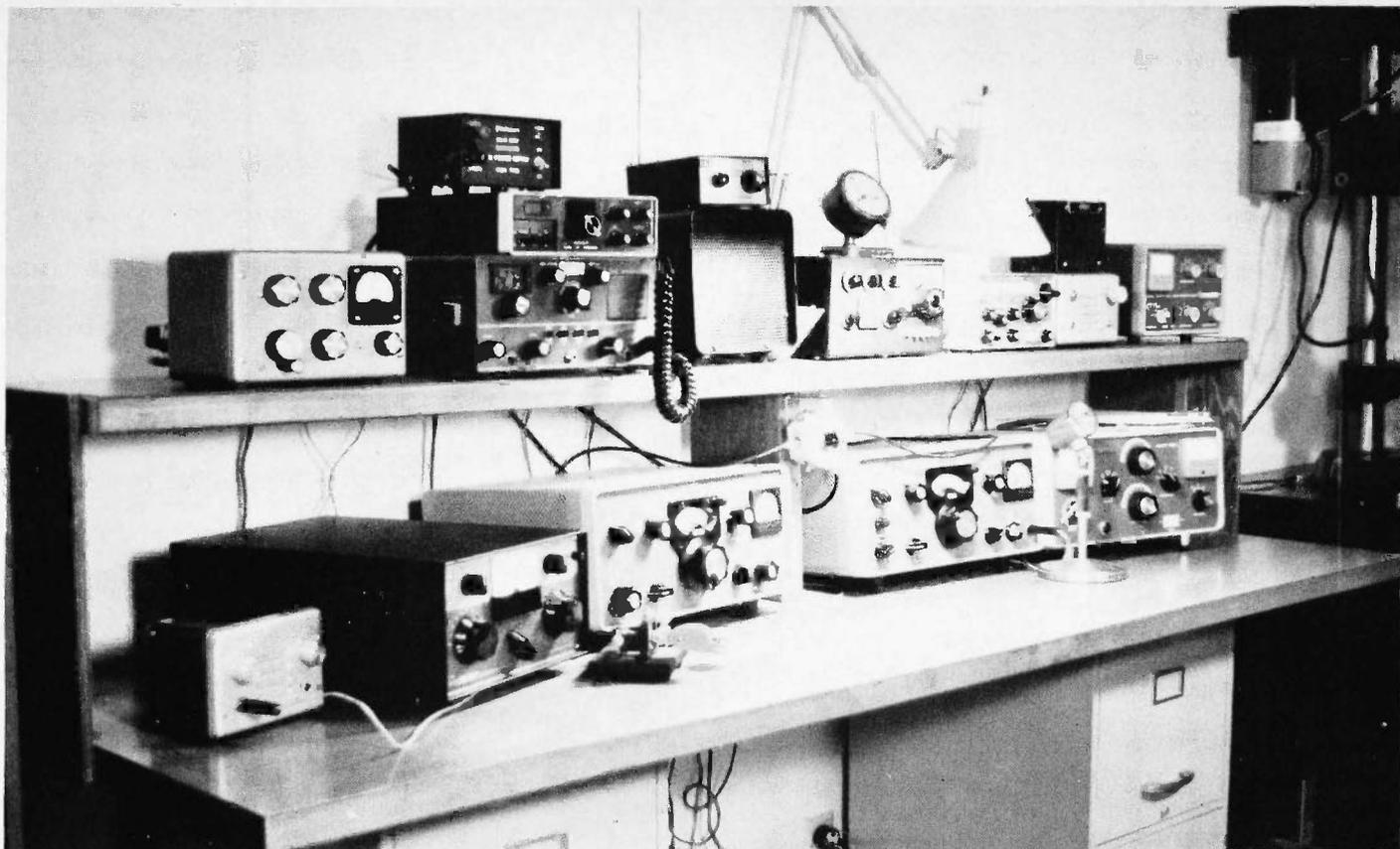
The typical (?) ham radio station has various pieces of equipment. For low band work in "single sideband" (SSB) voice communications, the minimum equipment is a transmitter, a receiver (or combination), plus some form of antenna outside on your roof. Such a setup might cost \$500 in today's markets — although less expensive radio shacks might be set up by buying used equipment with the guidance of experienced hams in your local amateur radio club.
