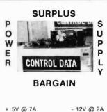
+ 5V @ 7A - 12V @ 2A +12V @ 2.5A +180 V @ 150 ma +30V @ 200ma (unregulated) -6.2V @ 25ma (no adj. pot)
