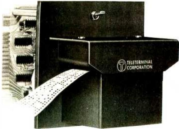
Photo 1: The Teleterminal Corporation Fly Reader for use with the KIM-1 microprocessor.
