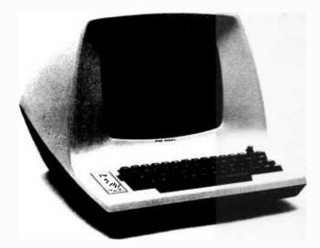
CHARACTER GENERATION 5 x 7 dot matrix. DISPLAY FORMAT Standard: 1920 characters, displayed in 24 lines of 80 characters per line. CHARACTER SET Standard: 64 ASCII characters, displayed as upper case, plus punctuation and control. COMMUNICATIONS RATES 75, 110, 150, 300, 600, 1200, 1800, 2400, 4800,
