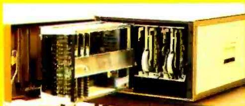
Retainer bar secures circuit cards firmly in sockets.
