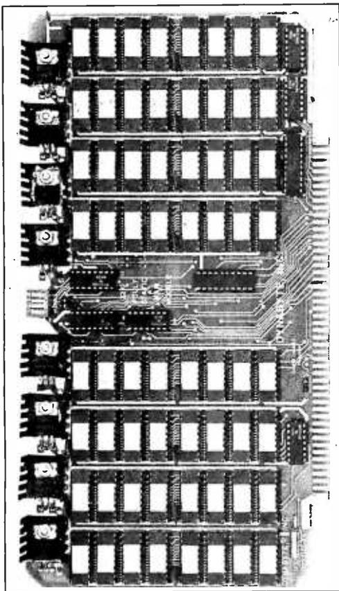
Two fully static programmable memory modules for the Altair (S-100) bus are now available from Dynabyte Inc with access times of either 450 or 250 ns. The 250 ns mode is compatible with 4 MHz Z-80 processors.
