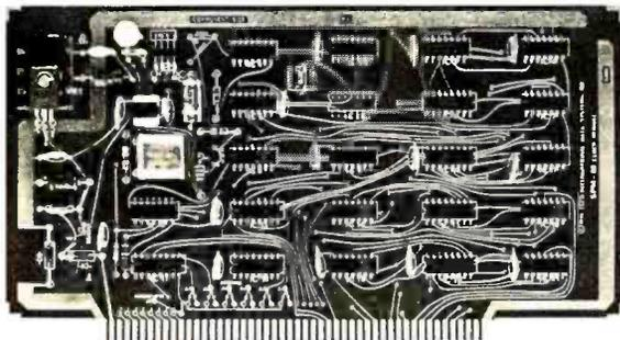
**88-SPM CLOCK MODULE:** The 88-SPM provides a time of day clock and an independent realtime clock on one S100 compatible module. Provisions are included for battery backup so the 88-SPM can maintain the time during power-off conditions. \$96.00 kit
