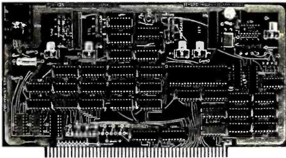
**88-UFC UNIVERSAL FREQUENCY COUNTER:** The 88-UFC is an S100 compatible frequency and period measurement module. The 88-UFC has four software selected inputs. Frequency measurement to above 600MHz and period measurement to 1/10th microsecond are standard. The counter provides nine digits of readout and is priced at \$179.00 in kit form.
