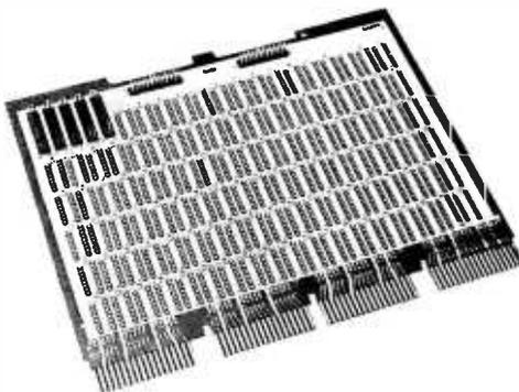
The CIP4 and CIP4/11 universal wire wrapping boards plug into the Digital Equipment Corp standard "Omnibus" and "Q-Bus" backplanes, and provide 32 columns of 60 low profile socket terminals per column with alternate rows of ground and power terminals. The boards will accommodate up to 110 16 pin sockets or an equivalent in other sizes and are priced from \$1.50 to \$2 per chip position, from Garry Manufacturing Co, 1010 Jersey Av, New Brunswick NJ 08902, (201) 545-2424. ■
