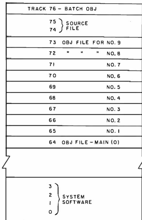
Figure 3: Allocation of the mass storage on a floppy disk. In order to allow quick reloading from the microstations, the current microstation object file is kept for each microstation, dedicating one track per microstation and one track to the main computer's object file. Thus if a program blows up in a student's system, it can be reloaded (and patched) without reassembly.
