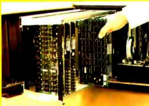
System Three front panel swings open and 21-slot motherboard/card cage slides forward for easy insertion of extra circuit boards.
