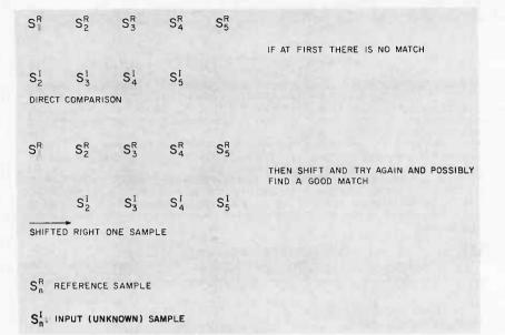
Figure 16: Shifting the unknown left and then right one position helps prevent mismatches due to missing ends or beginnings. In this case the right shift gave a good match. This test has been simplified to one parameter (S) which might be the output of one filter in a filter bank.
