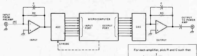
amplifier, needn't have as sharp a cutoff, but it should have the same cutoff frequency as the input filter. For the simple filters in figure 1, the cutoff frequency is equal to  $1/2\pi$ RC, where R and C are the values of the feedback resistor and capacitor, respectively.
