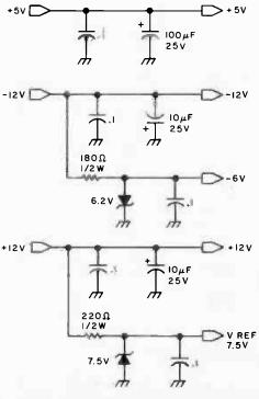
Figure 3c: Power supply circuitry for figures 3a and 36.
