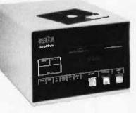
The DataMate minifloppy disk system is a data storage and editing unit for connection between any RS-232 asynchronous ASCII coded printer or display terminal and its modem. Features include 560 addressable records of up to 128 characters each, selective data transfer rates of up to 9600 bps, editing capabilities, search modes, and manual and remote controls. The price is \$1750 from Western Telematic Inc, 2435 S Anne St, Santa Ana CA 92704.
