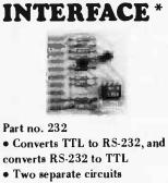
converts RS-232 to TTL • Two separate circuits • Requires -12 and +12 volts • All connections go to a 10 pin gold plated edge connector • Board only \$4.50; with parts
