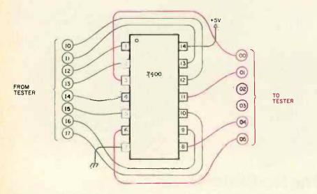
Figure 2: One method of hooking the tester up to a 7400 TTL integrated circuit.
