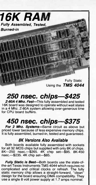
Fully S-100 Bus Compatible—Each 4K addressable to any 4K slot and separately protected by DIP switches.
