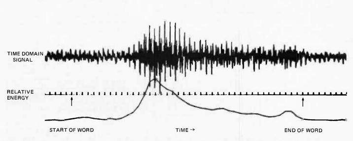
Figure 1: A time domain voice waveform and its energy. The top trace is the time domain signal for the word "three." The bottom trace is the energy in the above signal computed every 10 ms. Note that the signal before and after the word (arrows mark the beginning and end of the word) is not zero. This is due to background noise picked up by the microphone, in this case computer cooling fans and air conditioning noise.
