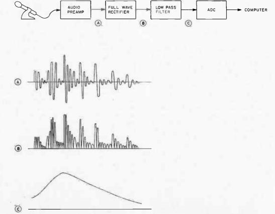
Figure 3: Rectifying the microphone signal at A we obtain signal B which contains a slowly varying DC component proportional to the volume of the signal and various high frequency components due to the formants. The low pass filter separates these and the analog to digital converter (ADC) the volume sees only signal.
