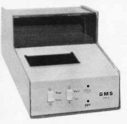
General Micro-Systems' new tape drive subsystem is a fast, inexpensive, high capacity mass storage device for microcomputers. The SYS 1 records biphase Manchester code at 1600 bits per inch on ANS1 specified data cassettes with a transfer rate of 2000 characters per second at ten inches per second.
