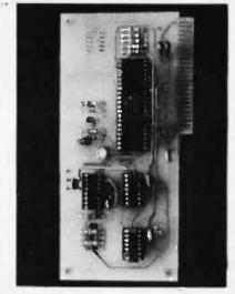
Electronic Systems has announced a serial IO board for the Apple II computer. The board comes with software for input and output to and from a Teletype or other serial device via an RS-232 interface.
