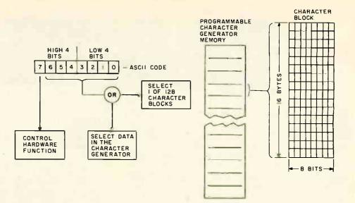
Figure 2: Decoding the code byte. The highest order bit of the 8 bit code is used for control hardware functions (such as reverse video). The remaining seven bits select character blocks in the character generator read only memory, the programmable character generator, or both (depending on what mode of operation is being used). Each data block consists of 16 bytes with eight bits. The 1s and 0s are converted to screen dots and spaces by the hardware.
