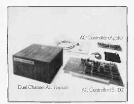
A new system designed to control AC devices remotely from any Altair (S-100) bus or Apple II computer over existing 110 VAC wiring has been announced by Mountain Hardware, POB 1133, Ben Lomond CA 95005. The new unit,
