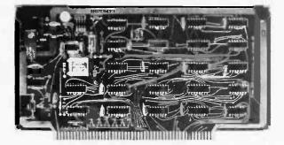
88-SPM CLOCK MODULE: The 88-SPM provides a time of day clock and an independent realtime clock on one S100 compatible module. Provisions are included for battery backup so Ihe 88-SPM can maintain the time during power-off conditions. \$96.00 kit
