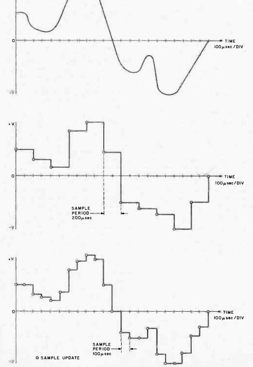
Figure 2c: Waveform in figure 2a after being processed through a digital to analog converter at a sample rate of 10,000 samples per second. 25 samples within a period of one second could not effectively record the event. At what sampling rate should audio speech be digitized?
