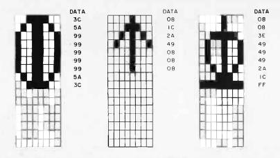
Figure 4: Some arbitrary special characters. The 16 bytes that form a character are projected onto a 16 by 8 grid, each bit corresponding to one space. The programmer can choose any combination of 1s and 0s to create filled and empty spaces, respectively.
