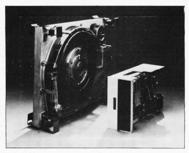
Photo 3: Shugart SA4000 fixed disk drive (left) next to standard SA800 floppy disk drive.
