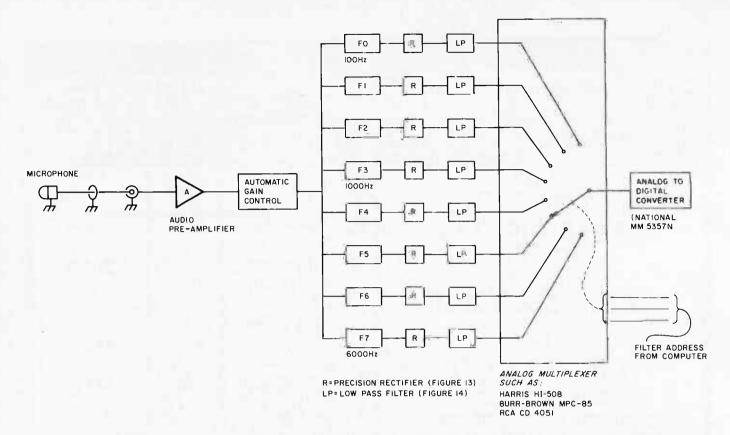
Figure 12: A detailed block diagram of a filter bank feature extractor. The output of the eight bandpass filters is sampled and digitized every 10 ms. Spectral information as well as word boundaries can be extracted from this set of data. See text for an extensive description of this particular implementation.
