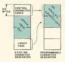
Figure 3: Automatic mode. In this mode, the upper case characters come from the existing character generator while the control character and lower case codes automatically reference 64 special characters in the programmable character generator memory. This is probably the most convenient mode of operation for many applications, since the normal upper case character set is available along with the special graphics characters.
