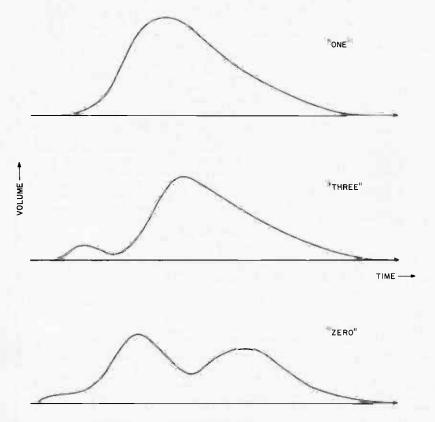
Figure 4: Amplitude envelopes of the words "one," "three," "zero." Note that "one" has one hump while "three" has two. The smaller one corresponds to "th" and the larger one to "ee." In "zero," "z" is the low amplitude area in the beginning. The dip corresponds to "r" and the humps to "e" and "o." Vowels always have high amplitude because they are produced with the mouth open and with strong excitation.
