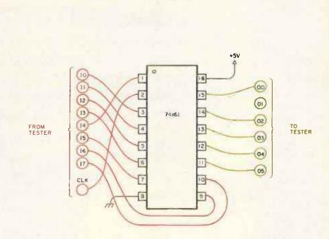
Figure 3: Tester hookup for a TTL 74161 integrated circuit. Note the use of the clock line coming from the tester. This is to ensure that the integrated circuit receives clock signals of the proper speed relative to the other test input lines.
