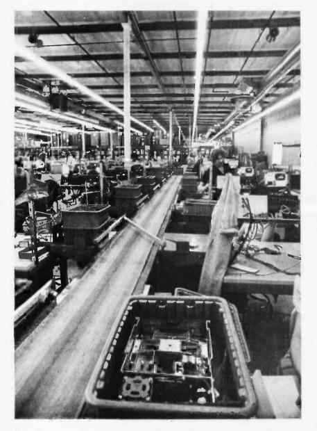
Photo 1: One of the high speed conveyors at Shugart Associates' Sunnyvale CA plant. Metal arms swing out to capture plastic bins of parts. 600 to 800 floppy disk drives and 300 to 400 minifloppy drives are turned out every day at the plant.
