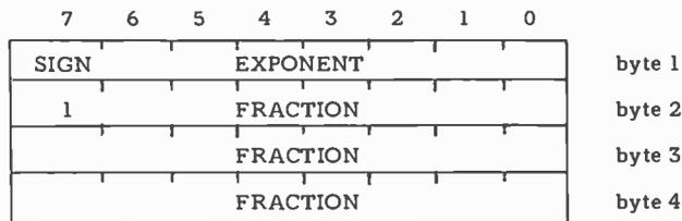
Figure 1: Format for the arrangement of data in the computer's memory for the binary floating point representation described here. The high order bit of byte 2 will usually be '1' because of normalization. The only time that this will not happen is when the number being represented is zero.
