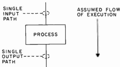
Figure 1: The process block is the "black box" of programming: it is entered by a single input path, does some arbitrary operations upon data, and is exited by a single output path. The "arbitrary operations" can be as simple as one step in an arithmetic calculation, or as complex as a compilation of a program — it all depends on the point of view taken.
