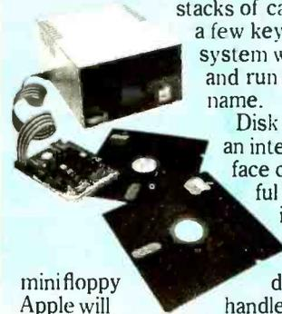
Disk II consists of an intelligent interface card, a powerful Disk Operating System (DOS), and one or two drives. Your mini floppy Apple will handle up to seven inter face cards and fourteen drives, for control of nearly 1.6 megabytes of data, with no expansion chassis. The combination of ROM-based bootstrap loader and an operating system in RAM provides complete disk handling capability, including these special features:
