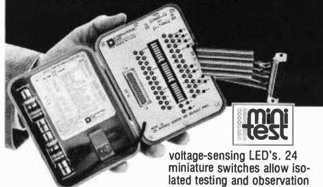
Our Model 60 is called "The Blue Box" by thousands of users. This compact unit packs the most testing capability per dollar. Pinpoints the source of trouble between the Modem and Terminal. Provides access to all 25 lines of the EIA RS 232 interface. Has 12 monitoring LED's plus two
