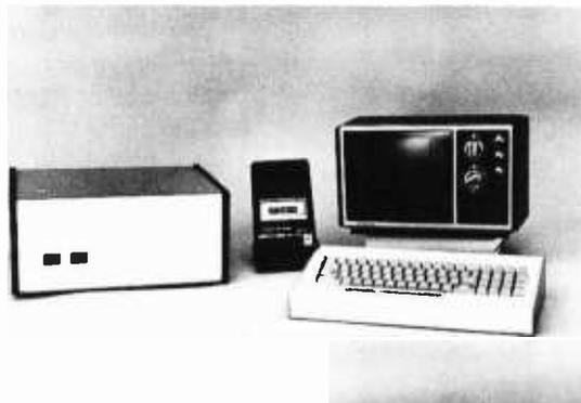
Central Data also offers, fully-assembled and in kits, a range of other computer products including (pictured above) our 2650 microprocessor, software packages, TV/Monitor, ASCII keyboard, and (not pictured) floppy disk system, to name just a few.
