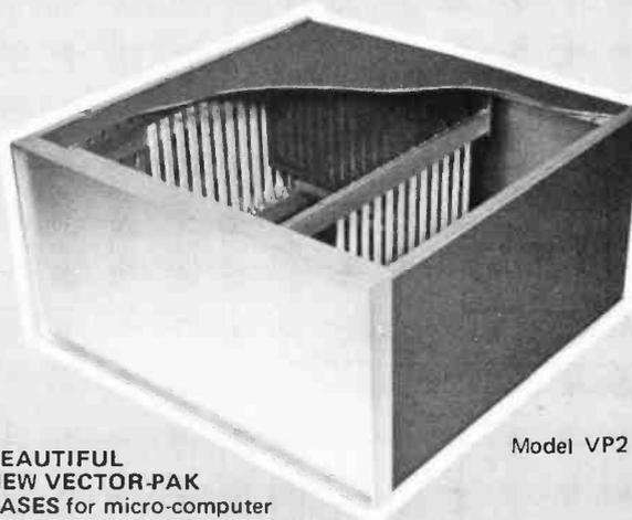
**BEAUTIFUL NEW VECTOR-PAK CASES** for micro-computer circuitry, assembled. Constructed of aluminum, finished in vinyl. Slide out covers for easy access. Includes card guides, heavy chassis plate, perforated bottom cover for cooler operation. Card guides perpendicular to front panel, Model VP1, \$163.00. Card guides parallel to front panel, Model VP2, \$159.00.
