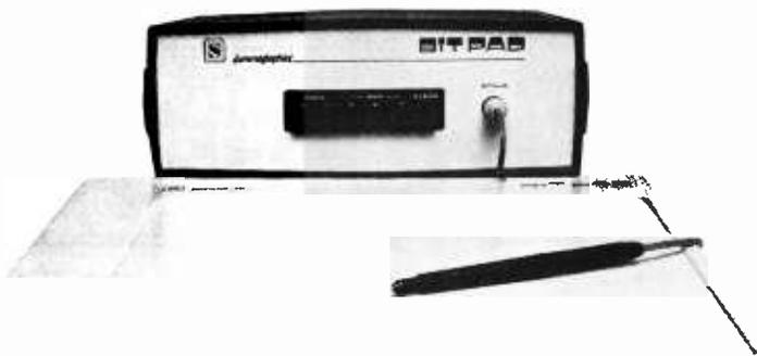
Bit Pad is the low-cost digitizer for small computer systems. Better than a joystick or keyboard for entering graphic information, it converts any point on a page, any distance into its digital equivalents. It's also a menu for data entry. You assign a value or an instruction to any location on the pad. At the touch of a stylus, it's entered into your system.
