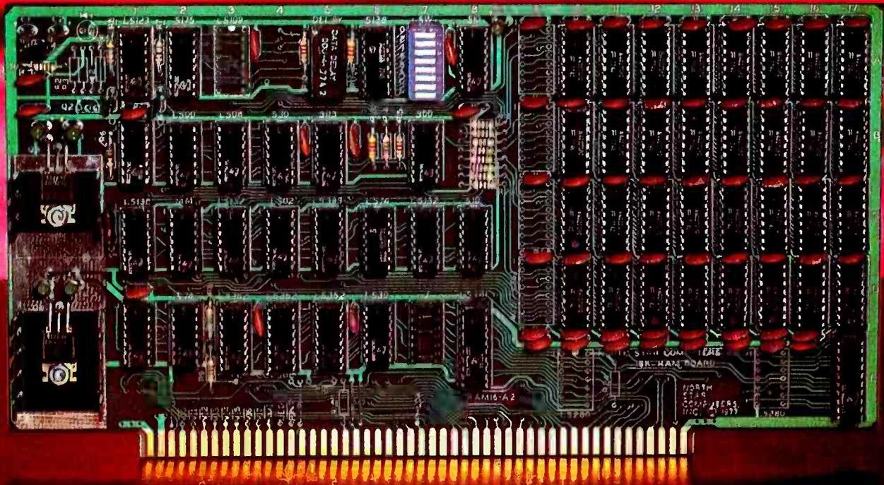
**The North Star 16K RAM board** is a star performer in our HORIZON computer. Just as important, it is the ideal memory for most other S-100 bus systems. No other RAM board can surpass the speed, reliability, and quality features of the North Star 16K RAM at any price.
