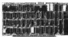
**Naked Terminal.** 80 character x 24 line = 1920 character display capacity. Not just a video interface but a full terminal; plug into a mainframe with keyboard and monitor and save! Upper and lower case; black/white or white/black; block mode editing; addressable cursor; half and full duplex; no software support required; addressable status and I/O ports, \$350.
