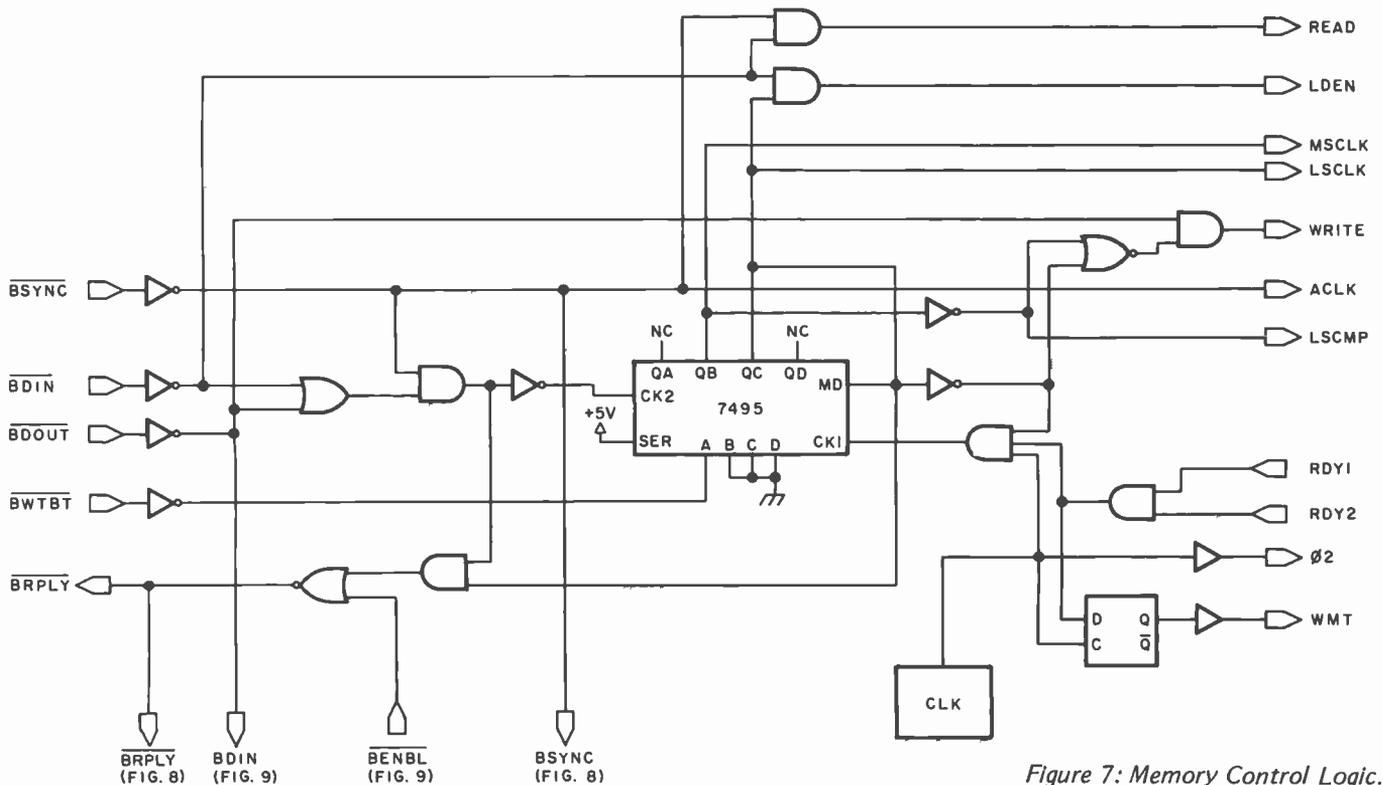
Figure 7: Memory Control Logic.
