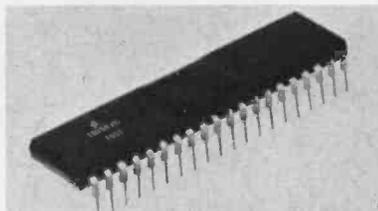
The TR 1983 bus oriented universal asynchronous receiver transmitter (or UART) that is fully compatible with the asynchronous capabilities of the 8251 UART is now available from Western Digital Corp, 3128 Red Hill Av, POB 2180, Newport Beach CA 92663. It has a 28 pin package pinout that allows direct replacement of the 8251. The TR 1983 features full or half duplex operation, and is powered by a single +5 V supply. For further information, write to the company. ■
