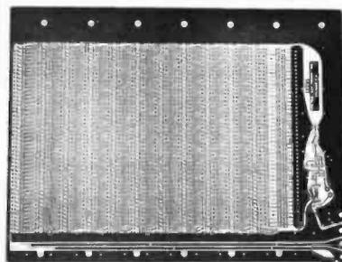
**S100 MOTHERBOARD, \$29.50.** 11 positions ready for connectors. Glass epoxy, etched circuitry for passive or active termination, 12 tantalum capacitors and instructions.
