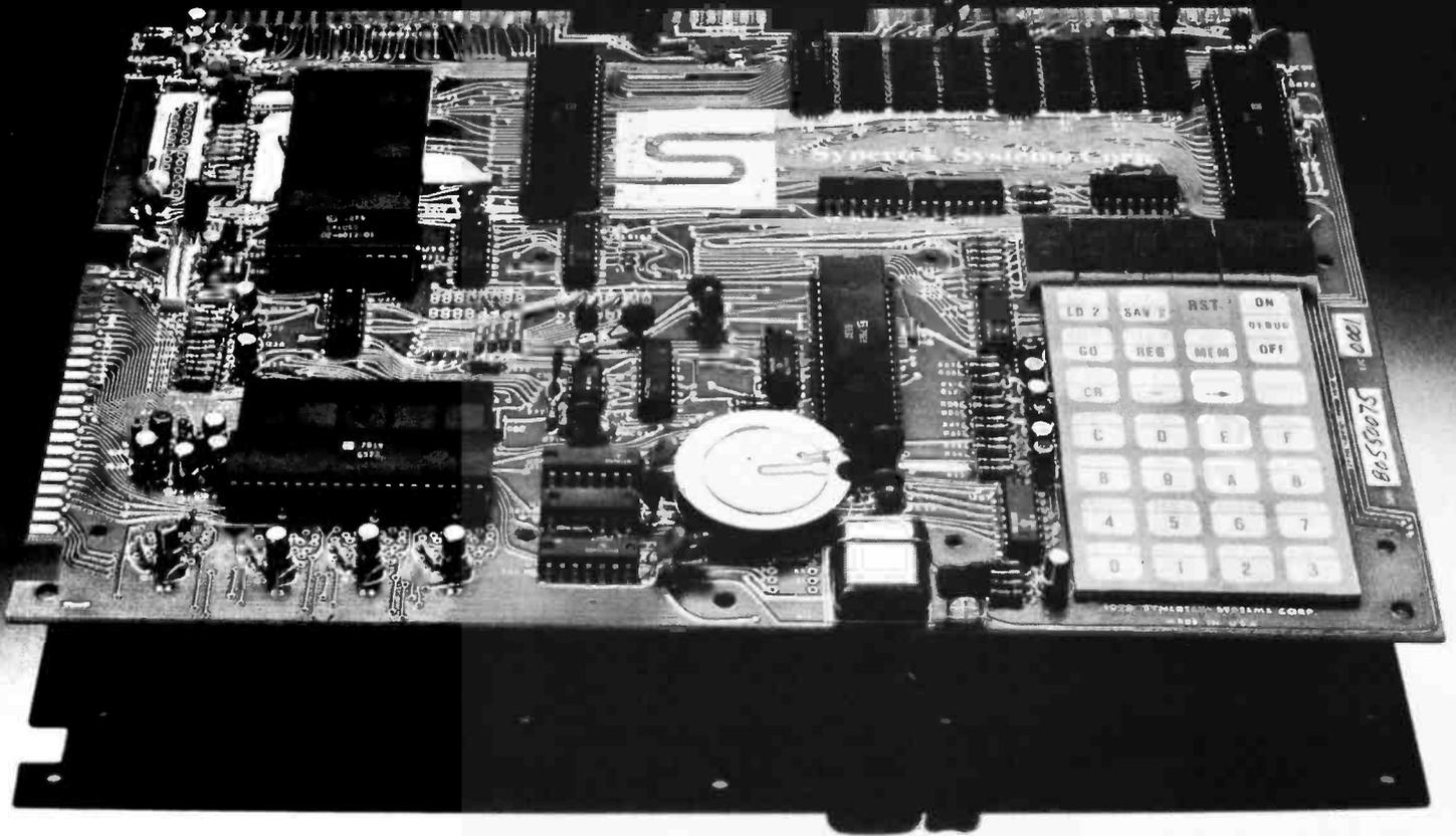
In performance. In quality. In availability. OEMs, educators, engineers, hobbyists, students, industrial users: Here's our Versatile Interface Module, a fully-assembled, tested and warranted microcomputer board that's a true single-board computer, complete with keyboard and display. All you do is provide a +5V power supply and the Versatile Interface Module gives you the rest—and that includes fast delivery and superior quality.
