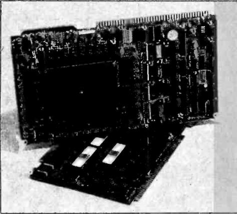
This 16 K byte core memory for 8080 microcomputers is now available from Ampex Corp, 200 N Nash St, El Segundo CA 90245. Fully compatible with SBC 80 single board computers, the MCM-8080 provides nonvolatile storage for 16 K bytes with a data access time within 325 ns. The read and write cycle times are 780 and 1240 ns, respectively.
