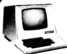
The Hazeltine 1400 Video Display Terminal is designed to optimize interactive real-time operations. The interface is capable of either local or remote connection through an EIA RS232-C interface at baud rates that are switch selectable up to 9600 baud.
