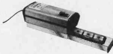
shortwave UV tube, a specular reflector, and a V shaped holding tray that maintains up to six chips at a constant exposure distance. The high intensity tube is fully protected within the anodized aluminum housing, and a safety interlock prevents the unit from operating when the tray is not fully inserted. The conductive foam pad holds the chip in place during exposure and prevents electrostatic build up, while protecting the chip from possible static charge. ■
