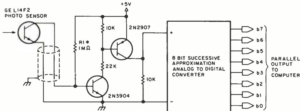
\*Raising the value of this resistor will increase sensitivity. Lowering it will reduce sensitivity (range of resistor values is 4.7 k to 3.3 M $\Omega$ ).
