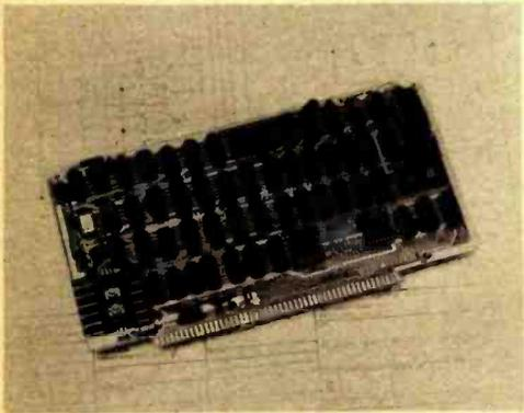
Requiring +8 VDC at 1.2 A, the Flashwriter generates a video display of 1024 characters arranged as 16 lines of 64 characters each and uses a 7 by 9 dot matrix to produce a high quality, high
