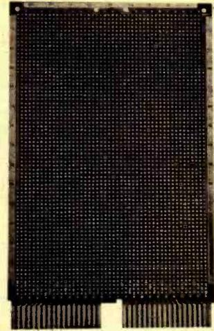
This new general purpose prototyping circuit board permits construction of custom interface circuits for Heath H11 microcomputers and Digital Equipment Corp LSI-11, PDP-8 and PDP-11 minicomputers.
