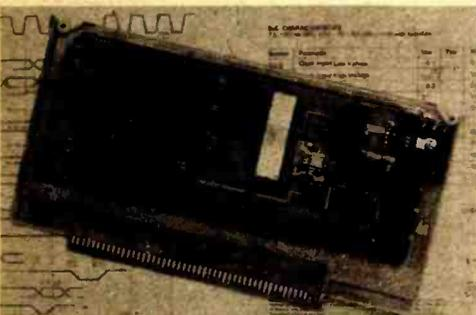
This new Z-80 processor board is offered assembled or in kit form. The board offers fully blocked design with on board wait state select, and is jumper selectable for operation at 2 MHz or 4 MHz. The board will operate standard 8080 software without modification. All Z-80 lines are fully buffered.
