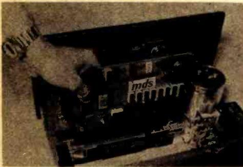
The MD-690 is an S-100 compatible processor board featuring the Motorola 6800 processor. This processor uses the MC6802 which combines the instruction set of the 6800 with internal programmable memory and crystal controlled clock.
