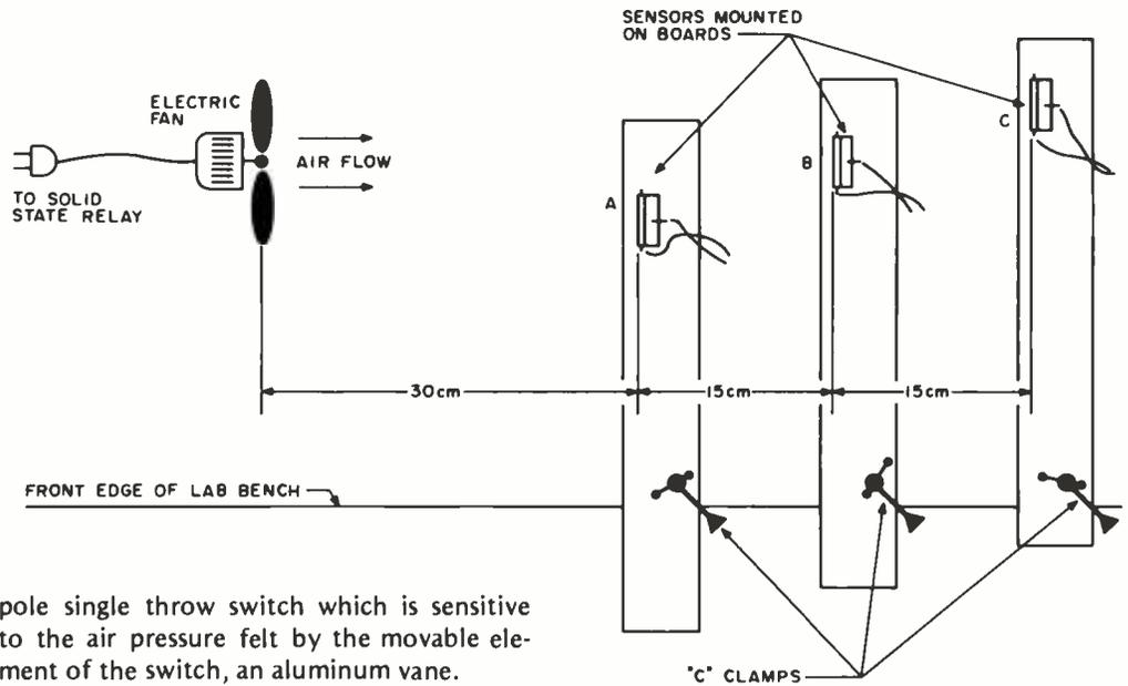
pole single throw switch which is sensitive to the air pressure felt by the movable element of the switch, an aluminum vane.
