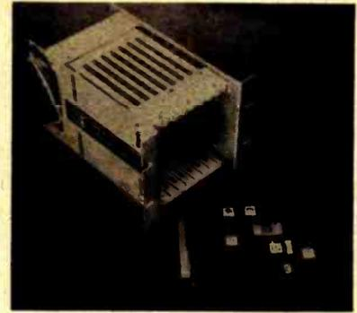
This new single board computer contains a processor, memory and IO on a single 4.5 by 6.5 inch (11.4 by 16.5 cm) card. The Model OB8001 also includes serial communications interface meeting both the 20 mA current loop and RS-232C standards. The microcomputer using the 6800 processor can be used to implement a wide variety of stand alone controllers. The processor module is available without chassis as a stand alone computing system with standard card edge connectors.
