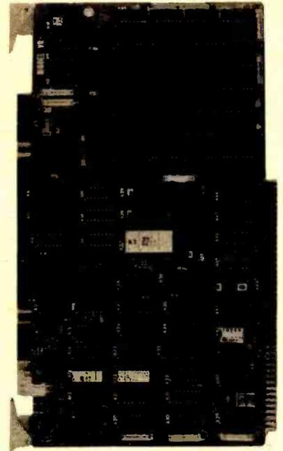
The Datacube VR-106 video programmable memory board provides 80 by 24, 80 by 12, 40 by 24 or 40 by 12 character display formats under software control. The display consists of 128 upper case, lower case and Greek characters in a 7 by 7 or 7 by 9 font. A bipolar programmable read only memory character generator can be used for reverse video, underline, half intensity, blinking or graphics block.
