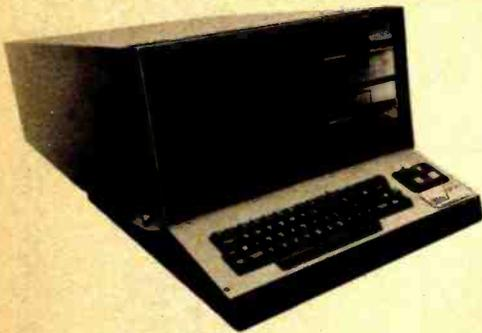
The VPD-40 is a fully integrated system featuring an 8085 processor, 32 K bytes or 64 K bytes of programmable memory, twin minifloppies, a video display, programmable keyboard, motherboard and serial and parallel IO ports in a flip top cabinet. Supporting software includes a disk operating system, text editor, extended and commercial BASIC, relocatable assembler, linkage editor, debugging program, floppy disk system diagnostic program
