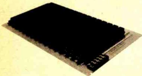
Compatible with the S-100 computer systems, the Artec shielded motherboard is made of 0.125 inch (0.32 cm) FR4
