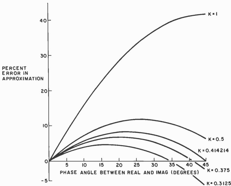
Figure 1: A plot of the percent error in the magnitude approximation for different values of K. We are approximating the square root of  $REAL^2 + IMAG^2$  by the formula  $L + KS$ , where L is the larger and S is the smaller value of the absolute values of the real and imaginary parts of a vector.
