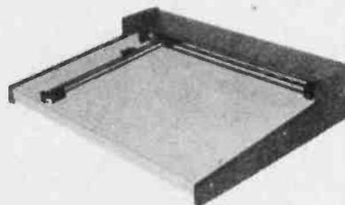
This X, Y plotter includes a plotter, drawing surface, electronics, and power supply completely assembled and ready for interface to any 8 bit transistor-transistor logic parallel port. The pen holder accepts any writing instrument or stylus 7 to 11 mm in diameter, encoded for 0.01 inches per pulse (0.005 inch optional). The maximum pen travel speed is 2.5 inches per second with a 24 V supply. A basic 8080
