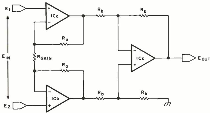
$$E_{OUT} = \left(1 + \frac{2R_a}{R_{GAIN}}\right) (E_2 - E_1)$$
