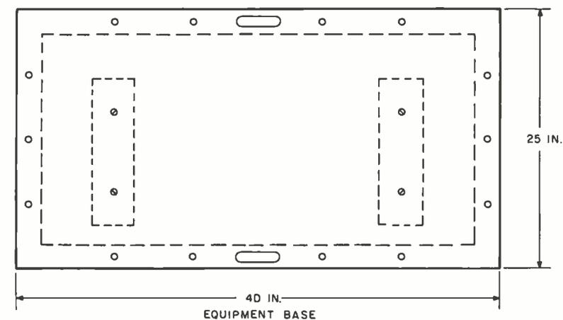
Figure 1: Plans for building the author's computer system cabinet. The unit is built from 5/8 inch plywood and features two U-bolts for adding an antitheft chain. All components are mounted on the floor of the cabinet. See accompanying photos.
