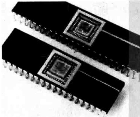
Zilog Inc has announced the availability of a Z8000 microcomputer processor circuit that offers users the architectural resources of mini and large mainframe computers in a single circuit device. The processor is available in two versions: the Z8001 in a 48 pin ceramic dual-in-line package that allows the user to address up to 8 M bytes of memory; and the Z8002 in a 40 pin ceramic dual-
