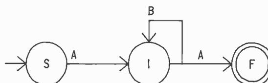
Figure 3: A lexical finite state machine for recognizing the entities that will be accepted by the game: <TO>, <TAKE>, <MOVE>, <CAP>, <FROM>, <END>, <POS>.
