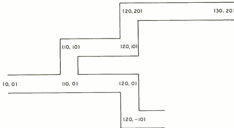
Figure 6: Maze pitfalls. On its first, nonoptimized attempt, the mouse will traverse the entire length of the dead-end corridor. After optimizing the path by deleting backtracked corridors, a shorter path is taken.
