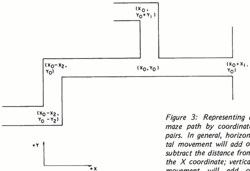
Figure 3: Representing a maze path by coordinate pairs. In general, horizontal movement will add or subtract the distance from the X coordinate; vertical movement will add or subtract from the Y coordinate.
