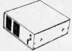
Accommodates all S-100 Mother Boards. Built-in card cage with card guides. Lighted reset switch. Rotron whisper fan. Includes heavy duty power supply. (+8 volts DC @ 30 AMPS, +16 volts DC @ 4 AMPS, -8 volts DC may be added.)
