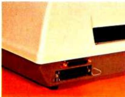
serial character synchronous Centronics compatible interface.
