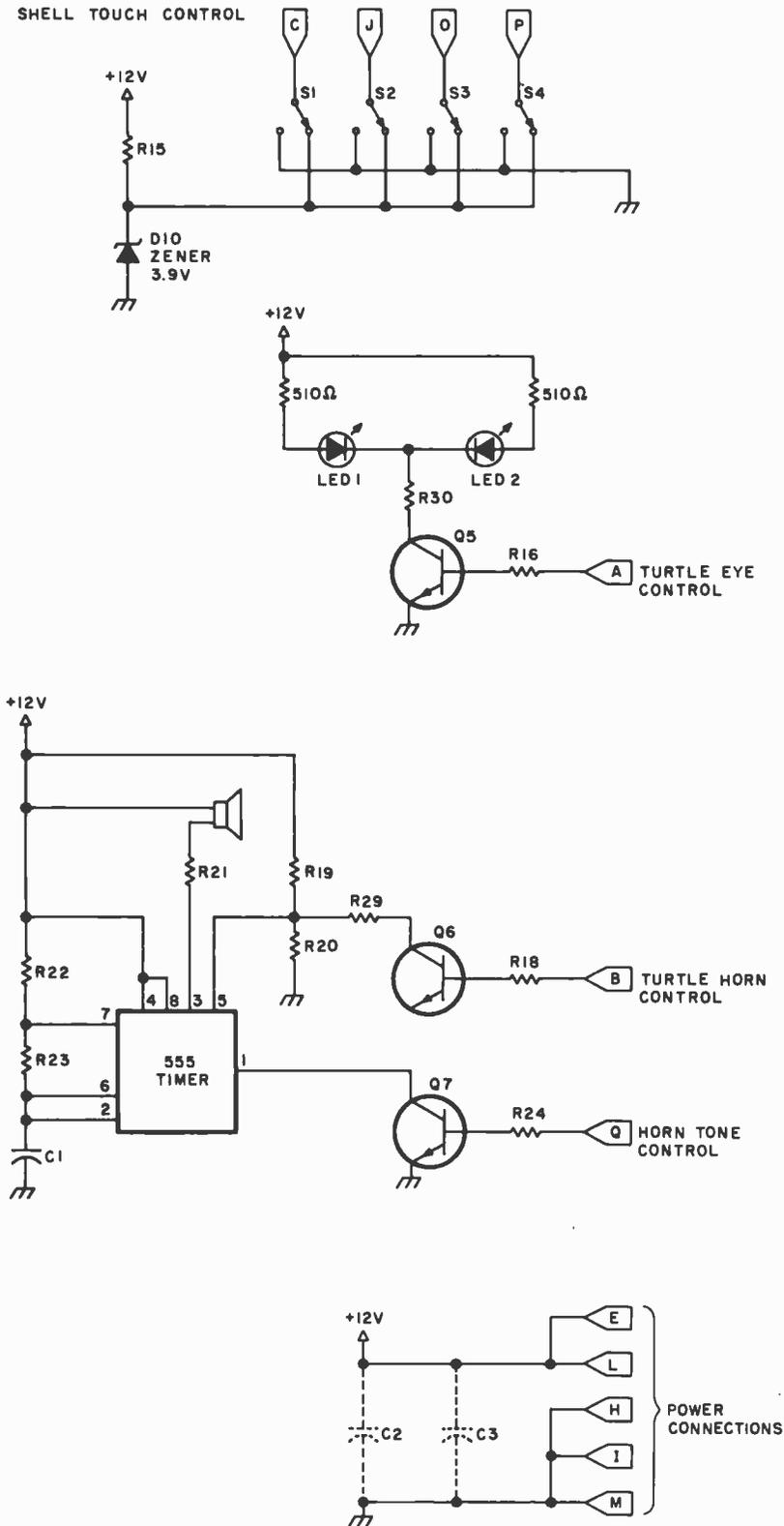
Figure 3: Schematic of the Turtle's touch sensor, lights, and horn control circuitry.
