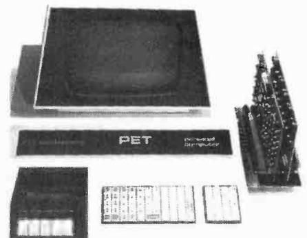
BETSI is the new Interface/Motherboard from Forethought Products—the makers of KIMST\*—which allows users of Commodore's PET Personal Computer to instantly work with the scores of memory and I/O boards developed for the S-100 (Imsai/Altair type) bus. BETSI is available from stock on a single 5 1/2" x 10" printed circuit card.
