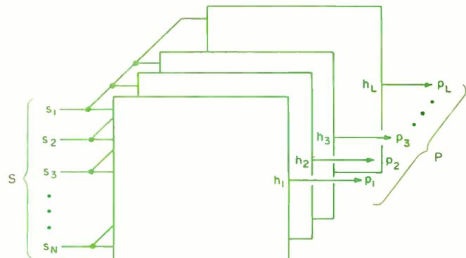
Figure 11: We will define the set of operators  $H = (h_1, h_2, \dots, h_L)$  as a function which maps the input vector  $S$  into the output vector  $P$ .
