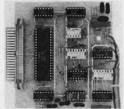
This board is RS-232 compatible and can be used with or without the expansion bus. There are on-board switch selectable data rates of 110, 150, 300, 600, 1200 and 2400 bps; parity odd, even, or null; 5 to 8 data bits and 1 or 2 stop bits. It has a data terminal ready line. The board alone sells for \$19.95 (with parts \$59.95). Assembled, it is \$79.95. Contact Electronic Systems, POB 21638, San Jose CA 95151.
