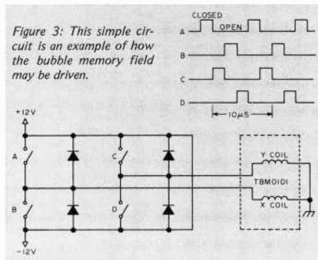
Figure 3: This simple circuit is an example of how the bubble memory field may be driven.
