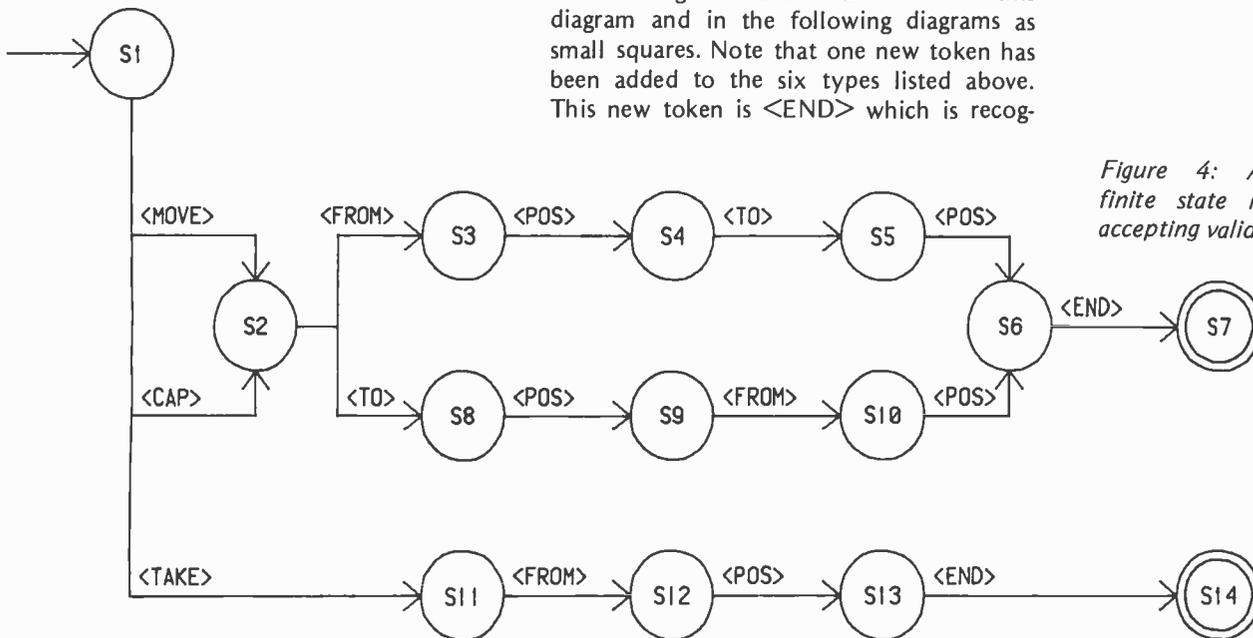
Figure 4: A syntactic finite state machine for accepting valid commands.
