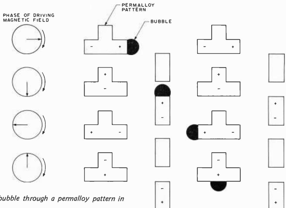
Figure 1: Movement of a magnetic bubble through a permalloy pattern in response to a rotating magnetic field.
