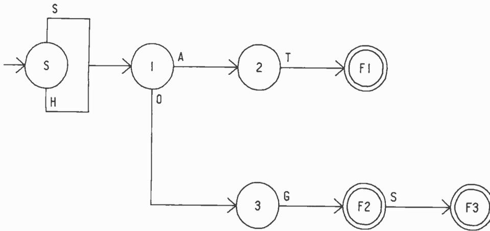
Figure 1: A finite state machine with one initial state and three final states that is capable of recognizing the words: sat, sog, sogs, hat, hog and hogs.
