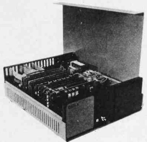
2, 8 K byte static programmable memory, 2 port parallel I/O (input/output) board, cable and two disk regulator board. For further information, contact Gimix Inc, 1337 W 37th Pl, Chicago IL 60609.
