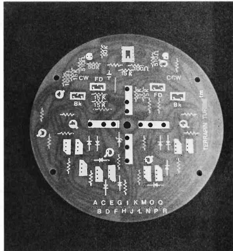
Photo 2: The foil side of the Turtle's printed circuit board.
