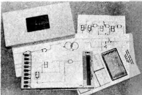
The Model 100 Broder Logic Trainer trains students without previous electronic background for digital electronic related assignments. It improves and grades the ability of the user. The Model 100 includes all gates, flip flops, positive and negative edge triggered devices, master-slave clocking, preset and clear functions. Switch circuit and Venn diagram problems as well as BCD and binary counting modes are included.
