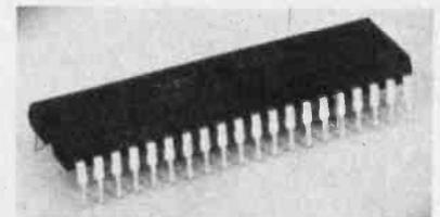
memory, while the  $\mu$ PD8035 is scheduled for applications using external program memory. The functional power of the units can be expanded using standard 8080A/8085A peripherals and memory products. The microprocessors are available in a standard 40 pin, plastic or ceramic dual-in-line package.
