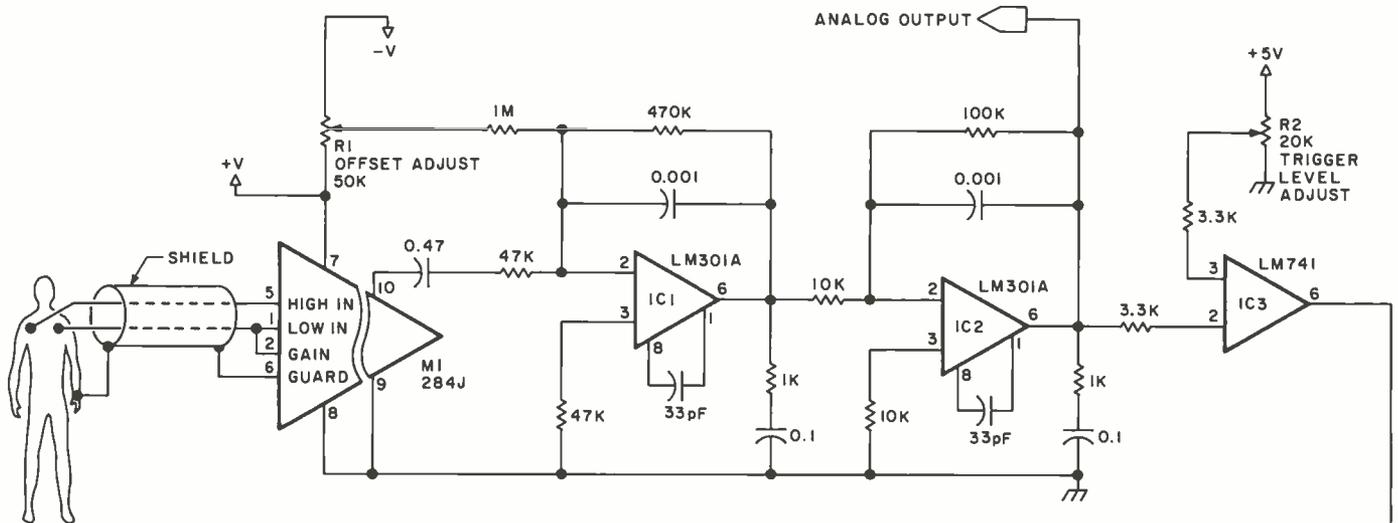
Figure 2: Schematic diagram of biofeedback monitor. IC4 is a type 284J isolation amplifier costing \$59 plus shipping from Analog Devices, Rte 1 Industrial Park, POB 280, Norwood MA 02062. +V is anywhere from 9 to 15 V and -V is from -9 to -15 V. All capacitors are 100 V ceramic unless otherwise noted. All circuitry should be mounted on a ground plane to reduce AC pickup. Connecting wires should be as short as possible. The electrode cable must be shielded to obtain proper operation.
