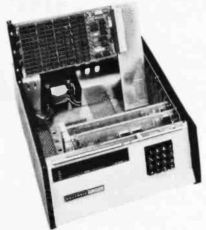
The H8 Extender Board allows Heathkit owners to troubleshoot their machine easily because each board is up above the computer for access to all circuits and components. Jumper links in power lines make power measurement simple. The links can be replaced with fine copper wire, which protects the traces or the motherboard from damage due to excessive current during testing.
