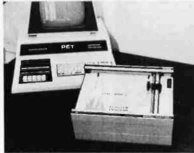
West Coast Consultants software provides users with full graphics capability for Houston Instrument's Hiplot plotter. Programs that drive the plotter through an RS-232 interface are currently available on tape cassette for the PET, Apple II, and TRS-80. The programs are written in BASIC and require a minimum of 16 K bytes of memory. For further information, contact West Coast Consultants, 1775 Lincoln Blvd, Tracy CA 95376. The prices are \$50 and \$75 for the programs.
