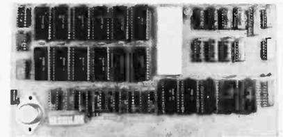
The DLX-10 is a single-board computer that executes BASIC directly in high-speed hardware from 5 to 10 times faster than 8080 systems or 2 to 5 times faster than Z80 systems. It does not replace the microprocessor but functions as a separate BASIC computer. It can boost an S-100 bus microcomputer system into the performance range of a minicomputer.
