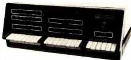
The new series II CPO Board features a 4 MHz Z-80A CPU and a full feature front panel. 20-slot actively terminated motherboard, with 25-amp power supply (50/60 HZ operation, incl. 68 cfm fan).
