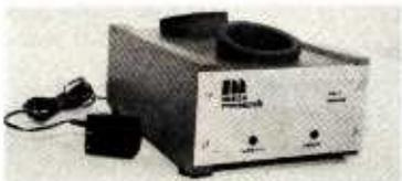
This acoustic modem uses a new type of crystal-lock circuitry. Even in kit form no calibration or adjustments are required.
