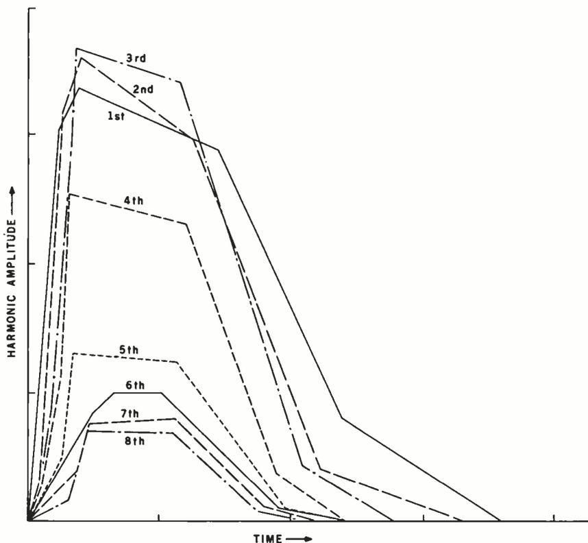
**Figure 7b:** Simplified analysis of a trumpet note. The complex curves seen in figure 7a have been divided into relatively long line segments to reduce the amount of information necessary to specify the sound to the computer. The graph here is based on Moorer's straight-line-segment simplification of his trumpet analysis; see reference 3.
