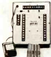
For the TRS-80 with Level II Basic • Provides 8 outputs • Provides 8 inputs • 2 ft. of interconnecting cable w/ connector • Plugs directly into TRS-80 • Power supply provided • Assembled and tested. Part No. VAR80, Introductory price \$109.95.
