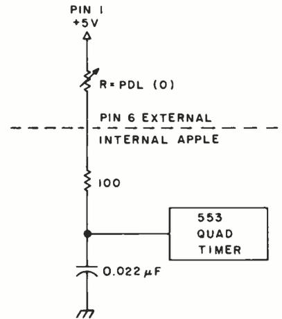
**Figure 1: A representation of the paddle-input system used by the Apple II computer.**
