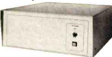
CMC Marketing Corp, 10611 Harwin Dr, Suite 406, Houston TX 77036, has announced the Model 2018 Microcomputer Mainframe System. The system consists of an eighteen-slot S-100 bus motherboard and cabinet; a constant voltage transformer that provides for input voltages of 120 or 230 VAC; and a
