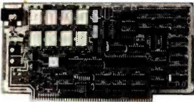
**88-MODEM S-100 ORIGINATE/ANSWER MODEM WITH AUTO-DIALER.** Software selectable baudrate provides any baudrate from 66-600 baud. Provides 1.5 stop bits when operated in 5-bit code mode. Auto-answer programs available for CROMEMCO CDOS, CP/M, North Star Horizon and MDS, and Alpha Micro.
