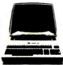
**ADM-42.** The semi-intelligent terminal that provides you with flexibility of format, security, editing, interface, and transmission. Two-page display standard (Optionally expandable to eight) • Blanking, blinking, and reverse fields • Three ways to TAB • 16 Function keys do the work of 32 • Detachable keyboard.
