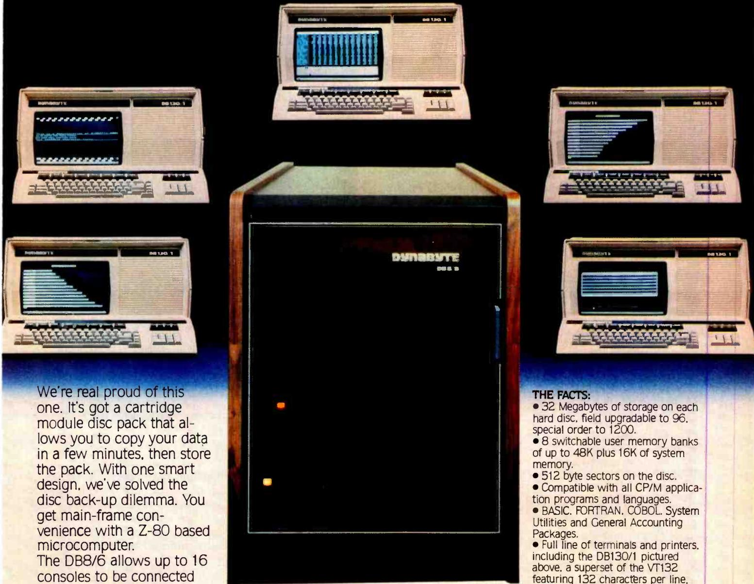
We're real proud of this one. It's got a cartridge module disc pack that allows you to copy your data in a few minutes, then store the pack. With one smart design, we've solved the disc back-up dilemma. You get main-frame convenience with a Z-80 based microcomputer.
