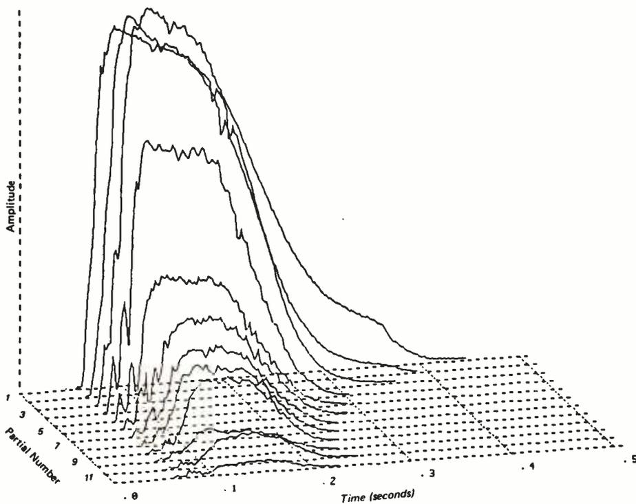
**Figure 7a:** Computer analysis of a tone produced by a trumpet. This is a two-dimensional projection of a three-dimensional plot. Amplitudes of different harmonics present in the note have different attack and decay characteristics. (Figure reproduced from the *Computer Music Journal*, volume 2, number 2, 1978, page 1; used by permission).
