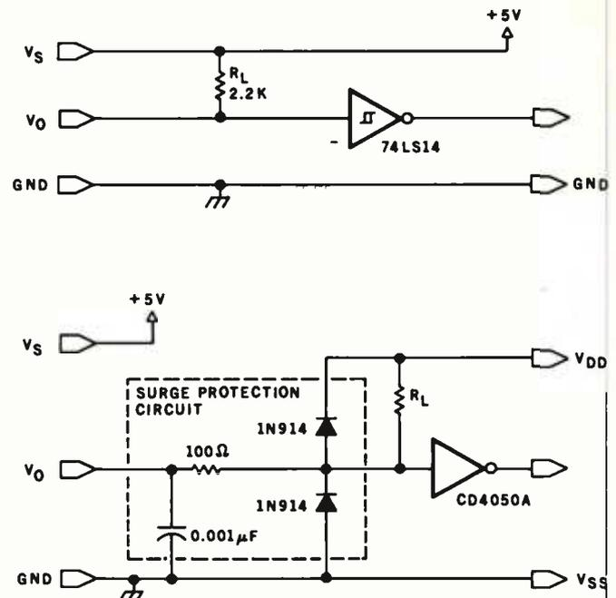
Figure 1: A pair of schematics showing (1a) the TTL interface for the HEDS-3000 bar-code reader, and (1b) the CMOS-logic interface. This diagram is reproduced from page 9 of the HEDS-3000 Digital Wand User's Manual, which accompanies the reader in a prototyping kit.
