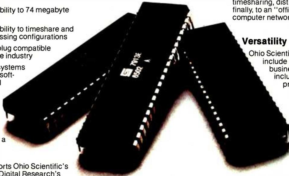
The GT option further extends Challenger III performance by utilizing the 6502C processor and high speed static RAM (150 ns. access) to achieve memory to accumulator ADD of 600 ns. and 1.2 MIPS average operation. This performance level places the C3 GT models comparable to mid-range minicomputers (\$50,000 to \$100,000 price range) in typical business and other information
