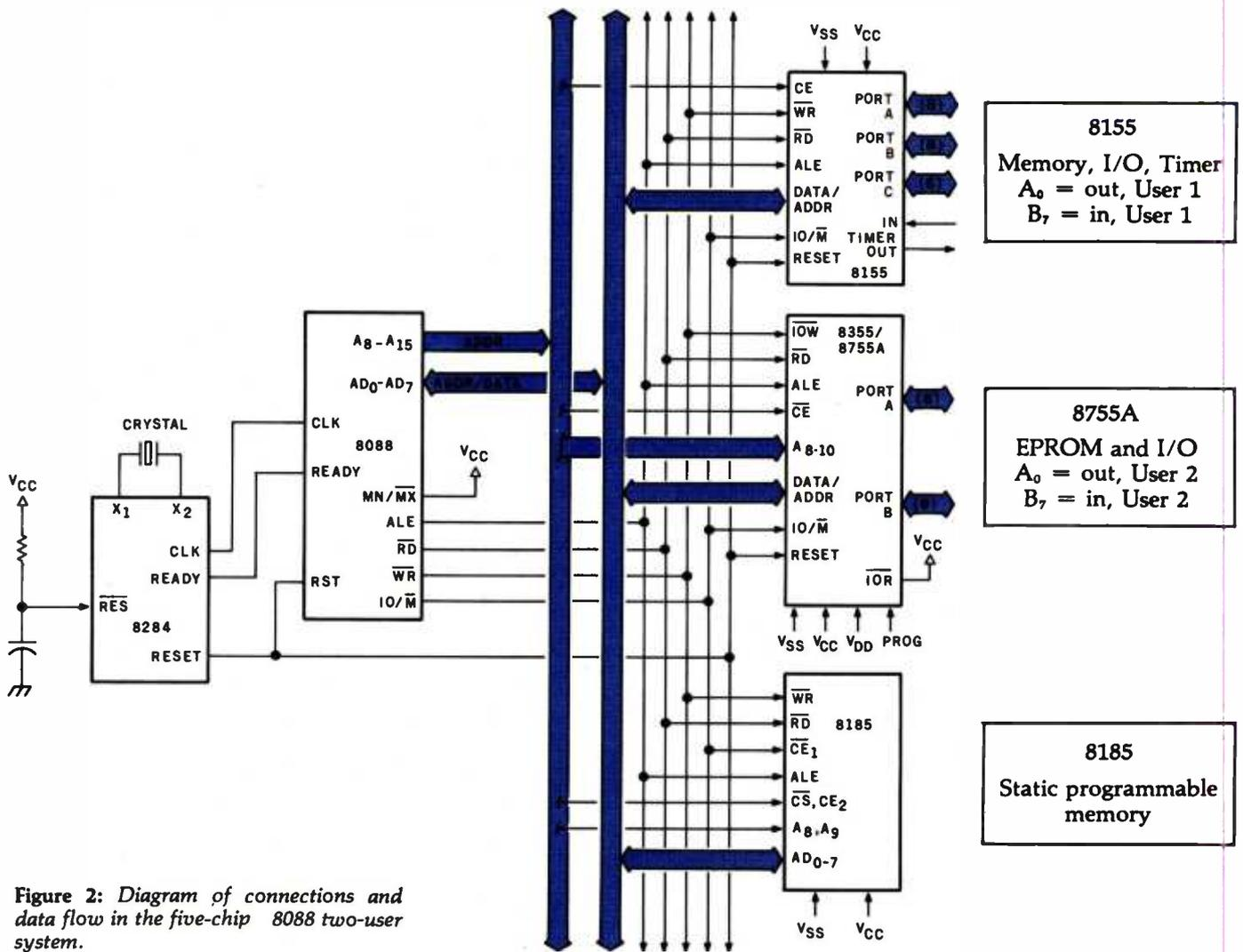
Figure 2: Diagram of connections and data flow in the five-chip 8088 two-user system.
