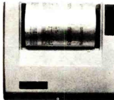
**Printing Characteristics:** 225 characters/second (170 lines/minute) throughput • 9 horizontal x 12 vertical matrix • 96 ASCII character set with upper and true lower case • 80 characters/line • 5.8 lines/inch
