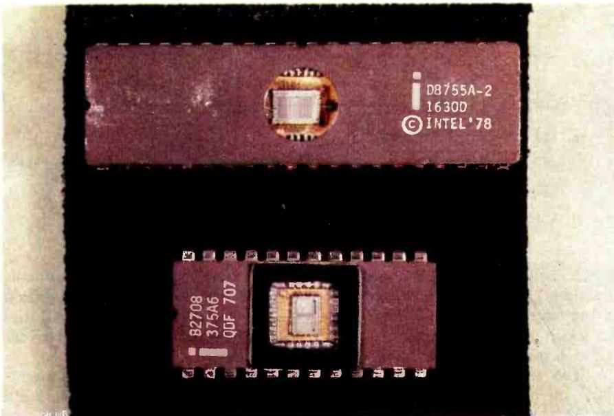
**Photo 2:** Side-by-side comparison of the 8755 EPROM, top, and the older 2708 EPROM. The difference in package size is due to the presence of I/O ports on the 8755. The 8755 requires a single 5-V power supply and contains 2 K bytes of memory; the 2708 requires three different power supply voltages (+5 V, +12 V, and -12 V) and contains 1 K bytes of EPROM.
