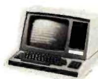
Two Z80 processors, mini-floppy drives, 25X80 display, 16K expandable to 48K!
