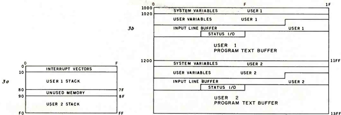
**Figure 3:** Map of memory use of the 8088 multi-user operating system. Programmable memory from hexadecimal addresses 00 thru FF is contained in the 8155 integrated circuit and is used chiefly to hold the pushdown stack for each user. Memory from hexadecimal locations 1000 thru 13FF is in the 8185 device, and stores various data belonging to the two user-tasks. Memory from hexadecimal addresses 0F800 to 0FFFF takes the form of EPROM in the 8755A, which stores the operating system.
