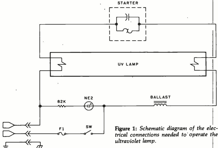
Figure 1: Schematic diagram of the electrical connections needed to operate the ultraviolet lamp.
