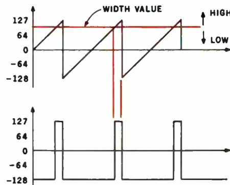
**Figure 3:** Derivation of a rectangular waveform. The value of samples from a sawtooth waveform are compared with some constant width value. If the sawtooth value is greater than or equal to the width value, the constant +127 is sent to the D/A converter. If the sawtooth value is less than the width value, the constant -128 is sent to the D/A converter.
