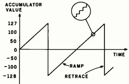
Figure 1: Generation of a sawtooth waveform by software. Coordinate points along the waveform are generated by continuously adding a constant value, *FREQ*, to the accumulator (register A). The point values (samples) are sent to the D/A converter. A close-up circle demonstrates the inevitable stair-step quality of the curve reproduced from discrete samples. The 6502 assembler code to produce the sawtooth is shown in listing 1.
