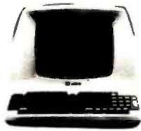
**ADM-31.** A terminal that's too smart to be considered dumb. Comes complete with keyboard, control logic, character generator, refresh memory & interface • Displays two pages of text instead of one • Field protect mode • Factory installed selected parameters. Reg. Price. \$1,450 ..... **Sale! \$1,195**
