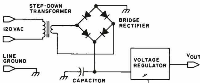
Figure 1: Schematic diagram of a typical power supply circuit containing a step-down transformer, a full-wave bridge rectifier, a filter capacitor, and an integrated circuit voltage regulator.
