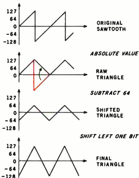
**Figure 2:** Method for transforming samples of a sawtooth waveform into samples of a triangular waveform. First the absolute value of the contents of the accumulator is determined. A constant value, 64, is subtracted from the accumulator. The remaining value is multiplied by 2; the multiplication is performed by the simple method of shifting the binary value one bit to the left.
