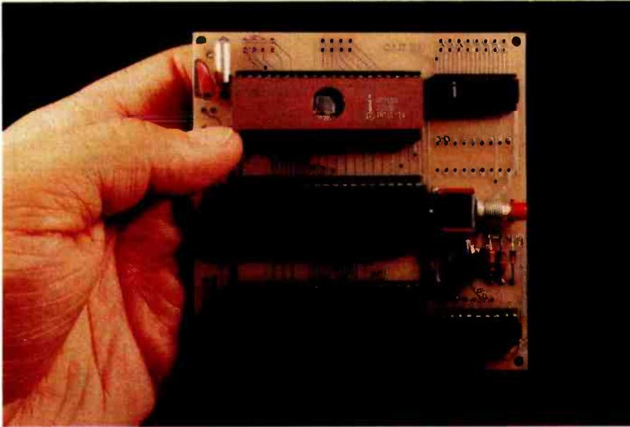
**Photo 1:** This 8088 system fits in the palm of your hand and uses only five integrated circuits. It contains enough read-only and programmable memory, and sufficient peripheral interfaces, to support two 300 bps terminals, running a Tiny BASIC interpreter on each.
