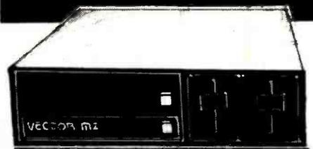
System B is a Z-80 based microcomputer with over 630,000 characters of on-line storage and is capable of handling standard accounting or special computations of any small business or large company department — even scientific calculations in a technical environment. Call for Our Price
