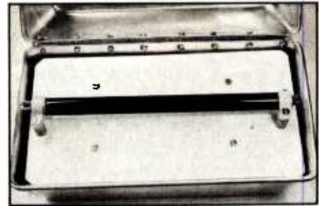
Photo 3: The ultraviolet lamp tube is supported on its aluminum baseplate by insulating standoffs and cable ties.
