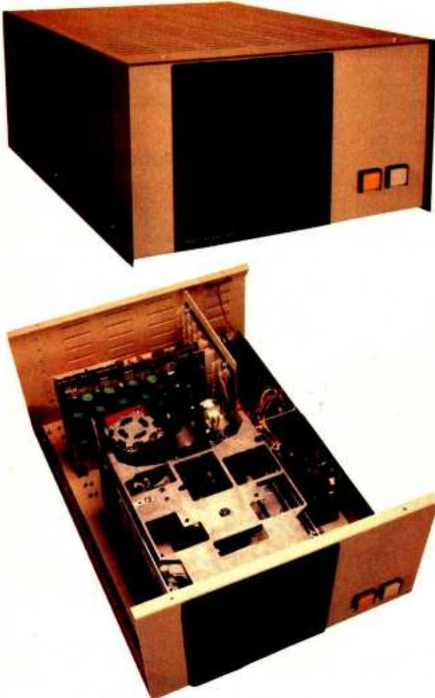
The C2-OEM with cover off showing the placement of floppy drives, UL recognized power supplies and 8-slot OSI BUS backplane.
