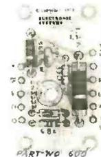
This board has two active circuits, one converts RS-232 to 20 mA, the other converts 20 mA to RS-232. Requires +12 and -12 volts. \$9.95 Part No. 600A Kit.
