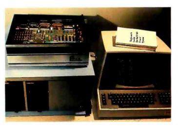
1: The Pascal Microengine is shown here in a system cludes two Shugart 8-inch disk drives in an Integrand cabinet 3000 CIQ120 terminal. The computer uses a 16-bit processor chip and it executes p-code directly through the use of three integrated circuits on which the processor microinstruction e stored. The Microengine also includes 64 K bytes of men a 24-bit parallel port, and two RS-232C serial interfaces. The store provided is the UCSD extended Pascal system.
