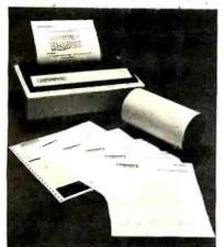
The model 737 dot-matrix printer features right-margin justification, proportional spacing, forward and reverse paper motion, and three-way paper handling. It prints 7-by-8 dot-matrix characters at 10 and 16.5 characters per inch for standard data processing tasks, and generates n-by-9 dot-matrix characters in the proportional character spacing used for data and text processing. The printer incorporates an adjustable nine-wire, free-flight printhead. Under manual or software control, the
