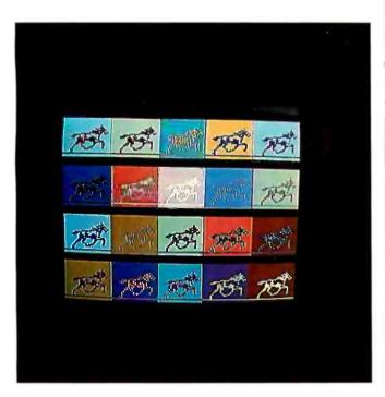
**Photo 2:** An example of the Apple III's high-resolution color graphics (290 by 192 lines of resolution with sixteen colors) displayed on an RGB (red, green, blue) color monitor. This particular demonstration is an animation program: the horses gallop on the screen.
