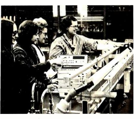
Photo 2: Forensic physics students taking data with a multimemory digital timer and an air track.
