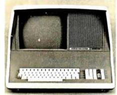
12" Display; 24 x 80 format; 18-key numeric keypad; 128 upper/lower case ASCII characters; Reverse video, blinking; Complete cursor addressing and control; Special userdefined control function keys; Protected and unprotected fields; Line insert/delete and character insert/delete editing; Eleven special line drawing symbols.
