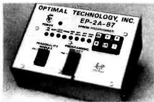
The Model EP-2A-87 EPROM Programmer has an RS-232 compatible interface and includes a 2K or 4K buffer. During the ON-LINE mode, another computer can down-load to the buffer. Only two easy-to-implement commands are available to an external computer. (Load
