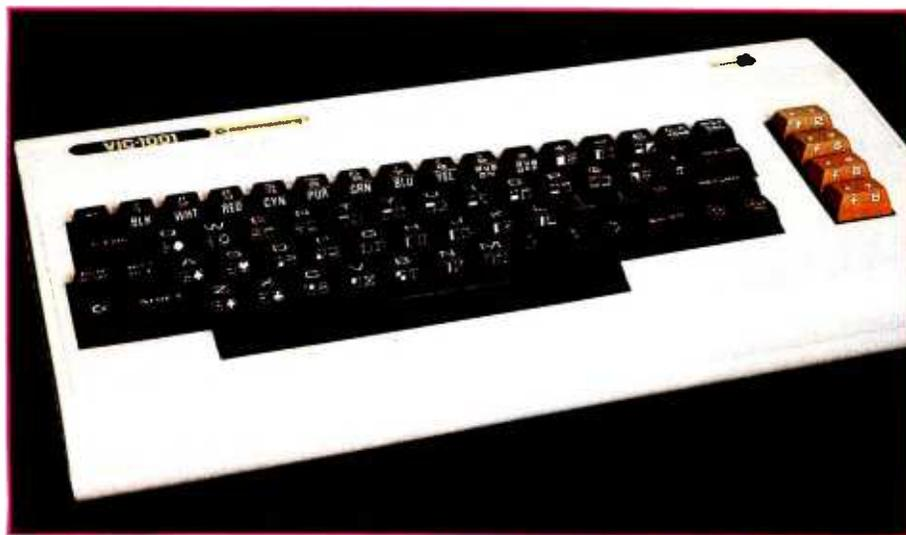
Photo 1: The Commodore VIC 20 microcomputer. This unit, a final prototype based on the Japanese version of the VIC microcomputer, differs from the American model only in the model number.
