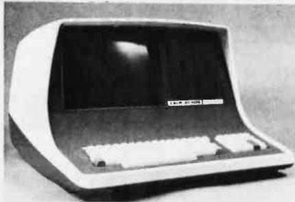
64K Double or Quad Density units available. Uses two Z-80 CPU's. Commercial-type terminal with 12" monitor. Dual double density minifloppies. Over 350 kilobytes of storage (twice that with quad density drives). Two serial RS232 ports, I/O ports standard. Expandable with optional S-100 S-100 interface. Comes with CP/MTM 2.2 operating system. MiniMicroMart can supply a wide range of CP/M development and application software.
