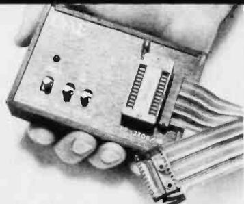
OAE's PP-Series EPROM Programmers plug directly into any vacant EPROM socket and allow you to transfer data directly from RAM to EPROMs. No additional power supplies are required. All timing & control sequences are handled by the programmer. Each unit includes internal DC to DC switching regulator, ZIF socket and 4 ft. ribbon cable terminated with a 24 pin plug. Programmers are available for all EPROMs from 2708's thru 2532's.
