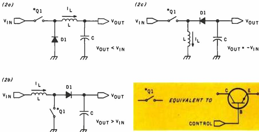
Figure 2: The configurations of switching voltage regulators: the voltage-step-down (2a), voltage-step-up (2b), and polarity-inverting (2c) arrangements are depicted. The component shown as a switch is assumed to be a bipolar transistor driven in saturated switching mode. Some commercial designs may use field-effect transistors.
