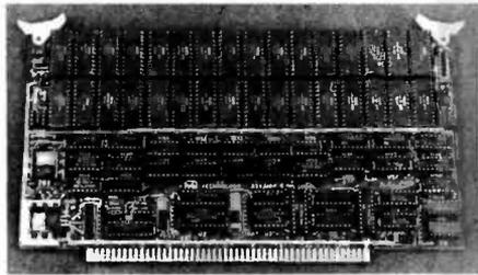
The 32K x 8 bit/16K x 16 bit STATIC RAM BOARD uses low power and its fast device access time of 200 nsec (max.) allows for operation @ 4 MHz without any wait cycles.
