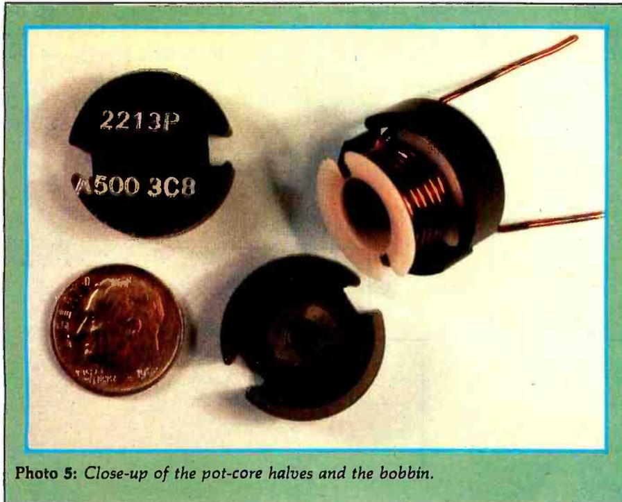
Photo 5: Close-up of the pot-core halves and the bobbin.
