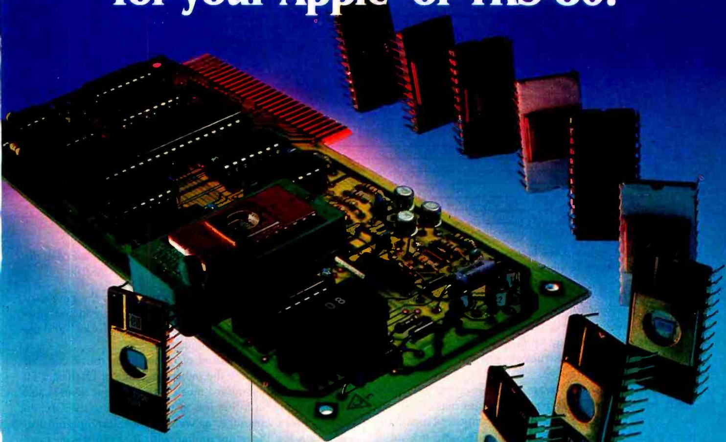
Apparat announces the most versatile EPROM burner available today for your TRS-80 model I and III or Apple computer . . . the Apparatus PROM Blasting system (A.P.B.). Most EPROM burners will program only one type of EPROM. The A.P.B. system will program all commonly used 24 pin EPROMs by using special personality modules that adapt the unit to the EPROM. The following EPROMs are programmable: 2704, 2708, 2716, (3-volt) & (5-volt), 2732, 2508, 2516 and 2532.
