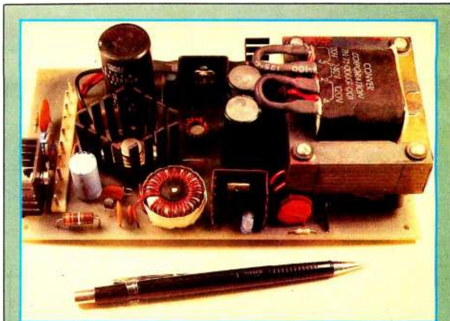
**Photo 2:** A commercially sold switching power supply that combines both linear-regulator and switching-regulator technology to provide outputs of  $\pm 12$  volts and  $+5$  volts. Note the use of the toroidal inductor and the relatively small heat sinks. This unit was made by Conver Corporation, 10631 Bandlely Dr, Cupertino CA 95014. (408) 255-0151.
