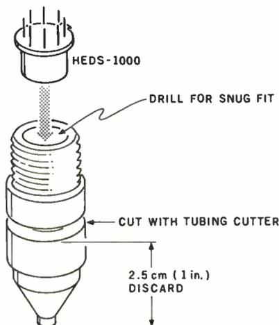
Figure 2: Modifications made to Schaefer No Nonsense pen barrel. With contents removed, the pen becomes a home for the HEDS-1000 sensor. The cable and indicator LED are affixed to the pen barrel (2a), while the sensor is mounted to the pen tip (2b).
