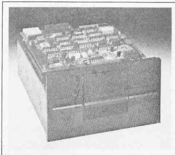
sity: 48 TPI • Cylinders: 35 or 40 • Tracks: 70 or 80 • Recording Method: FM or MFM • Rotational Speed: 300 RPM • Transfer Rate: 250K bits/second • Latency (avg.): 100 ms • Access Time: Track-to-track 12 ms; Settling 15 ms • Head Load Time: 50 ms
