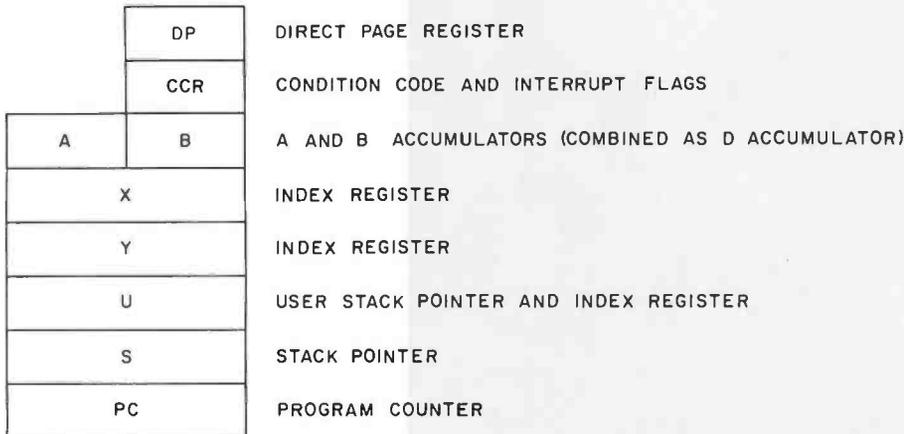
**Figure 1:** Register model of the Motorola MC6809 microprocessor. In addition to its program counter (PC) and stack pointer (S), the MC6809 has four user-programmable 16-bit registers: X, Y, U, and D. (D is equivalent to a concatenation of registers A and B.)
