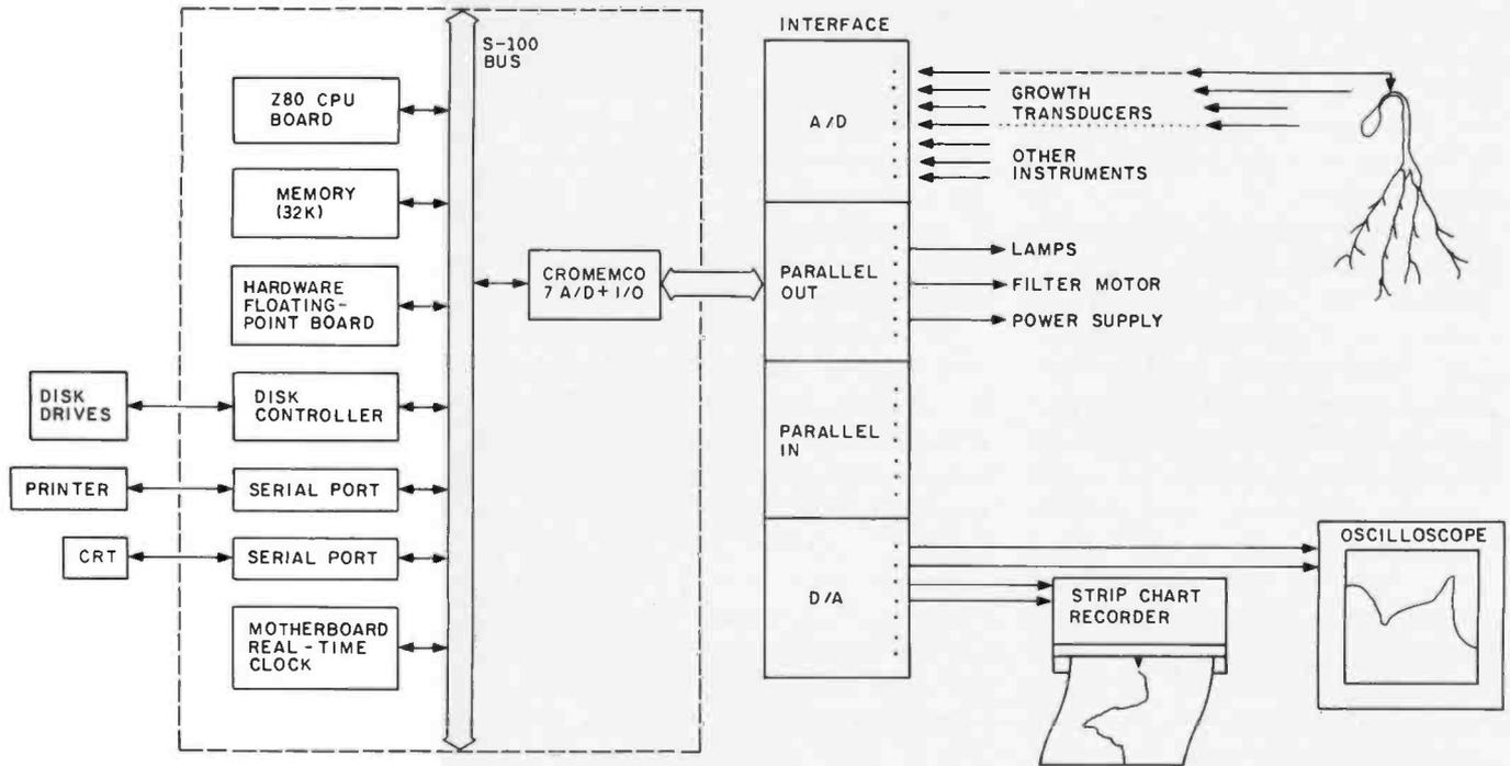
Figure 2: Block diagram of the hardware and peripherals used in the author's data-acquisition system.
