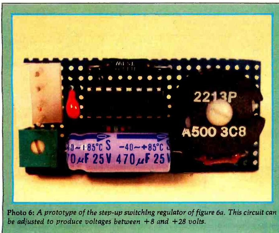
Photo 6: A prototype of the step-up switching regulator of figure 6a. This circuit can be adjusted to produce voltages between +8 and +28 volts.
