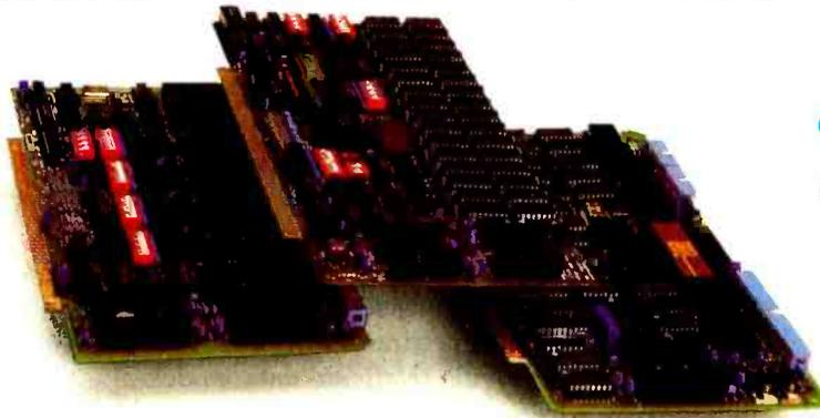
**DOUBLE DENSITY FLOPPY DISK CONTROLLER BOARD** — controls up to four 5¼-inch or 8-inch disk drives using IBM soft sectored formats. It features 1K of on-board buffering, DMA controlled data transfers and the performance characteristics of the superior NEC 765 chip.
