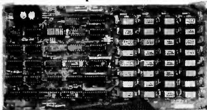
SD Systems has duplicated the famous reliability of their ExpandoRAM I and II boards in the new ExpandoRAM III, a board capable of containing 256K of high speed RAM. Utilizing the new 64K x 1 dynamic RAM chips, you can configure a memory of 64K, 128K, 192K, or 256K, all on one S-100 board. Memory address decoding is done by a programmed bipolar ROM so that the memory map may be dip-switch configured to work with either COSMOS/MPM-type systems or with OASIS-type systems.
