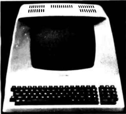
Upper and lower case, 15 baud rates: 75 to 19,000 baud, dual intensity, 24 x 80 character display, 12 x 10 resolution. Numeric pad. Programmable reversible video, auxiliary port, self-test mode, protect mode, block mode, tabbing, addressable cursor. Microprocessor controlled, programmable underline, line and character insert/delete. "C" version features typewriter-style keyboard. List \$925 **\$739**
