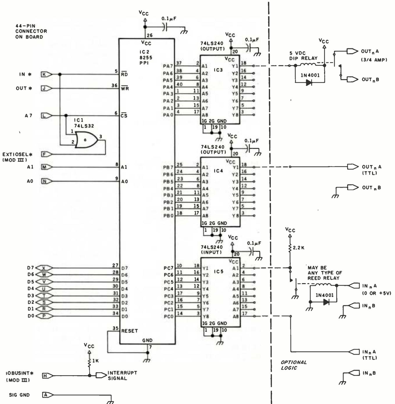
Figure 5: The GPIO board for the Model I and III uses an Intel 8255 Programmable Peripheral Interface chip as a 24-line controller. Sixteen of the lines are outputs and control 74LS240 drivers. Eight of the lines are inputs.
