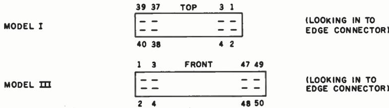
Figure 8: Cable wire list and edge connector orientation.
