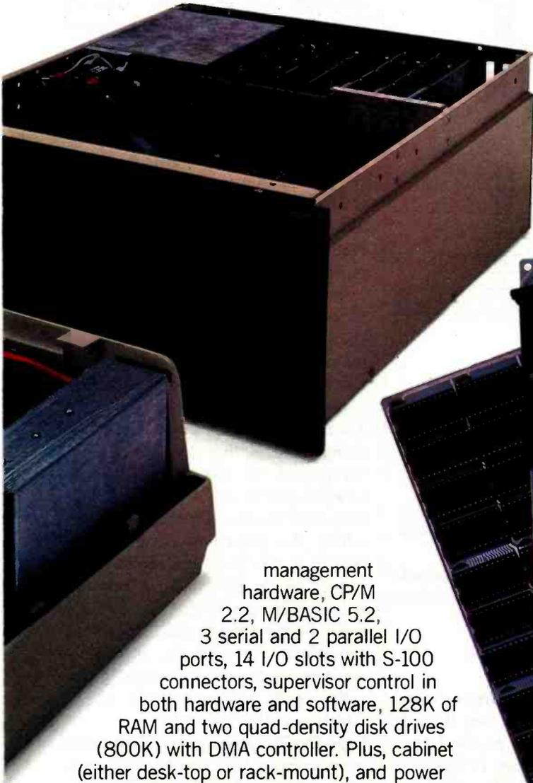
management hardware, CP/M 2.2, M/BASIC 5.2, 3 serial and 2 parallel I/O ports, 14 I/O slots with S-100 connectors, supervisor control in both hardware and software, 128K of RAM and two quad-density disk drives (800K) with DMA controller. Plus, cabinet (either desk-top or rack-mount), and power supply. The same system with 8" floppies and a full Megabyte of formatted storage costs \$5,659. And, we offer OEM pricing.
