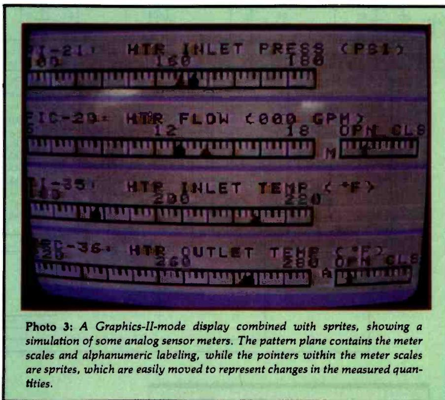
Photo 3: A Graphics-II-mode display combined with sprites, showing a simulation of some analog sensor meters. The pattern plane contains the meter scales and alphanumeric labeling, while the pointers within the meter scales are sprites, which are easily moved to represent changes in the measured quantities.
