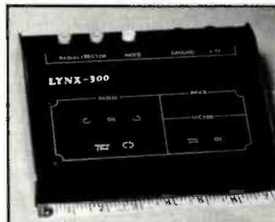
justments and to indicate if the adjustment is not within specifications. The Lynx-300 is powered directly from the drive.
