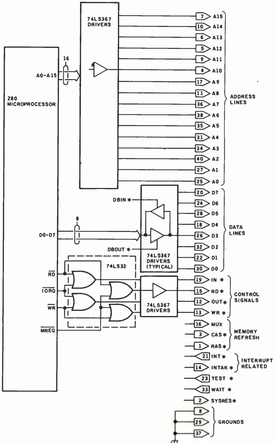
Figure 1: The system bus for the Model I is made up of 40 lines, very closely related to Z80 signals. Sixteen are address lines, eight are data bus lines, four are control signals for external devices, and the remainder are related to memory refresh, interrupt operations, and miscellaneous functions.
