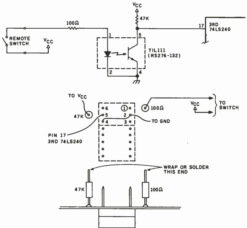
Figure 13: Sample optoisolator application for the GPIO. A remote switch lights the LED contained within the optoisolator. This turns on the phototransistor, bringing the collector to a 0 level.
