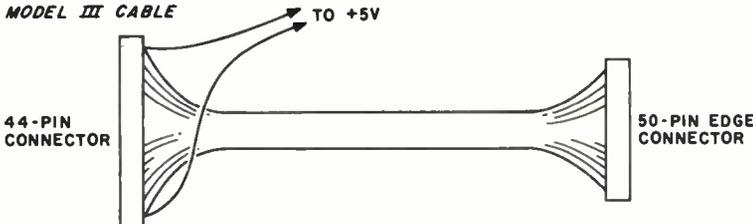
Figure 9: The cable for the Model I is different from the Model III version. The Model I version uses a 40-pin edge connector, while the Model III version uses a 50-pin edge connector. Both versions use a 44-pin connector for the prototype board.
