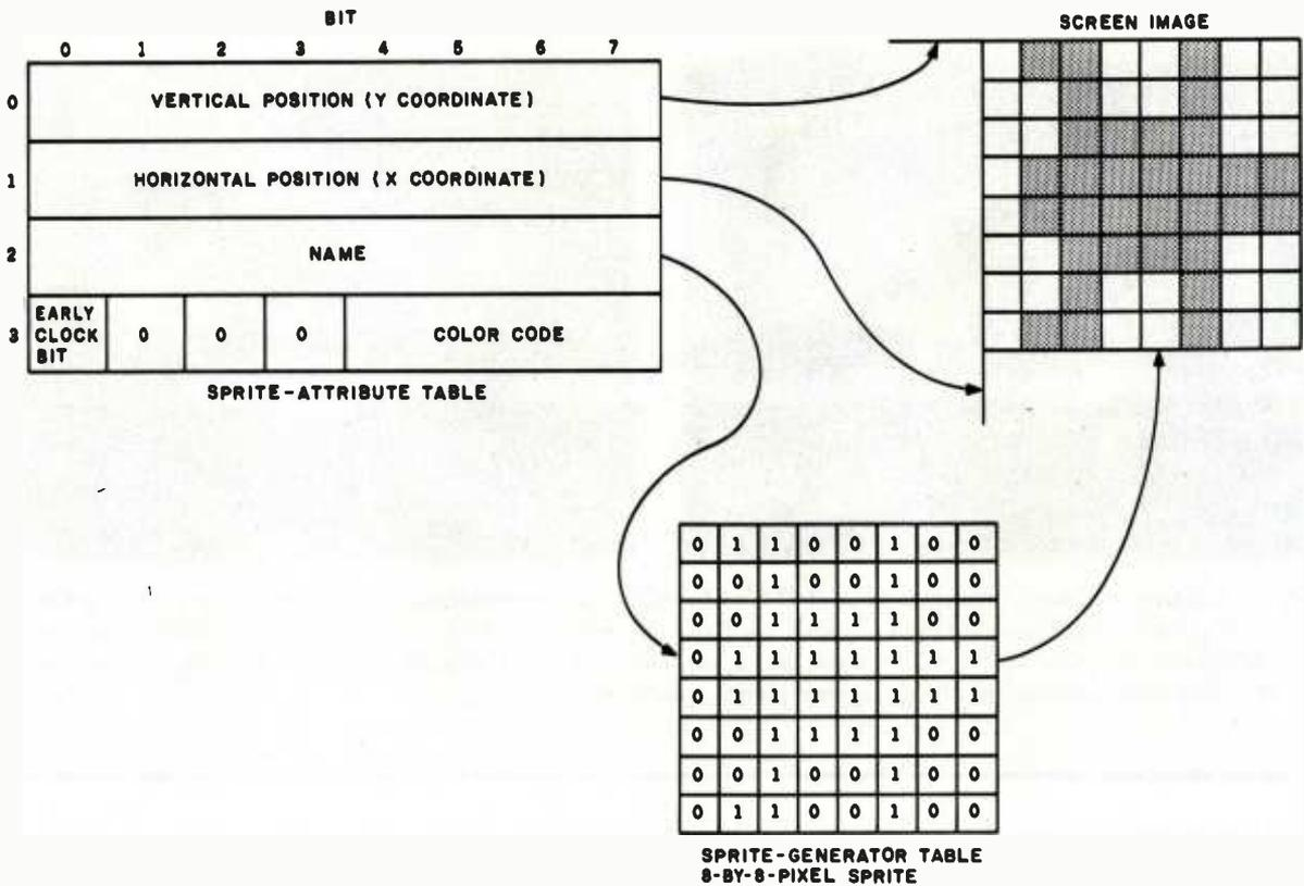
**Figure 3:** The binary coding for an 8-by-8-pixel sprite pattern is stored in VRAM in the sprite-generator table in 8 bytes. Each bit in the pattern coding corresponds to one pixel in the displayed pattern. Wherever a 1 is stored in a pixel's pattern bit, the sprite will be colored; where the bit is a 0, the sprite will be transparent. Each sprite can be only a single color.
