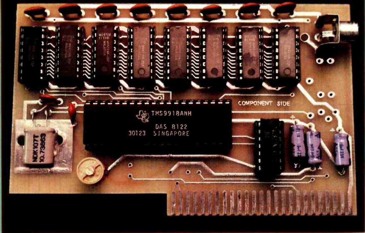
Photo 4: The Circuit Cellar E-Z Color Graphics Interface; a prototype printed-circuit board is shown. This typical TMS9918A color graphics interface is interfaced to the Apple II microcomputer bus with a minimum of components.
