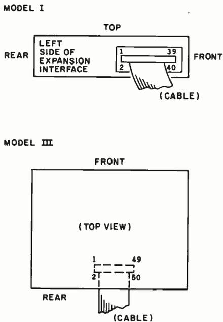
**Figure 10:** Cable connection to the Model I or III.
