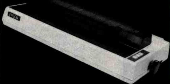
80 CPS, Bi-directional logic seeking 9x9 dot matrix, full 96 ASCII char. Set with true descenders, centronics-style parallel port (RS232 optional), 136 col., includes grafrax plus dot addressable graphics, friction feed and removable tractor feed. 21 lbs., 110 volt only.
