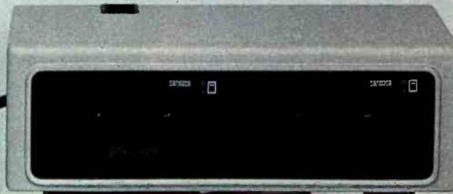
Digital's introduced a personal computing option which can turn a VT100 terminal into a personal computer that uses the CP/M® operating system.
