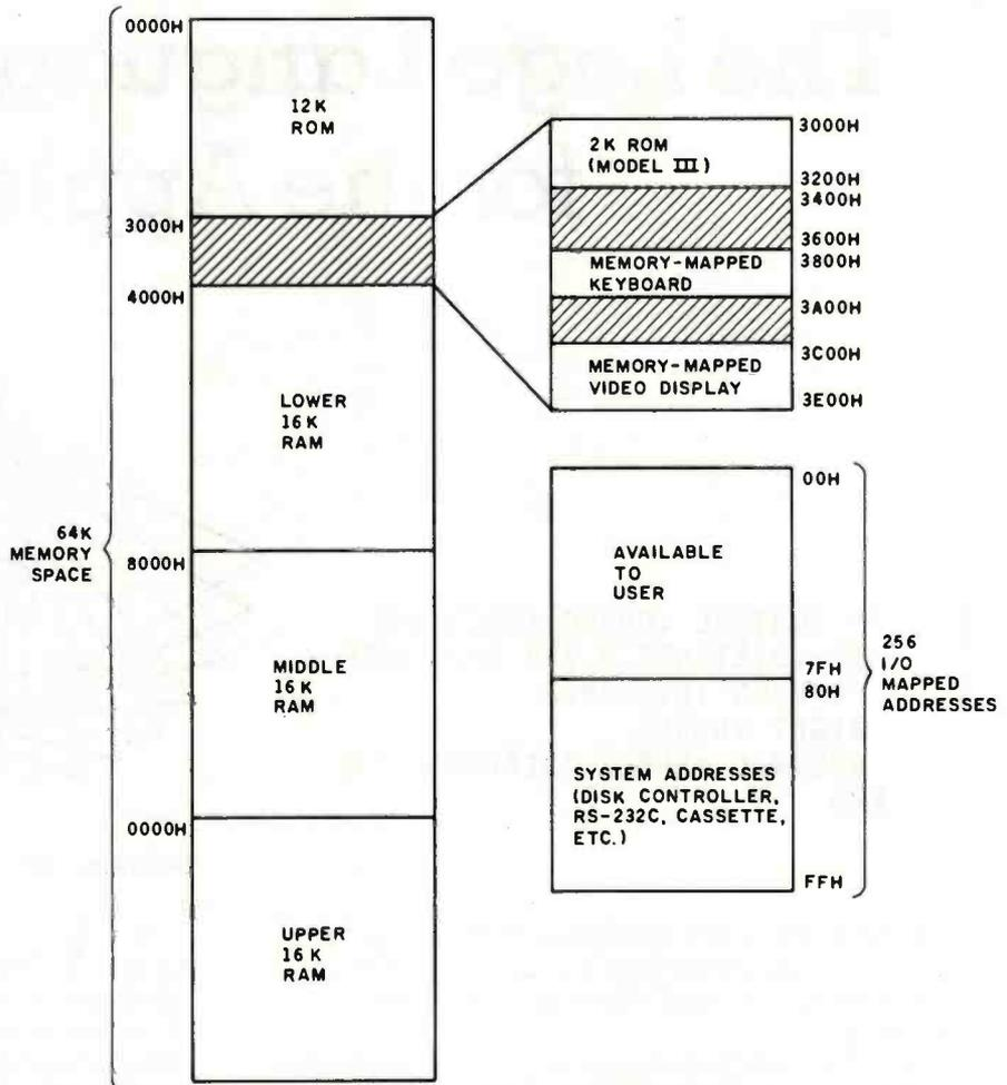
Figure 2: The Models I and III have 64K bytes of addressing space. Some system devices are memory-mapped and use dedicated addresses within the 64K bytes. Other system devices use the I/O-mapped addresses hexadecimal 0 through FF.
