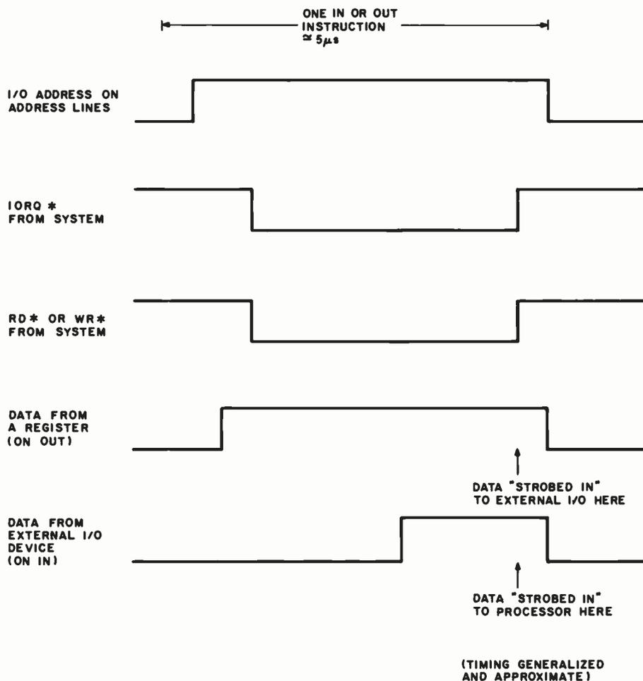
**Figure 4:** External I/O operations use an I/O address on the address bus, the IORQ\* signal, and the RD\* or WR\* signal to effect 8-bit data transfers to and from the external I/O device.
