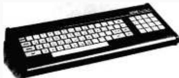
Reliable, portable RCA VP 3000 series Interactive Data Terminals feature: video and audio output; color-locking circuitry for sharp color graphics and rainbow-free characters; reverse video; tone and noise generator; 20 and 40 character formats; resident and programmable character set; LSI video and microprocessor control. All have a unitized 58-key, 128 character keyboard with flexible membrane switches, plus the features of the ASCII keyboards below.
