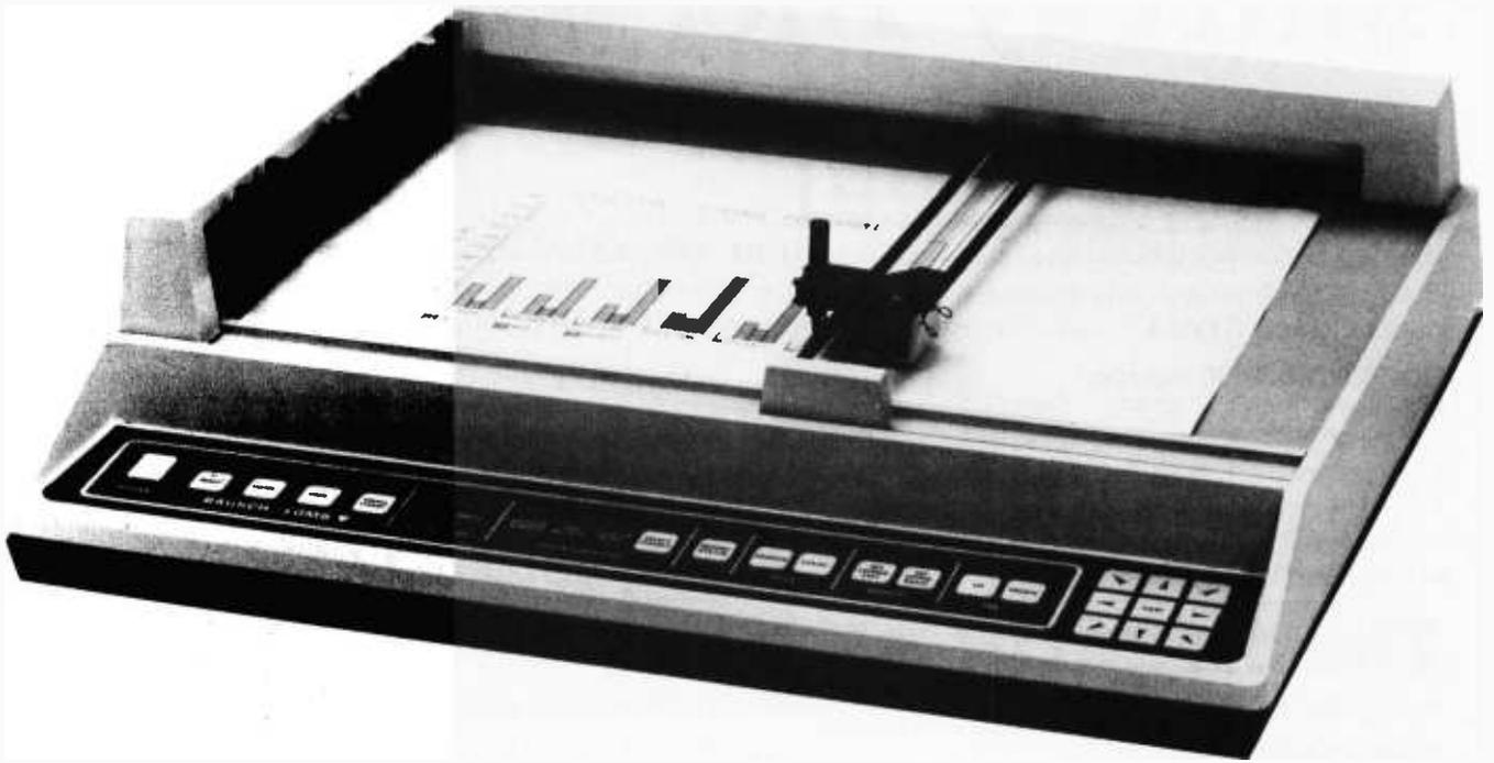
Photo 1: A flatbed plotter; shown here is the Houston Instrument DMP-29. (Photo courtesy of Bausch and Lomb; see vendor text box for address.)
