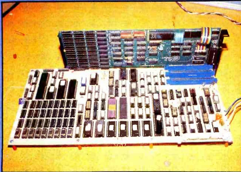
**Photo 3:** Prototype of the MPX-16 being tested for compatibility with the I/O-expansion bus of the IBM Personal Computer. A Quadram Quadboard (an expansion card for the IBM PC that contains 256K bytes of memory, a serial port, a parallel port, and a real-time clock) is inserted in one of the MPX-16's slots. It works!
