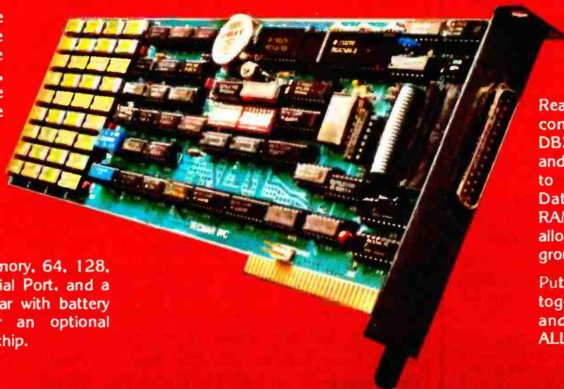
Ready to use, ALL IN ONE™ comes complete with the DB25 connectors on Serial and Parallel Ports, Software to set system Time and Date, and the popular RAMSPOOLER™ utility to allow printing as a background task.
