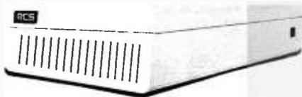
The 192k RAM, 2 asynchronous serial ports, 3 parallel ports, and a Real Time Clock are all built on to the motherboard, so you won't have to waste precious slots on them.
