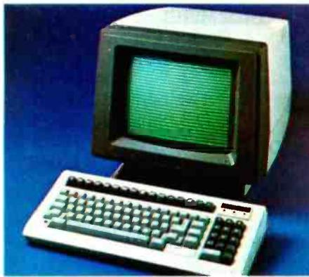
**VIDEO DISPLAY TERMINAL FROM SHINLEE CORP** --- Shinlee's T88 terminals is microprocessor-based, teletype-compatible model with detachable keyboard capable of displaying the complete ASCII set. The 12-inch screen will accommodate 2,000 characters in an 80 x 25 matrix. The T88 is compatible with most currently-available terminals. Size:
