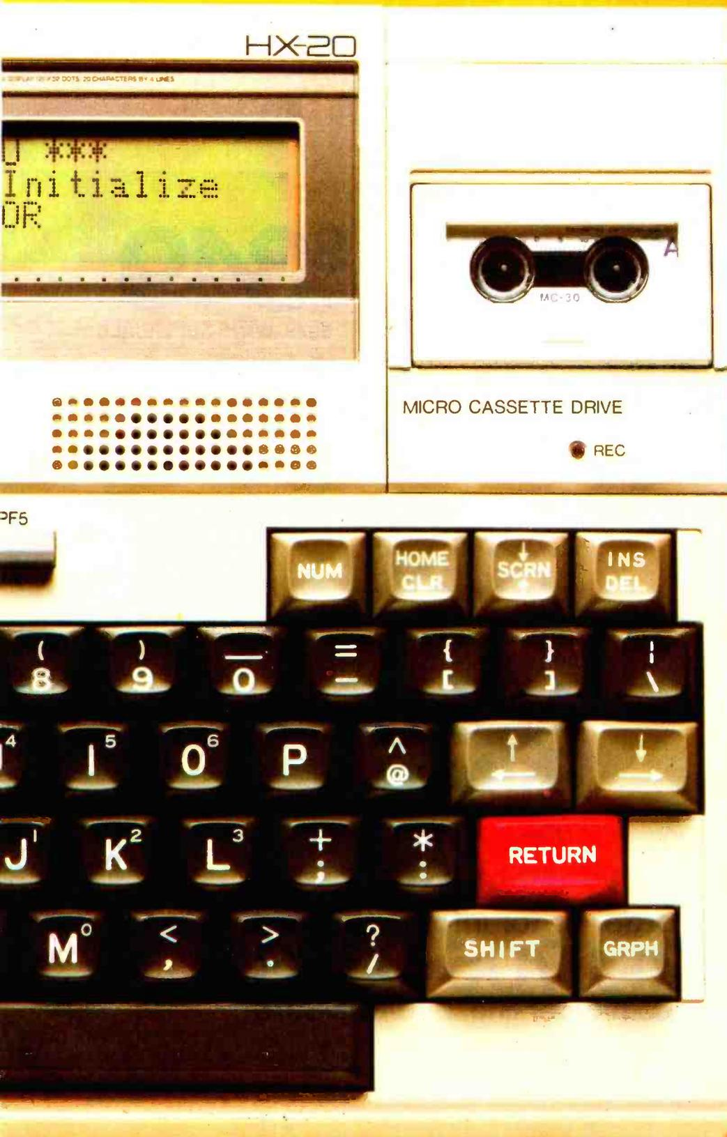
So with the HX-20, you can do programming, word processing and data entry just like you've got a big screen, up to 255 characters wide, with easy-to-read upper and lower case letters, numbers and punctuation and any 20 column by four line part of it visible by user command.
