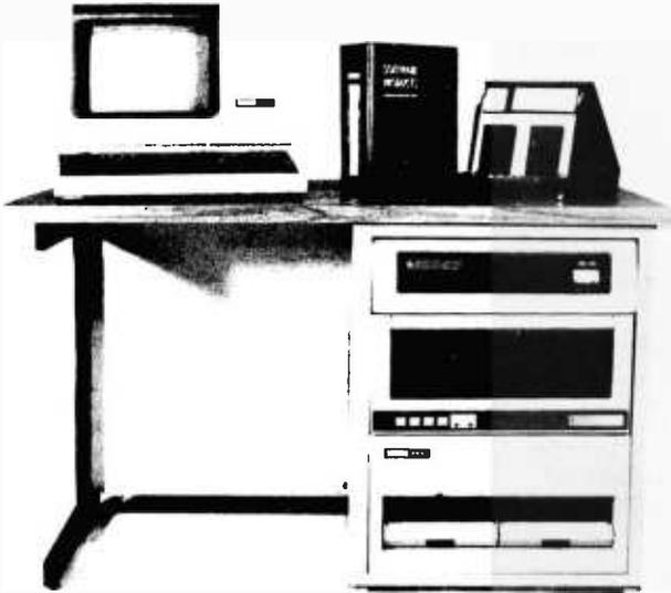
**CI-MWS03-SB** — LSI 11/2 computer workstation. LSI 11/2 CPU, 64KB Memory, power supply, KEV 11, in 16 slot rack mountable chassis. 2 port serial I/O. CRT terminal. 1 mega byte floppy disk system. Desktop workstation ..... **\$7,295.00**
