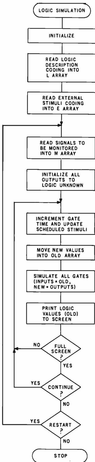
Figure 2: Flowchart of the Logic Simulator program. The simplicity of this diagram should lend encouragement to those interested in simulating digital logic circuitry. The implementation of this program in a high-level language (see listing 1) can be quite short.
