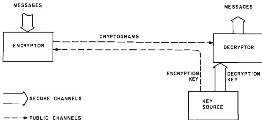
Figure 2: A public key cryptographic system. Encryption keys can be safely sent over the ordinary communication channel because the information they contain cannot be used to decrypt messages. Decryption keys are created near the decryptor and are not sent anywhere else. Each person who expects to receive encrypted messages creates a key for encryption and a corresponding key for decryption and sends the encryption key to those who will originate the messages.
