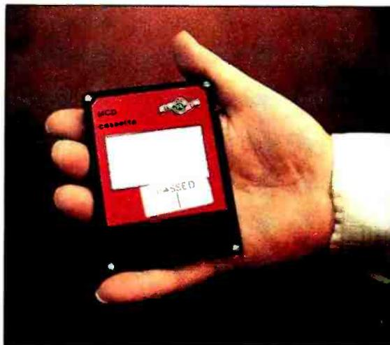
Here's a 3-inch disk pack for the Grundy Newbrain AD computer. The Newbrain disk-drive module houses two 3-inch disk drives in a small unit the size of the computer itself—in fact, the disk-drive module is meant to fit unobtrusively under the computer.
