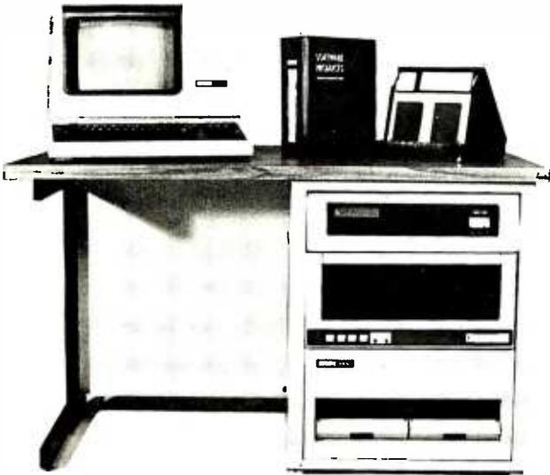
**CI-MWS03-SB** — LSI 11/2 computer workstation. LSI 11/2 CPU, 64KB Memory, power supply, KEV 11, in 16 slot rack mountable chassis. 2 port serial I/O. CRT terminal. 1 mega byte floppy disk system. Desktop workstation ..... **\$7,295.00**
