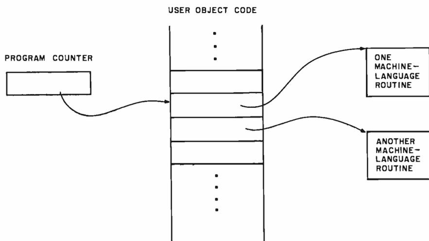
Figure 1: Simple threaded object code. The program counter points to certain object code, which in turn points to a machine-language routine. When that routine is finished, the program counter is incremented and points to the next object code, which points to the next machine-language routine.
