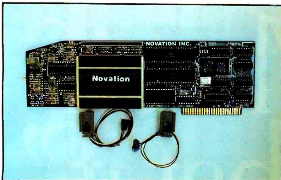
**Photo 1:** The Apple-Cat II basic system circuit board with the telephone connector cables. The cables are connected to pins located along the top of the card. Also shown are the two empty sockets for chips. The one on the left is for the Touch-Tone receiver chip; the other one (near the upper right corner) is for firmware ROM chips. (All photos are by the author.)
