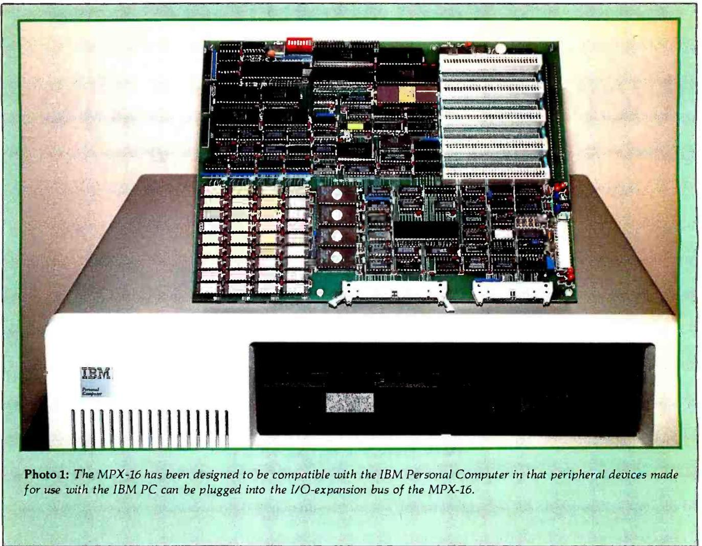
**Photo 1:** The MPX-16 has been designed to be compatible with the IBM Personal Computer in that peripheral devices made for use with the IBM PC can be plugged into the I/O-expansion bus of the MPX-16.
