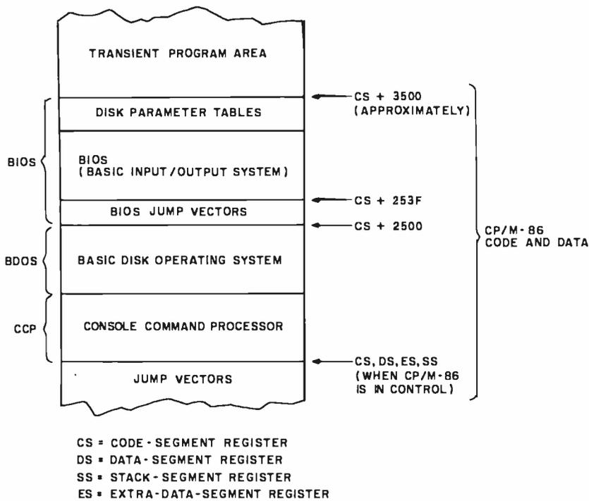
**Figure 3:** Memory map of the CP/M-86 operating system as configured for the MPX-16. In 64K-byte systems, the CS, DS, SS, and ES registers will all contain a value of zero, and the segments will overlap. User programs are loaded into the TPA (transient program area).
