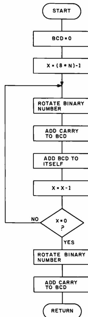
Figure 1: Flowchart of the binary to binary-coded-decimal (BCD) routine given in listing 1.
