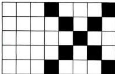
Figure 1: A 5- by 5-dot X-shape can be defined with only 5 bytes of memory.
