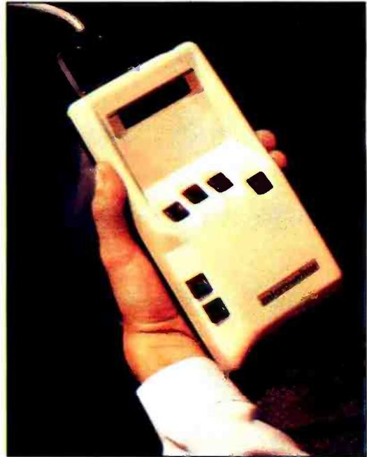
The Microwriter is one of the most interesting devices I saw at the show. A one-handed data-entry unit, it can be hooked up to a printer or a microcomputer, and it even has some limited word-processing features. You enter data by pressing down and releasing certain combinations of the six buttons. At £557.75 (less than \$1000), it's a bit expensive, but its portability and one-handed operation make it desirable to some.
