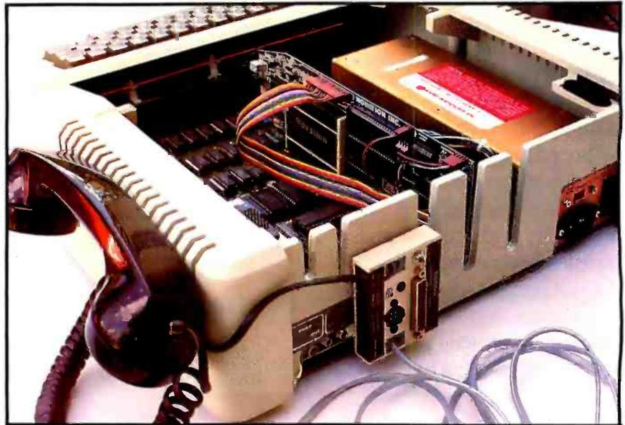
Photo 3: The Apple-Cat II and Expansion Module installed. Using the Expansion Module reduces cable clutter. The author has turned the unit sideways to permit full use of the adjacent slot on the back of the Apple.
