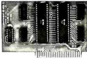
The JBE 6522 Parallel Interface for the Apple II Computer, plugs directly into any slot 1 through 7 in the Apple. This card has 2 6522 VIA's that provide:
