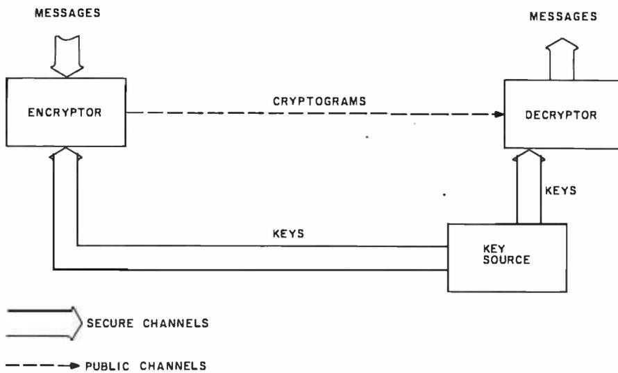
**Figure 1:** A conventional cryptographic system. Encrypted messages (cryptograms) are sent over a public communication channel, while the keys needed for encryption and decryption are sent over secure channels, for example, via courier. The key source may be located at the encryptor or decryptor, in which case one of the secure channels is very short.
