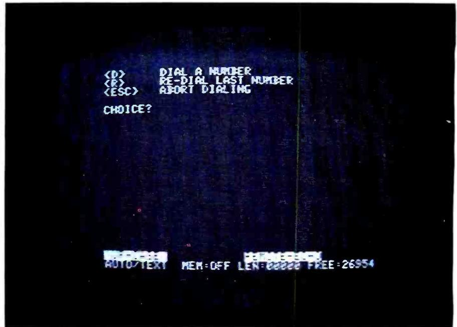
Photo 5: After typing A in the main menu (photo 4), you get this screen, which shows the auto-dial menu. Pressing R now will redial the last number entered. Pressing D will give you the next screen (photo 6).
