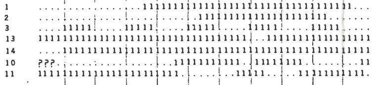
Figure 3: Simulation of the logic of a JK flip-flop. The design uses simple NAND and inverter gates and is presented to the simulator in the same way as in figure 1. The success of this model demonstrates the simulator's accuracy with sequential systems. (Cross-coupled gates used as latches present no problem.)
