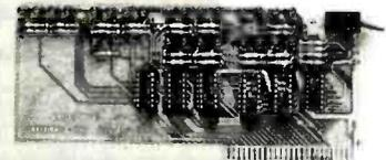
This handy little (3x7") board is ideal for teaching and troubleshooting. It has a run—stop, single step switch which makes identification of shorted lines between address or data-bits easy and shows single steps for teaching computer logic. The display board has 16 Address LEDs, 8 Data LEDs & 1 RDY LED. All lines are buffered.
