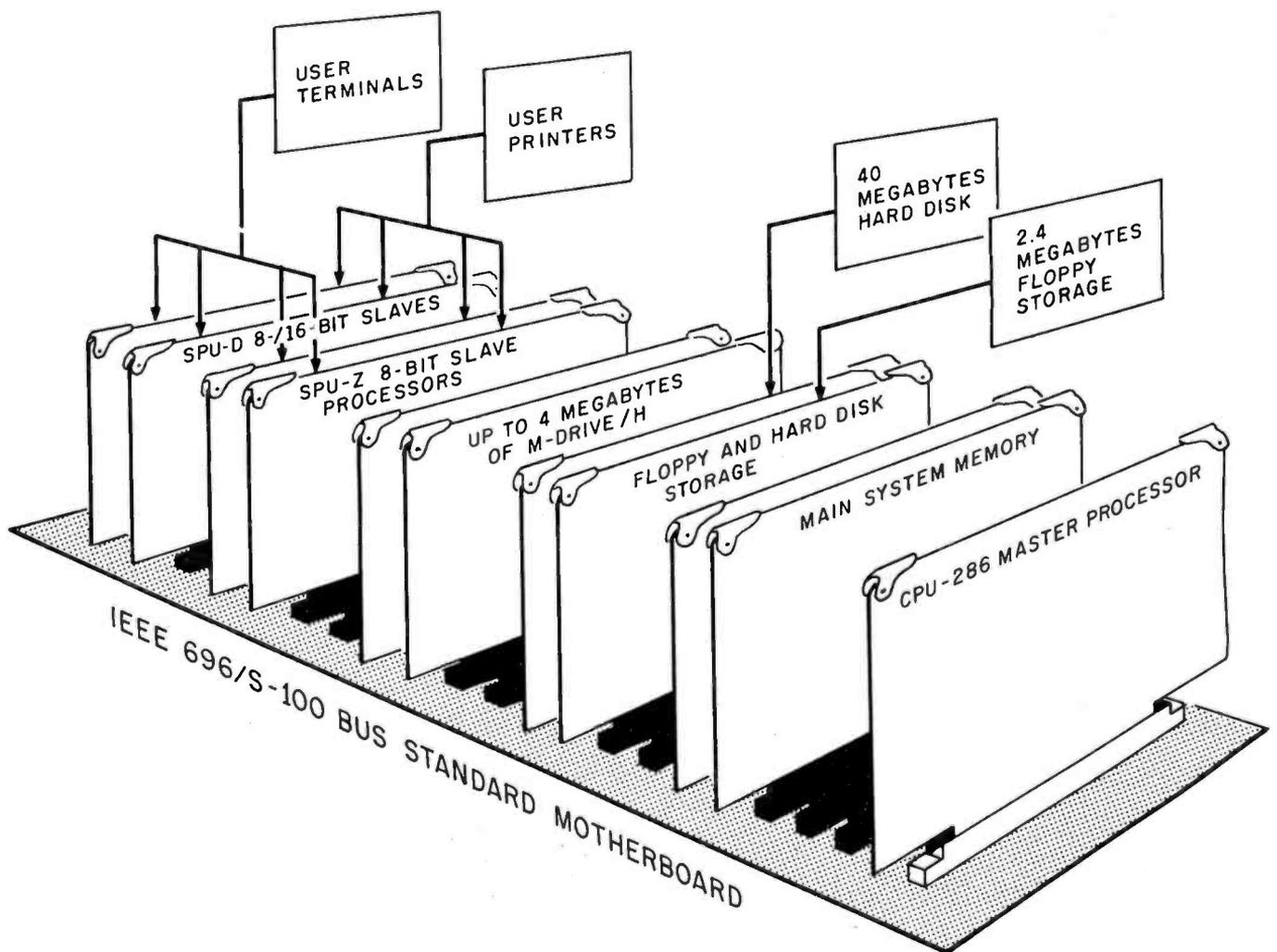
**Figure 1:** A typical system configuration with a CPU 286 master processor (based on Intel's iAPX 286) with its main system memory and floppy- and hard-disk storage. Up to 4 megabytes of M-Drive/H solid-state disk is supported by the system for ultrafast access times. Any mix of up to sixteen 8-bit or 8-/16-bit slave processors may be plugged into the system. (Figure provided courtesy of Compupro Systems.)
