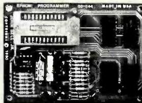
JBE's EPROM Programmer is designed to program 5V 2516's, 2532's & 2716's. It interfaces to the JBE Parallel I/O card using four ribbon cables. An LED indicates when the EPROM is being programmed. A textool zero insertion force socket is used for the EPROM. Comes with complete documentation for writing and reading EPROM's in the Apple II or Apple II Plus. Cables available separately.
