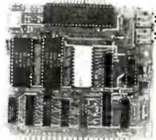
The Z8 Memory, I/O Expansion & Cassette Interface Board (Z8 Expansion Board for short) allows you to add up to 8K of additional memory plus three 8-bit parallel ports to your Z8 Basic Computer/Controller. The memory expansion will support any combination of byte wide RAM memory chips or 2716 or 2732 EPROM. The cassette interface is 300 baud Kansas City Standard (2400Hz/1200Hz).
