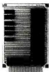
15/30 pin, 3 1/4 x 4 1/2 board w/.1" x .2" hole spacing and power strip run every 1.2". Allows 6x7 8pin IC's or 2x3 24pin IC's
