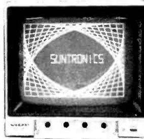
Features: Composite Video Input/Output • Switchable Input Impedance 75 or 10K ohm • 750 Line Resolution at Center and 500 Lines at Corners • Dimensions are 12.13" x 11.34" x 11.65" for the 12" model and 8.66" x 8.54" x 9.05" for the 9" model
