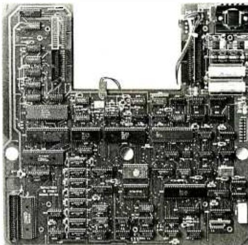
industry standard Z80A-based microcomputer with 64K bytes of RAM. It includes the CP/M\* operating system. Which means you get to choose from literally thousands of ready-to-use application programs.
