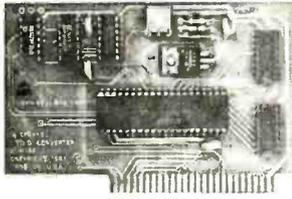
JBEs 16 channel A-D Converter plugs into your Apple II computer. It uses an ADC0817 which incorporates a 16 channel multiplexer and an 8 bit A-D Converter. The 16 inputs are high impedance and the voltage range is 0 to 5.12 volts. Conversion time is <math>< 100\mu\text{sec}</math>. The resolution is 8 bits or 256 steps, linearity is  $\pm 1/2$  step. Two 16 pin DIP sockets are used for input, GND & reference voltage connections. There are 3 single bit TTL inputs. Doc. includes sample program.
