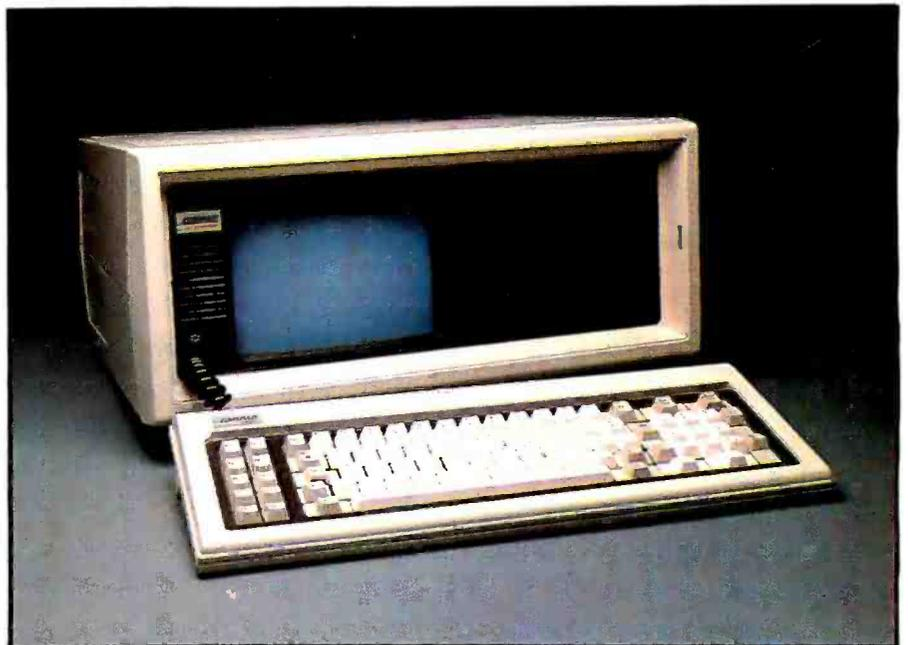
Photo 1: The Compaq, a portable IBM look-alike from Compaq Computer Corp.
