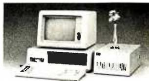
The 192k RAM, 2 asynchronous serial ports, 3 parallel ports, and a Real Time Clock are all built on to the motherboard, so you won't have to waste precious slots on them.
