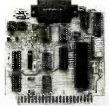
The Serial Expansion Board adds an additional RS-232C serial port to the Z8 system. It runs at 75 to 19,200 baud in all standard protocols. The 20 ma. current loop is opto-isolated for reliability and protection.
