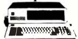
Includes 64K IBM-PC with two 320 KB floppy disk drives, controller color graphics card, monochrome monitor
