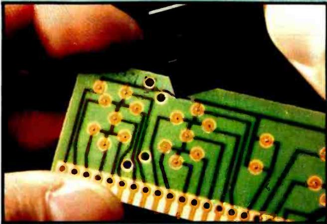
**Photo 3c:** Because this display has one common cathode line for all 4 digits, I had to cut it at strategic points to isolate the digits.
