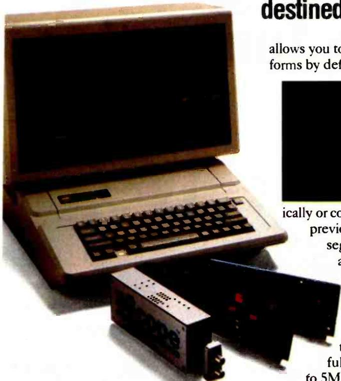
allows you to build complex waveforms by defining them mathematically or constructing them from previously stored waveform segments. aSource generated waveforms have 12-bit resolution and record lengths up to 4096.
