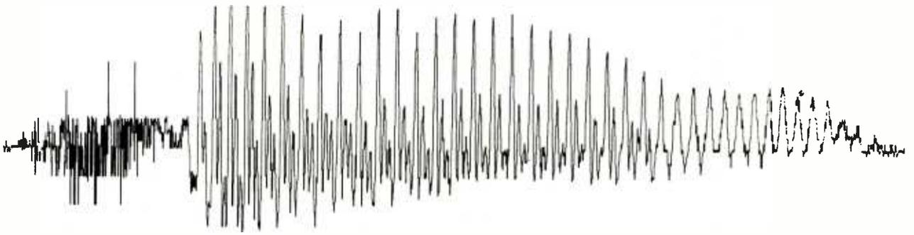
**Figure 3a:** The waveform for my utterance of the word "two" with no filtration. Corresponding to a plot of the function  $V(t)$  over time, where  $V(t)$  is the voltage of the incoming analog audio signal, it graphically depicts the sound-pressure variation at the microphone, over a 400-ms (millisecond) period while the word "two" is being spoken. This graph was produced on an Epson MX-70 dot-matrix printer and then reduced to about one third its original size.
