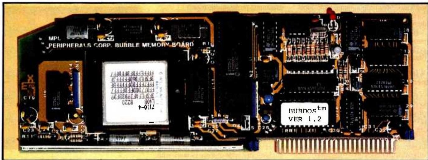
Photo 1: The BUBDISK for the Apple II. The large square chip is Intel's bubble-memory chip, which holds 128K bytes of nonvolatile data.
