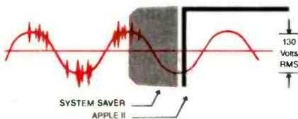
By connecting the Apple II power input through the SYSTEM SAVER, power is controlled in two ways: 1) Dangerous voltage spikes are clipped off at a safe 130 Volts RMS/175 Volts dc level. 2) High frequency noise is smoothed out before reaching the Apple II. A PI type filter attenuates common mode noise signals by a minimum of 30 dB from 600 khz to 20 mhz, with a maximum attenuation of 50 dB.
