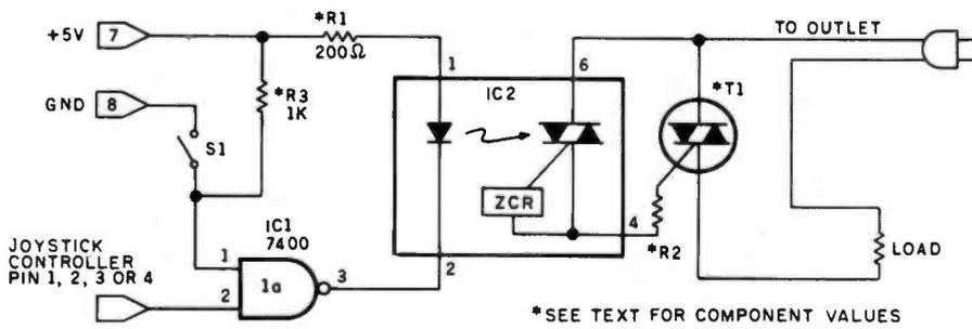
**Figure 4:** This solid-state relay isolates a computer from up to 7500 V, produces no EMI when switching, runs quietly because it has no moving parts, and connects directly to an Atari 400/800.
