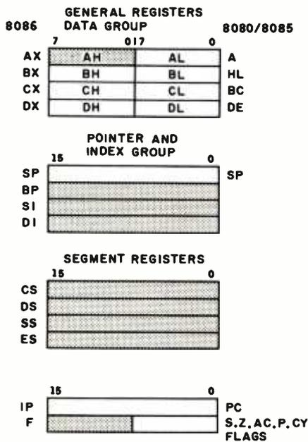
Figure 4: Shown is the 8080/8085 register subset of the 8086. The nonshaded registers are those used by conversion programs when converting programs from the 8080 to the 8086.
