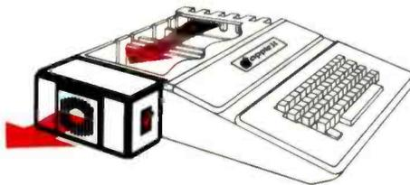
SYSTEM SAVER provides correct cooling. An efficient, quiet fan draws fresh air across the mother board, over the power supply and out the side ventilation slots.
