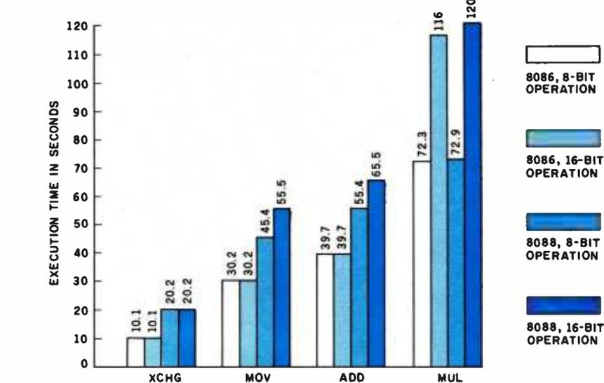
Figure 1: A comparison of representative 8086 instructions by processor (8086 versus 8088) and operand length (8 versus 16 bits).
