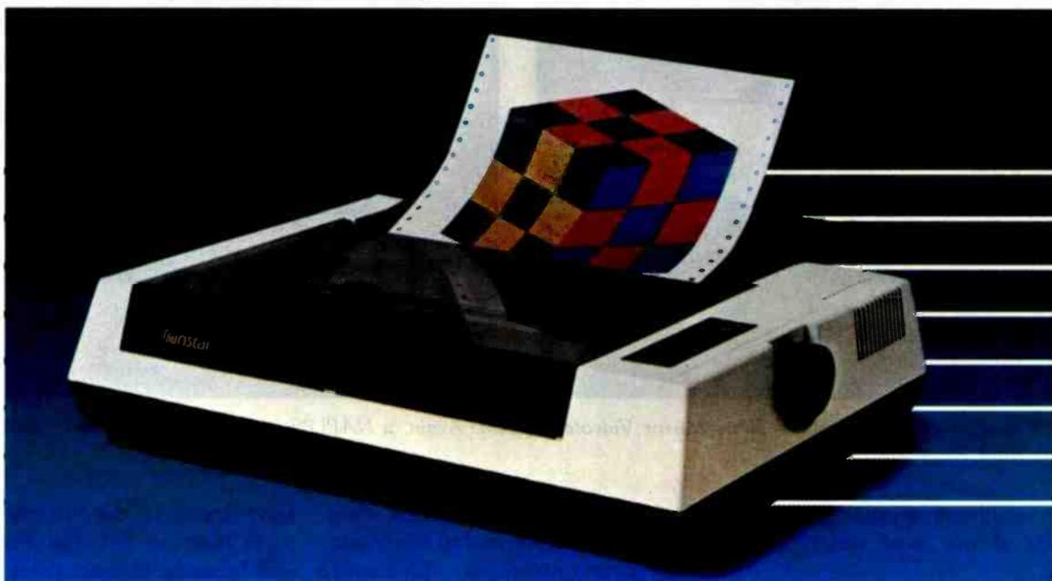
**T**he technology of the all-new Transtar 315 color printer revolutionizes color impact printing! Unlike old-fashioned printers needing multiple passes with pins to print color, the Transtar 315 employs an innovative 4-hammer print head to allow 7 colors and more than 30 shades to be printed in a single pass!
