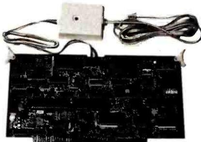
PMMI & Racal Vadic joined forces to bring you the first Bell 212A-compatible modem for the S-100 bus. The MM-212 is a top quality modem designed to meet all physical, electrical & timing requirements of the IEEE 696/S-100 specification. FCC registered for direct connection to the telephone line.
