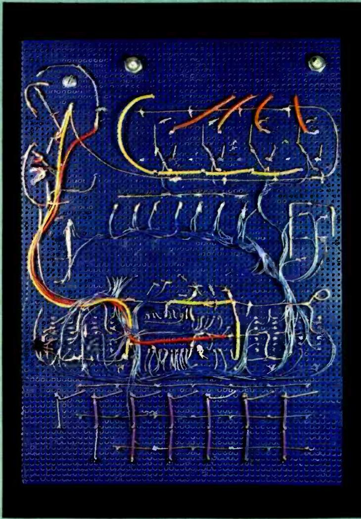
Photo 2: Back side of the RTC-4 prototype.
