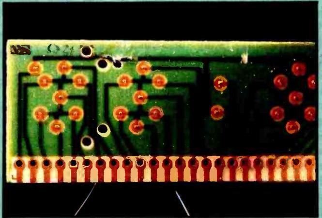
**Photo 3d:** Finally, I drilled holes and soldered wires to the individual digit connections.
