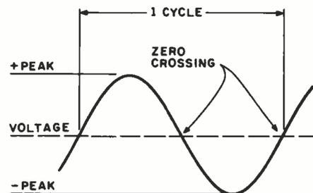
**Figure 3:** Switching power on and off at the zero-crossing points of the AC cycle. The circuit shown in figure 4 uses this technique to prevent production of electromagnetic interference.
