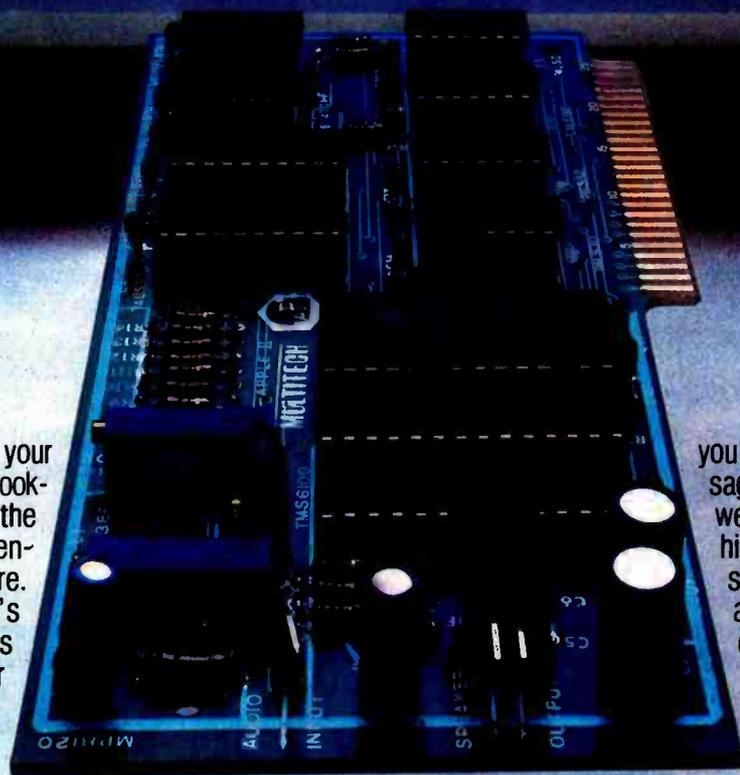
you to create virtually any message you want. And because we use Texas Instruments' high-performance TMS5220 speech chip—coupled with an on-board amplifier and external high-quality speaker—you also get the most natural sounding voice quality around.
