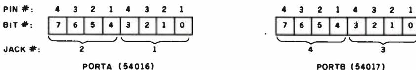
Figure 2c: I/O ports used to access joysticks.
