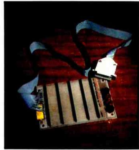
**Photo 5:** The new port-bus assembly, fitted with female 0.1-inch bus connectors and 10-kilohm termination resistors. Insert circuit boards beginning with the connector farthest from the cable end. The separate power supply is not shown.
