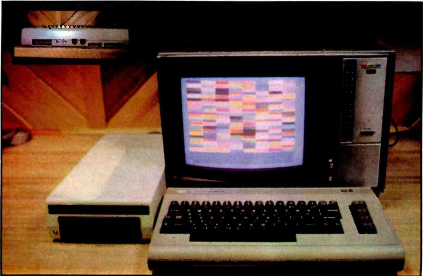
**Photo 1:** The Commodore 64 and 1541 disk drive. Inset shows rear view of the 64. From left to right, the cartridge slot for game or program cartridges; channel selector and TV output connector; the direct audio and video connector; serial port for disk drives or a printer; cassette interface; and the user port for peripherals such as the VICmodem.
