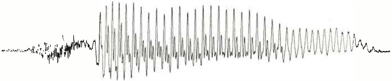
**Figure 3b:** Utterance of the word "two" after the PCM samples have been processed by a low-pass digital filter.
