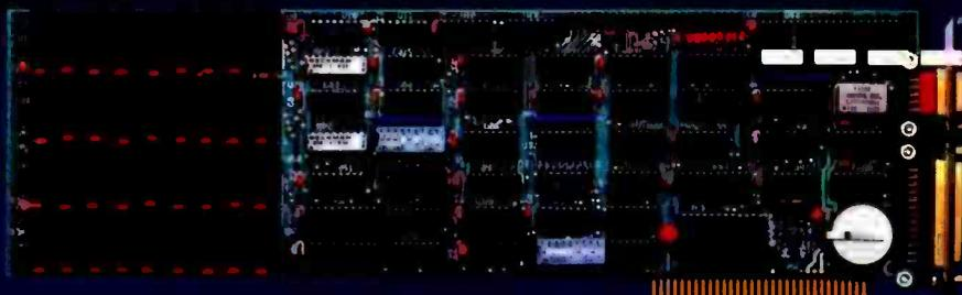
**The IDEBoard:** Multifunction combination board. Memory up to 265KB. Options include serial interface, parallel interface (printer or SASI hard disk) and/or clock/calendar with battery backup. Prices range from \$520 for 64KB with 1 option to \$695 for 256KB with 3 options. All prices include RAMFLOPPY disk emulation software.
