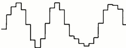
Figure 2c: Speech waveform digitized by differential pulse-code modulation.
