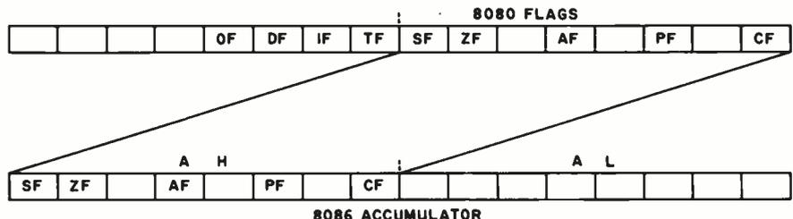
**Figure 3:** LAHF loads the AH register with the low byte of the flags, and SAHF loads the low byte of the flag register with the contents of AH. These instructions are included in the 8086 instruction set to accommodate conversion programs from 8080 to 8086.
