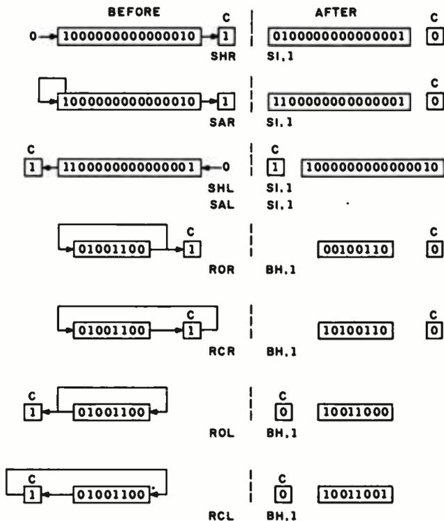
Figure 7: The shift and rotation instructions work on bytes or words. The two forms of shifts and rotations are single-bit, as shown, and a variable-bit form.
