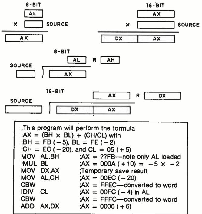
Figure 6: The 8086 multiply and divide instructions use dedicated registers for one of the operands and to hold the results of the operation.
