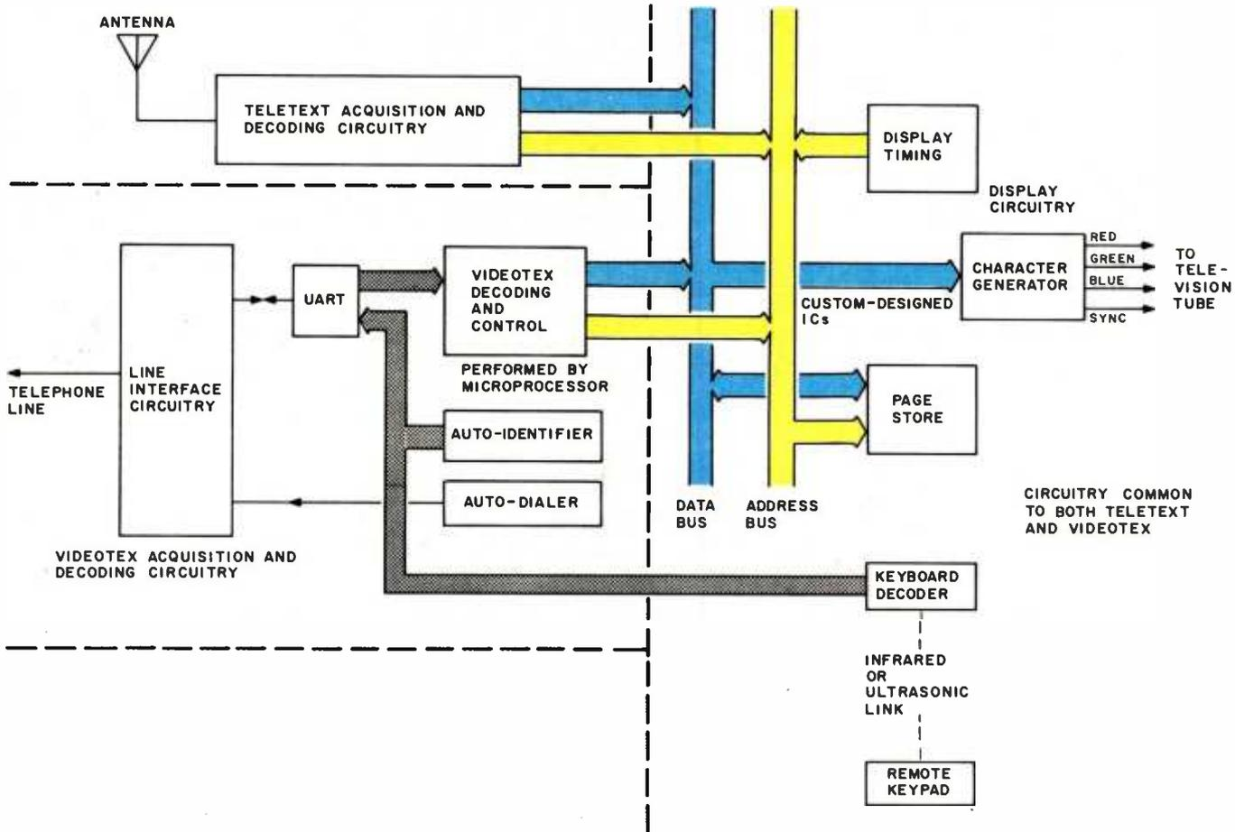
Figure 2: A block diagram of a complete teletext/Prestel terminal.
