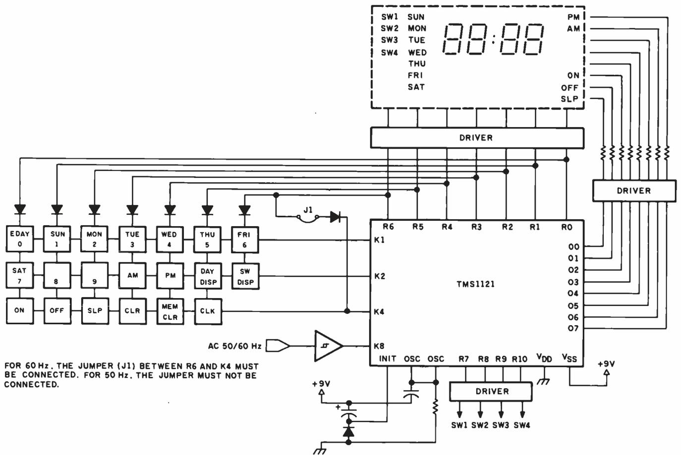
Figure 2: Block diagram of the Circuit Cellar RTC-4 real-time controller, showing the TMS1121C 4-bit microcomputer and its associated user-interface components.
