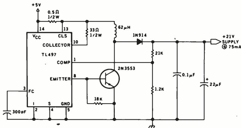
Figure 5: A DC-to-DC switching-regulator power supply provides the +21-V programming voltage suggested by the EEPROM's manufacturer.
