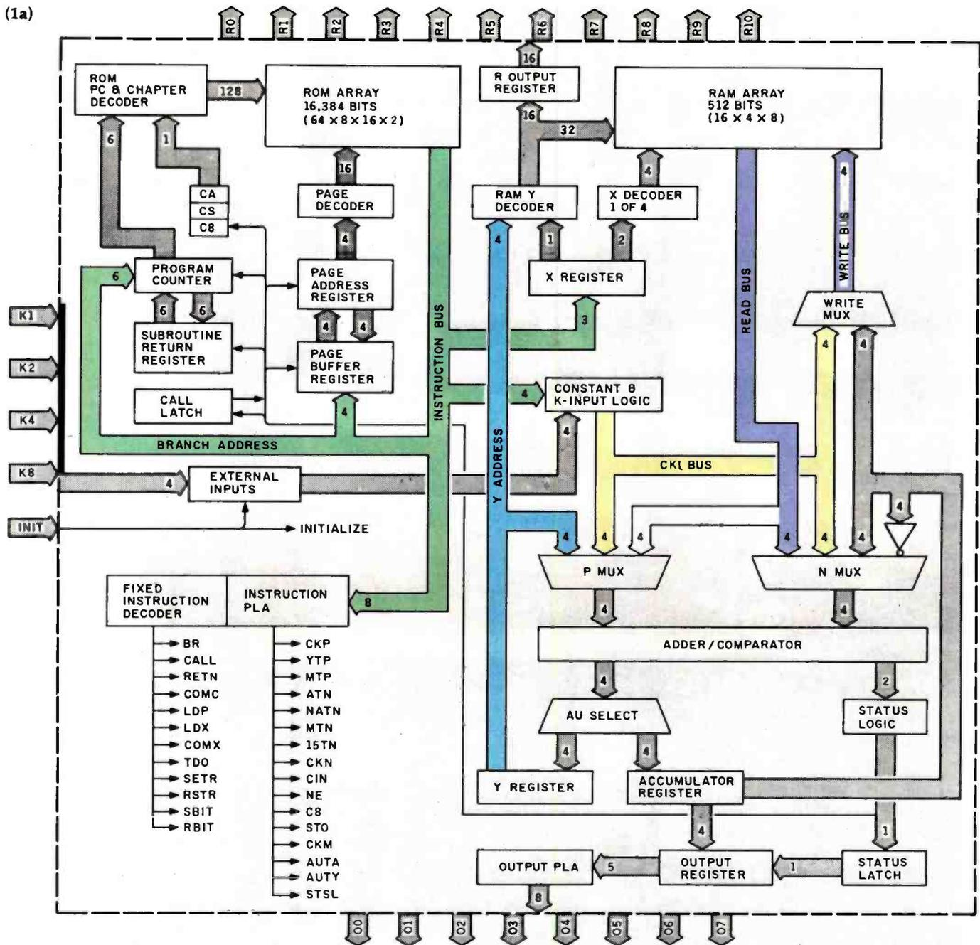
Figure 1: The functional block diagram of the Texas Instruments TMS1100 4-bit single-chip microcomputers is shown in figure 1a. Figure 1b shows the pinout and I/O specifications of the TMS1000 series.
