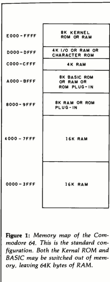
**Figure 1:** Memory map of the Commodore 64. This is the standard configuration. Both the Kernal ROM and BASIC may be switched out of memory, leaving 64K bytes of RAM.
