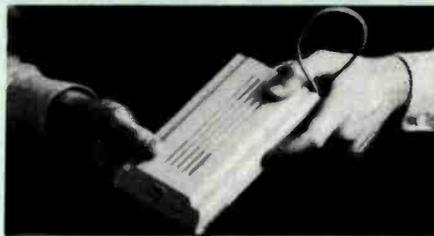
An exceptional value for a 1200 baud modem. The **Password** is a direct connect originate/answer type modem with 0-300 & 1200 baud capability (Bell 212A compatible). Features include auto dial, auto answer, auto mode and auto speed select, full & half duplex (local echo), DTR override, RS-232C pins 2 & 3 reversible & audio phone line monitor. Single button operation makes the **Password** very easy to use. Comes with an RS-232C cable, power supply & modular telephone cable.
