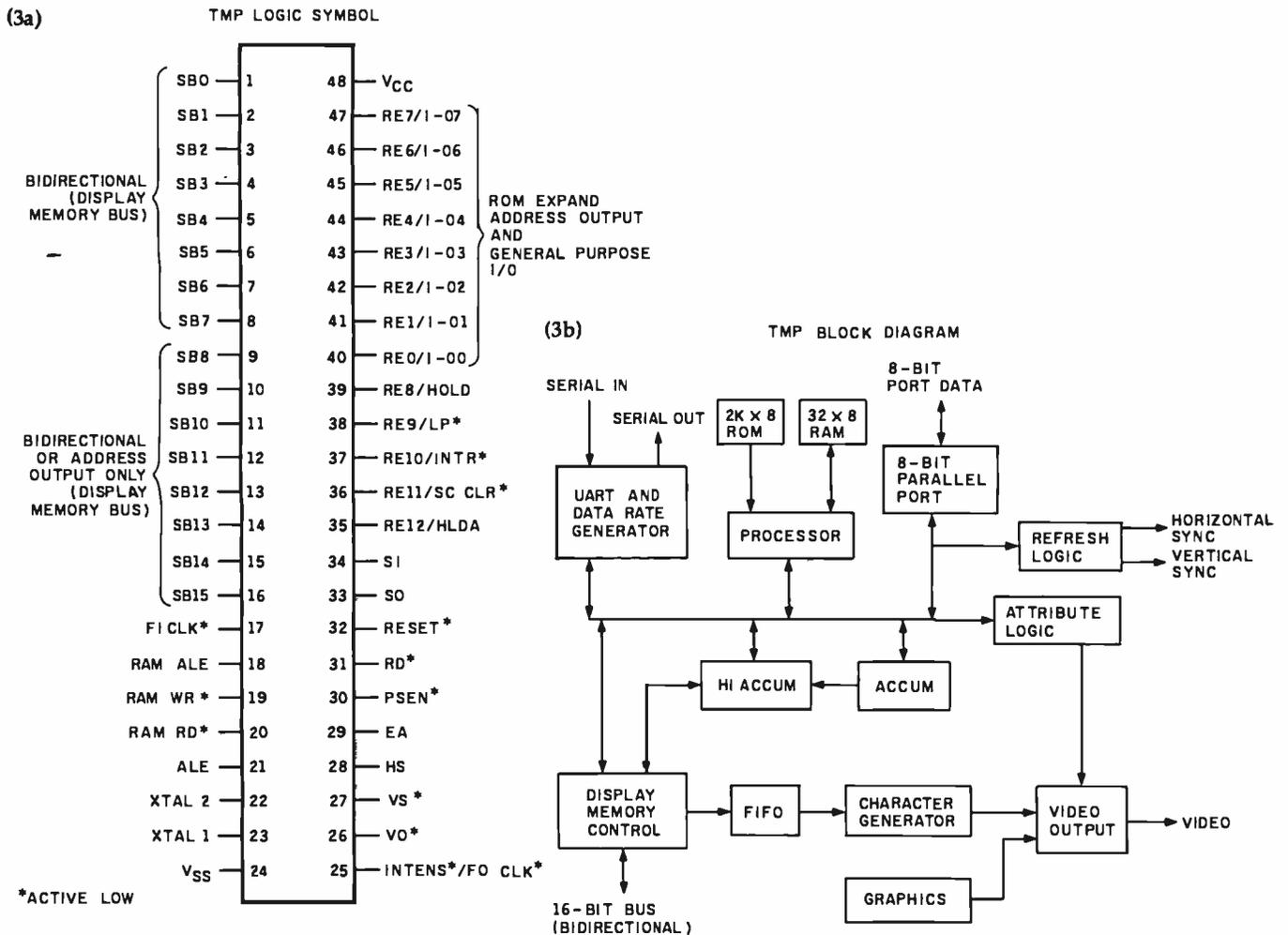
Figure 3: A pinout diagram (3a) and a block diagram (3b) of the National Semiconductor NS455A TMP.
