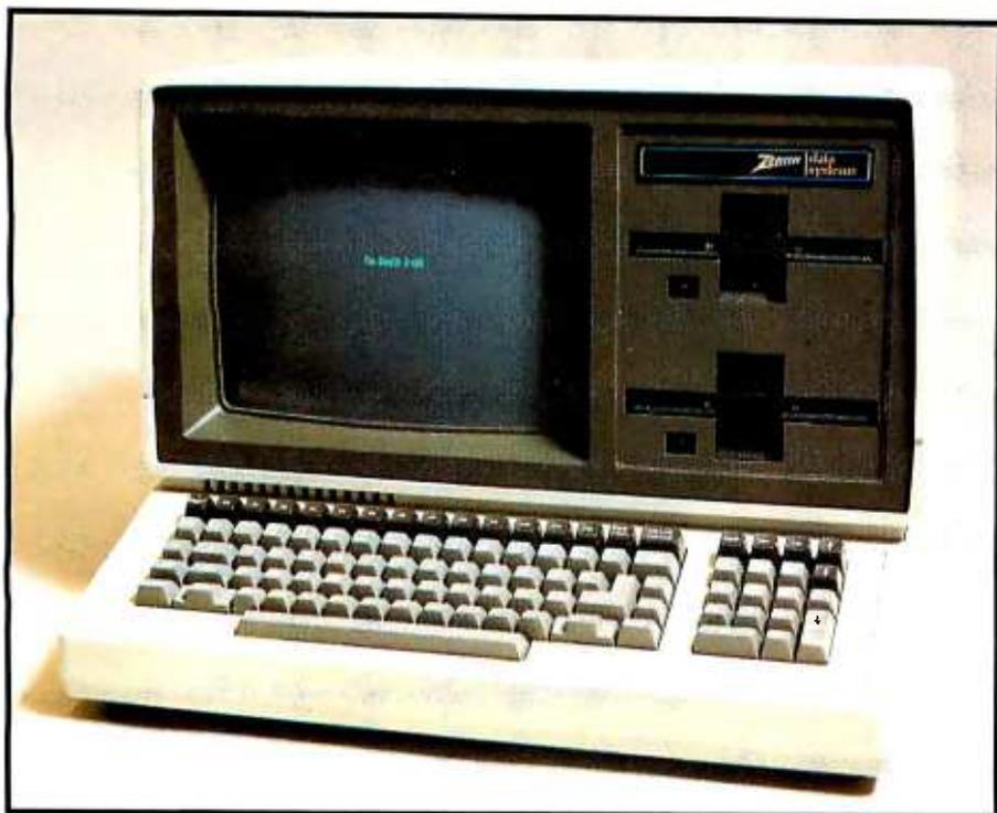
*Photo 1: The Zenith Z-100. This version features a monochrome monitor in All-in-One style. In another configuration, the Low-Profile style, the monitor is in a separate enclosure and the disk drives are arranged horizontally above the keyboard. An RGB color monitor is available for both styles. Note that the keyboard has an IBM Selectric-style key layout, with a numeric keypad on the right and a row of function keys along the top.*
