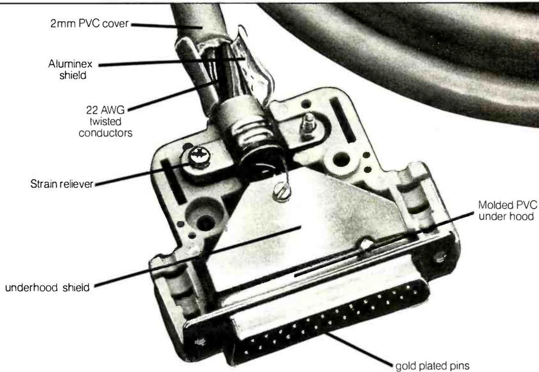
Take a look at the picture above. The shielding under the RS232 connector hood of DATA SPEC™ cables is different from anything you've seen before. No flimsy foil. Or painted hood. Instead, DATA SPEC™ gives you an extra heavy gauge shield under the normal hood which ensures that the cables exceeds the FCC requirements on emission standards.
