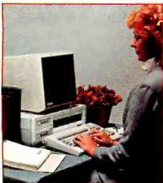
**STANDARD FEATURES:** • Full Graphics capabilities (640 dots x 200 lines) • 128K Ram (expandable to 256K) • Two RS232 Serial Ports • One parallel printer port • Color Display Card • Fully detachable, IBM-compatible Keyboard • 8 Expansion Slots • One 5¼-inch Floppy Drive (327Kb-formatted) • MS-DOS Operating System (MS-DOS 2.0 and CP/M compatible) • 8088 Processor • Spooler (part of system memory, can be used as a printer buffer) • Real Time Clock and Calendar
