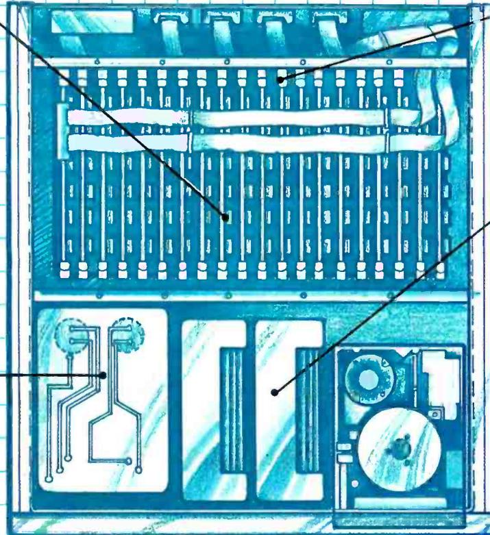
**Up to 32 Users — in Parallel** Our multiprocessor system uses up to 16 Slavenet™ processor boards — each a complete Z80 computer with 64K RAM per user — to maintain fast, multi-user performance as you add users or tasks. Both 12 and 20 slot S-100 models available.
