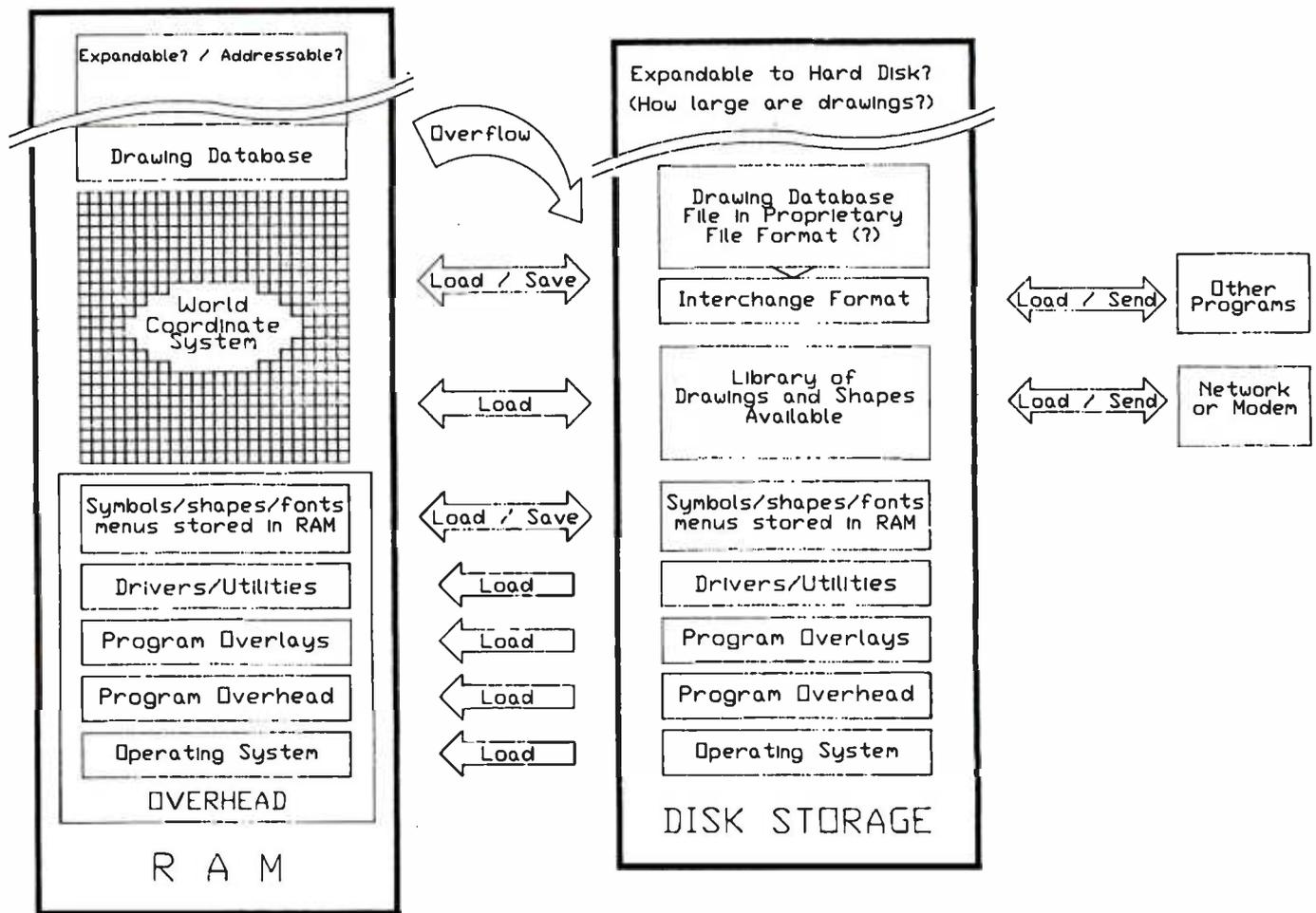
Figure 5: The interplay between RAM and disk storage.
