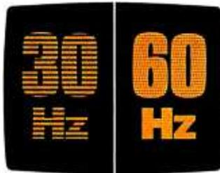
As simulated, Tek's 60 Hz refresh rate and bright phosphors result in a flicker-free image with perceivably better definition than that provided by 30 Hz terminals quoting greater pixel densities.
