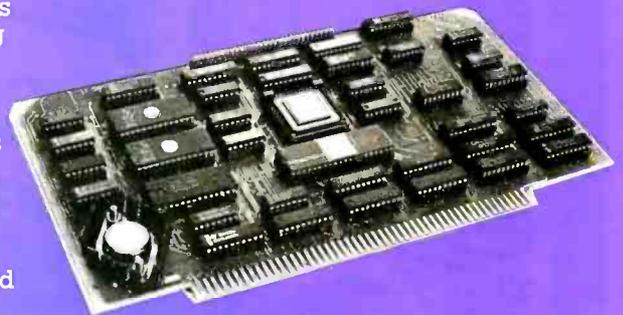
that will allow extension of the memory with a high speed dynamic memory board. The use of the companion memory board will allow use of an 8 Mhz 80286 without memory wait states. The board will contain 1 Mbyte of memory, and will allow cost efficient expansion of 80286 memory space.
