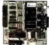
**8051-Based Single-Board Computer with Monitor/Debugger**
