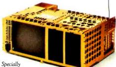
designed shock isolation system protects the fixed disk from jolts.
