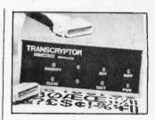
chronously, and it automatically adjusts to data rates ranging from 150 to 9600 bps. It has an errorcorrection feature that causes automatic resynchronization when linenoise errors occur. System hardware includes a Z80 central processor and dual RS-232C ports.
