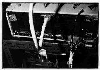
**Photo 2:** A rear view of the CS-9000, showing the IEEE-488 interface with the extender in place (far right), the disk-drive connector (next to the IEEE-488), the Centronics port (middle), and the three RS-232C ports. The connector on the top goes to the video display.
