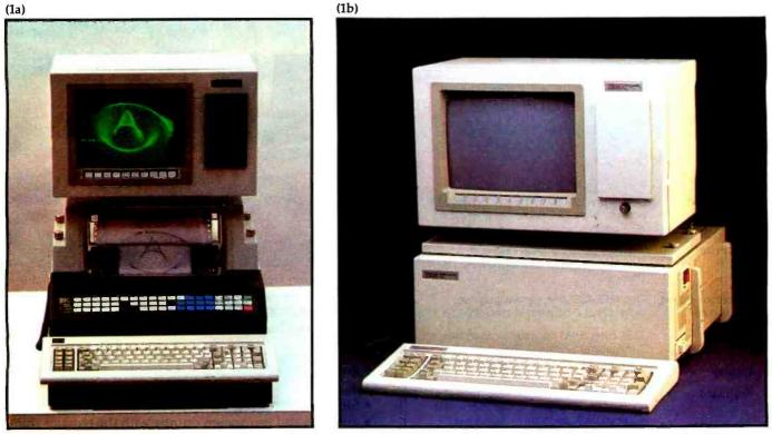
**Photo 1:** At left (1a) is a front view of a typically configured IBM CS-9000 with the built-in dot-matrix printer. The rectangular plate covers a mount for a single 5¼-inch floppy disk. Notice the paper tray under the keyboard. The handle below the video display connects to the mounting yoke (see text). Photo 1b shows a front view of the business configuration of the CS-9000. Note that the built-in printer and softkeys have been removed.
