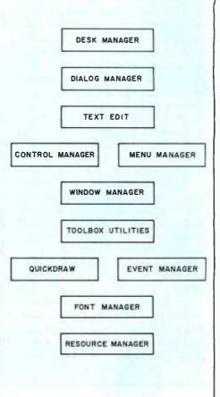
•Dialog Manager: Dialogue boxes are text boxes with several check boxes; usually, clicking the mouse button near a box selects it (and the action or condition associated with it) and unselects the previously checked box. An alert box (as in figure 1h) alerts you to a potentially dangerous situation and forces you to click on one of two buttons, "Cancel" or "OK." The Dialog Manager handles the display of and user response to a dialogue or alert box.
