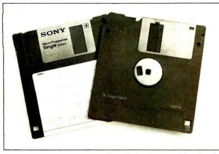
**Photo 4:** The Sony 3½-inch disk is encased in a rigid plastic housing, and the oval window through which the magnetic medium is accessed is protected by a metal shutter that slides out of the way when the disk is inserted in the drive. These factors help protect the disk from casual use.
