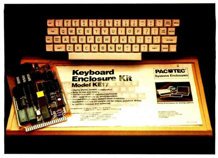
**Photo 2:** The Term-Mite ST can be connected to the stack-pole keyboard shown here, but the NS455A can be used more easily with an Oak full-travel membrane (FTM) keyboard from Oak Switch Systems Inc., POB 517, Crystal Lake, IL 60014. An enclosure from Pac Tec (Enterprise and Executive Aves., Philadelphia, PA 19153) enhances the terminal's appearance.
