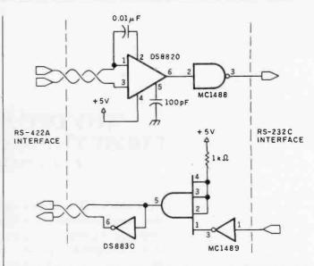
**Figure 1:** A method for interfacing between the RS-422A and RS-232C standards.
