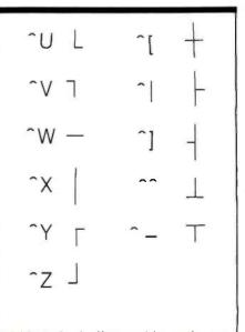
Table 8: In the line-graphics mode, certain control characters produce visible displays of corners, lines, and crosses useful for forming borders on the screen display (<sup>^</sup> is Control-Caret).
