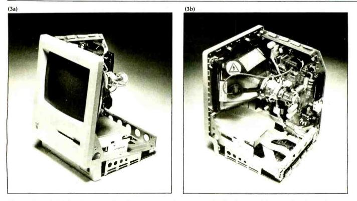
**Photo 3:** Inside the Macintosh computer. From the front (photo 3a), you can see the video display and the 3½-inch disk drive. From the rear (photo 3b), you can see the two main circuit boards (right and bottom), the rear of the video-display tube, the 3½-inch disk drive, and a row of connectors at the bottom of the unit. The connections go, from left to right, to the mouse, a second disk drive, two peripherals (these are two serial ports), and an external amplifier (for sound output).
