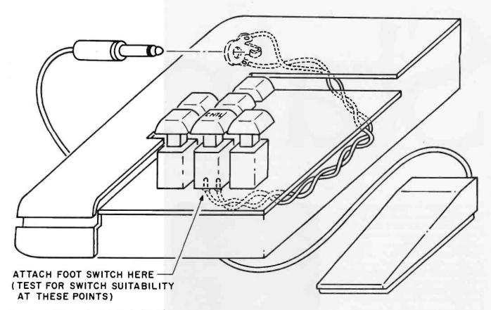
Figure 2: A diagram of a foot switch Control key.
