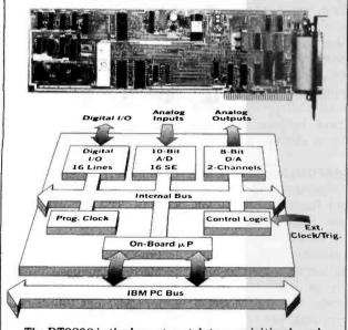
The DT2808 is the lowest cost data acquisition board for the IBM PC. It includes A/D, D/A, digital I/O, clock and DMA on a single board for \$295 in OEM quantity.
