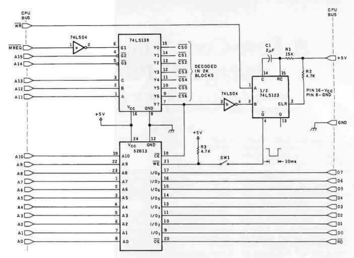
Figure 1: A schematic of the 52B13 EEPROM circuit. The EEPROM is decoded the same as the other 2K by 8-bit memory blocks. A one-shot provides the 10-ms write-enable pulse needed for the EEPROM to be programmed.
