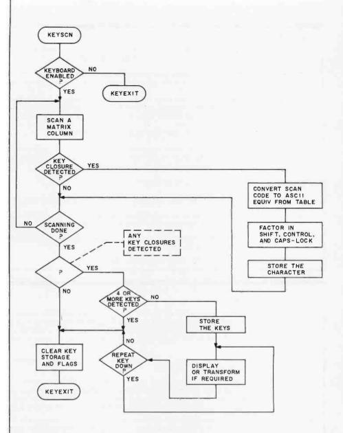
Figure 3: A flowchart of the keyboard-scanning routine.
