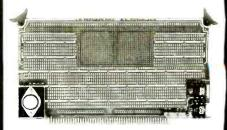
MULTI-PURPOSE PROTOTYPING KIT Industrial Quality with Plated-Thru holes for Wire-Wrap or Solder projects. Complete with  $+5, \pm 12v$  Regulators, Bus Bar, Filter Capacitors, and Manual.
