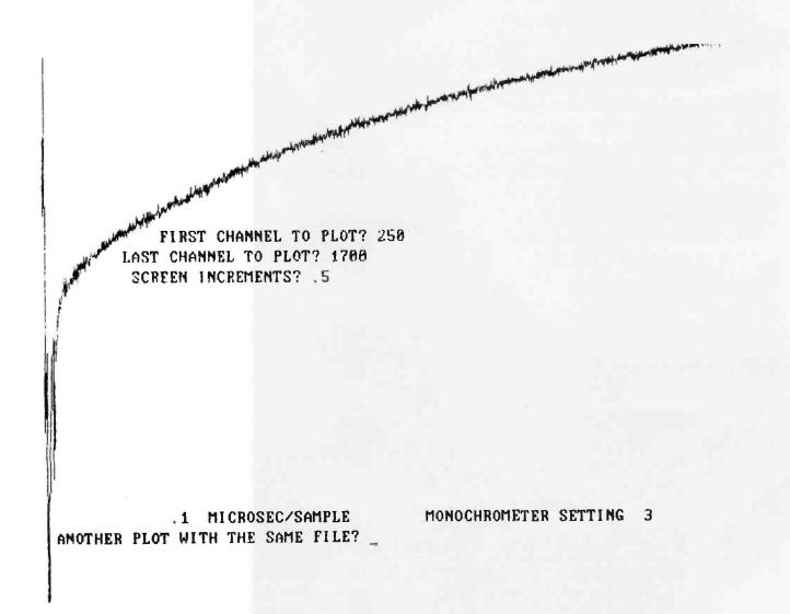
**Figure 1:** A screen dump of a plot of a single scan of the Biomation, showing the luminescence decay curve of Benzil excited by a pulsed nitrogen laser. Data was collected from a modified version of listing 1 and plotted using listing 2.
