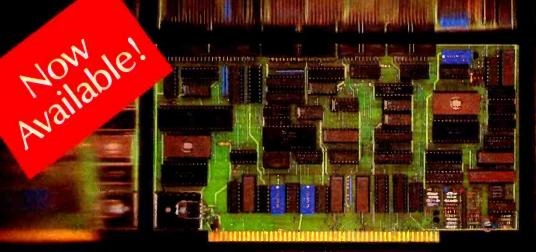
A hard disk and cartridge tape controller together on one board? Magic? Not really. It's Teletek's HD/CTC. The hard disk and cartridge tape drive controller provide the support necessary to interface both rigid-disk drives and a cartridge tape deck to the S-100 bus.
