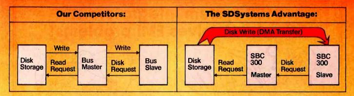
The SBC 300 offers you 64K bytes of dual ported parity RAM. Dual porting allows DMA transfers from disk storage directly to an individual slave processor. This maximizes multi-processor system performance.
